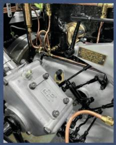
Restoring the steering box meant replicating not only the correct RR-monogramed plate, but also the proper nuts in the proper finish. The fasteners on this car, despite its being constructed in the United States, all conform to period British Imperial standards of the period. Every piece of hardware has to have the correct thread count and pitch as well as the size, shape, and finish accurate to the original.
