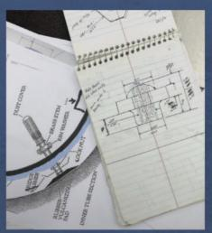
It's a not-uncommon scenario to have access to a part that is almost, but not quite, correct. Sometimes that part can be adapted with some careful thinking. "You cannot get short brass valve stems anymore," Travis says, "so we had to machine off the threads while not getting into the seating of the valve and whatnot in order to use the correct original caps."
