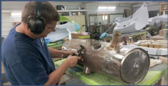
The Silver Ghost's fuel system is rather ingenious, if complicated. Mechanical and electrical fuel pumps were not yet common in this era, but the rear-mounted fuel tank means gravity feed wasn't an option. The Rolls used vacuum and a hand-pump primer with a return line. All of those pieces were decayed, damaged, or missing and had to be rebuilt, repaired, or replicated.
