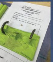
No details are too small to ensure that new-car experience. The cowl vent required both a special, offset bushing to be fabricated for smooth functionality, and also the creation of a new bug screen.
