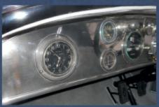
Living as it did in a setting where originality took a back seat to functionality, the Rolls had fallen victim to a previous owner's inclination to "tinker" as Travis puts it. One element of that was the replacement of the original 1921 wood instrument panel with this admittedly handsome, but not correct, chrome-and-stainless piece.
