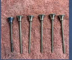
The original knurled-metal pull knobs for the instrument panel were replicated from fresh metal.
