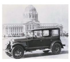
models were built in 1924, and sales were limited to just the three westernmost states, plus a dealer in Baltimore, Maryland. They were nice cars that featured a 60-hp Continental Red Seal six-cylinder engine on a 128-inch wheelbase. The company boasted its handbuilt automobiles contained
