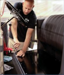
Installing the fresh, brown-leather upholstery was a mildly complicated affair thanks in part to having to compensate for the loaded state of the body bolted to the chassis with the engine in place. What may be flat upholstery in one state, can become oddly wrinkled if the body is twisted when it is bolted down, or even as the engine is installed in the chassis.
