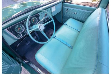
When Matt Field restored the truck, he took particular care to address only the parts that truly needed it. Inside, he retained the original paint and instructional decals on the glovebox door and inner roof panel. The rest of the interior was refreshed.
