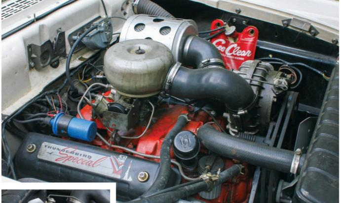
Unlike superchargers for the aftermarket, often the feature of a hot rod engine compartment, the '57 Ford blower was merely industrial in appearance. The McCulloch VR57 made about five pounds of boost.
