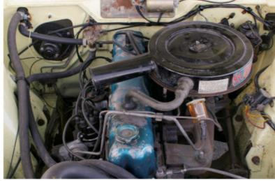
The standard engine during the first year of Gremlin production was this 128-hp, 199-cu.in. straight-six, which contributed to the Gremlin achieving as much as 25 miles per gallon. A 145-hp, 232-cu. in. six was optional and became the standard engine for 1971. This is a preservation effort, and the condition of the finishes is indicative that AMC wasn't striving for 50-year cosmetic durability.
