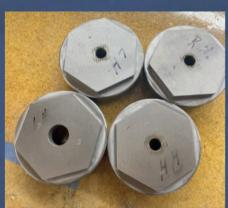
The internally threaded hubcaps were vulnerable to damage from careless use of the wrench. Fresh units were fabricated in the machine shop.
