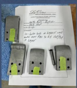
Untold openings and closings had taken their toll on the door hinges, resulting inevitably in sag and poor closing. To take things back to new, the machine shop was commissioned to re-bore the original hinges and machine fresh pins.
