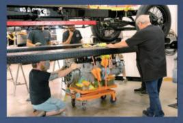
Low-trauma engine reinstallation (i.e., protecting all those carefully restored parts) involves a lift for the engine, a lift for the chassis, patience, and attention to detail.
