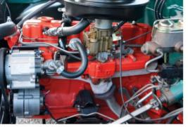
Horsepower wasn't a big concern when John Vikturek bought this K10 pickup in September of 1967. The 250-cu.in. inline six was known to be a reliable choice, especially when paired with a three-speed manual transmission.
