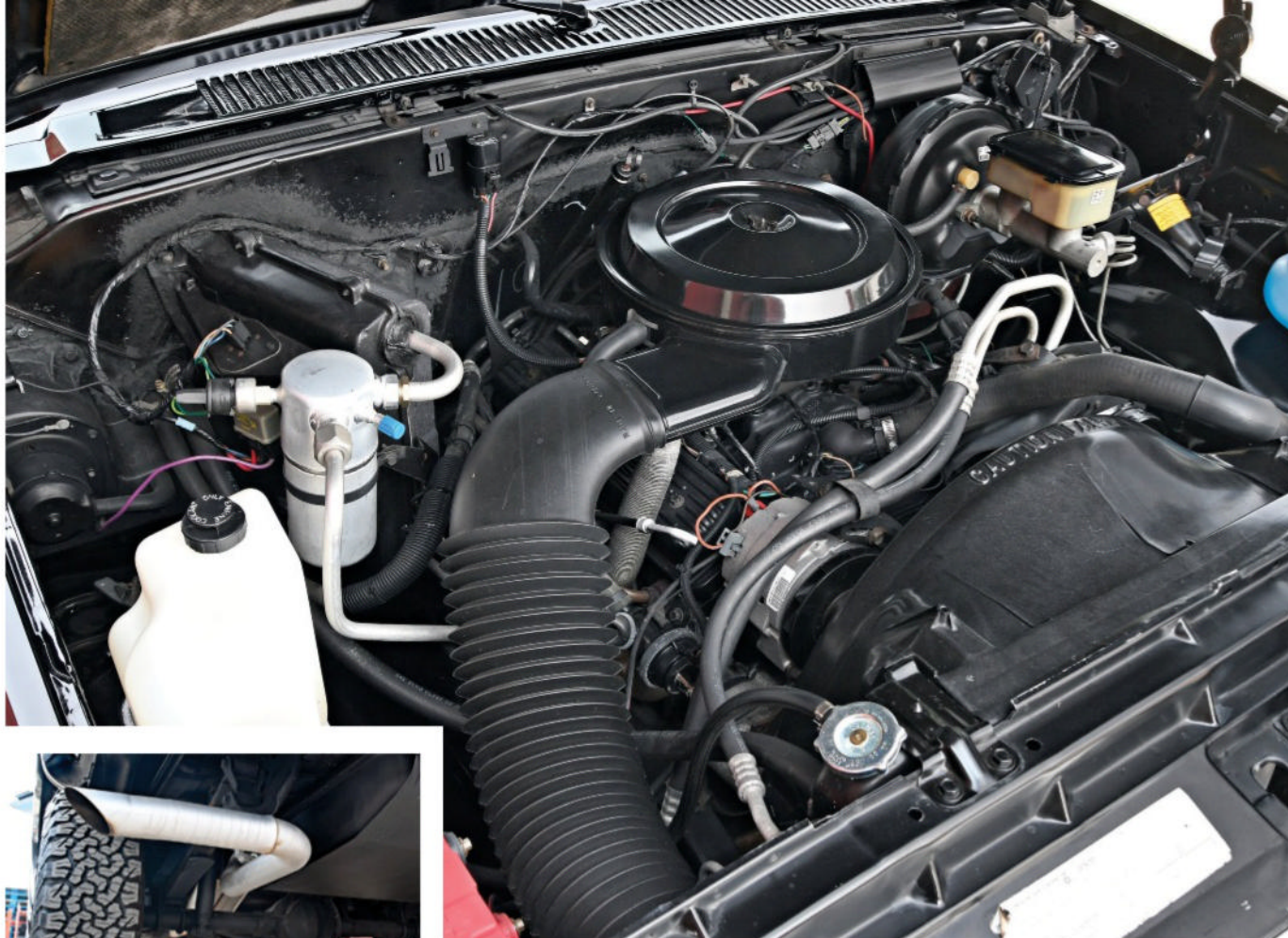
This Blazer was fitted with Chevrolet's EFI 305-cu.in. engine. Its diminutive displacement has managed more than 100,000 miles of travel.
