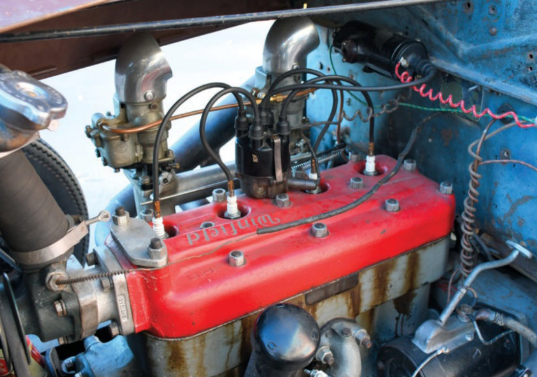
This is the engine Ray raced at Santa Ana, originally built for him by Cook's Machine Shop. Chris says it's been drilled for full-pressure oiling, has had large valves installed, and had an unmarked but "really big" camshaft installed. It has since had fresh pistons and a milder cam installed. The Stromberg 81 carburetors are a smaller version of the 97, originally intended to equip 1937-'40 Ford 60-hp V-8 engines.
