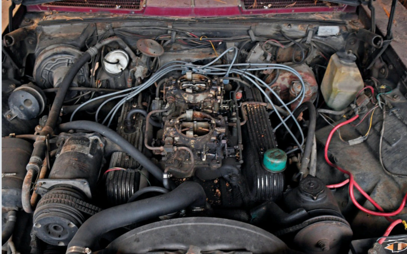
What makes this 1964 Buick Riviera desirable among collectors is the optional dual-quad 425-cu.in. V-8, which boasted 360 hp. It would become the foundation of Gran Sport option a year later.
