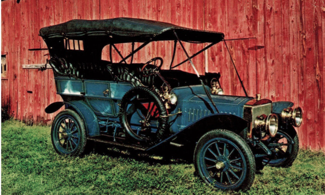
ABOVE: This 1907 Mitchell Model D 24/30-hp five-passenger Touring car rode a 100-inch wheelbase and was priced at $1,800. Note the stylish flared front fenders and large brass headlamps.
