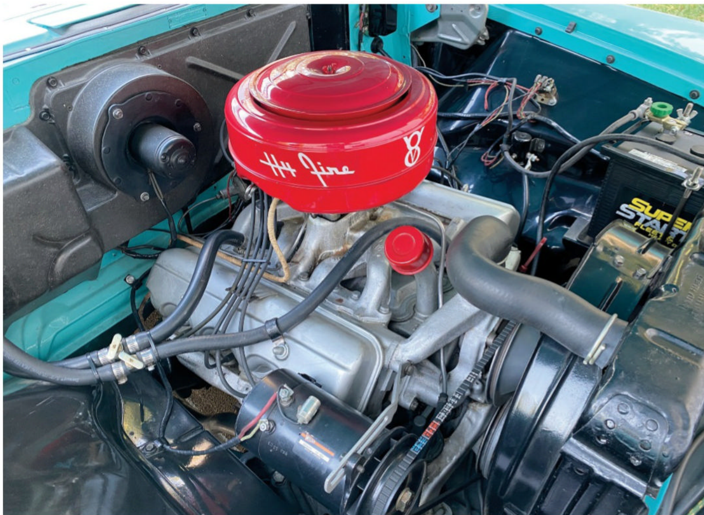
The original buyer of this car opted for the larger-displacement Hy-Fire V-8 but in basic, two-barrel form: a 167-hp, 259-cu.in. unit with 7.6:1 compression. For 1955, Plymouth cars still used a six-volt electrical system, but 12 volts would become standard the next year.
