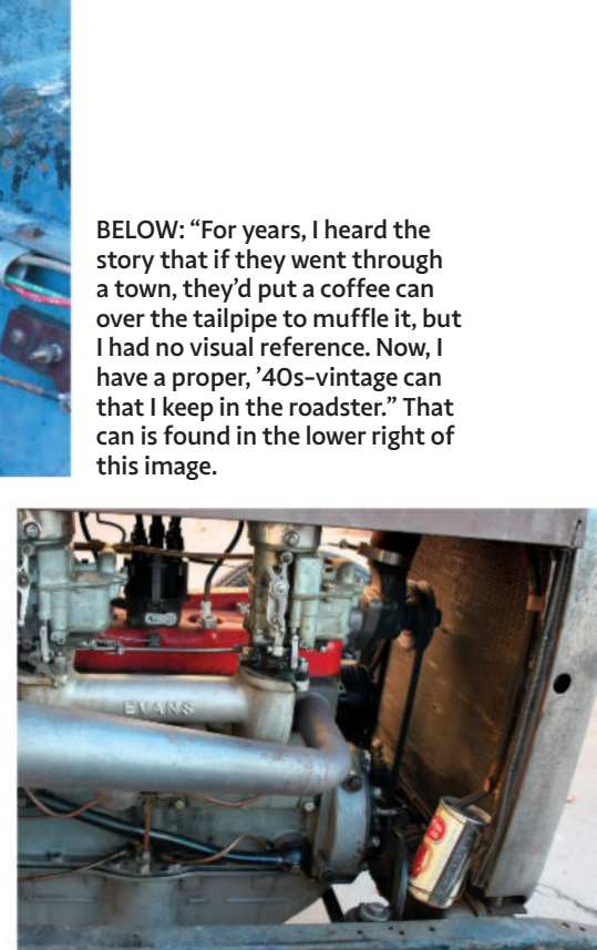
This is the engine Ray raced at Santa Ana, originally built for him by Cook's Machine Shop. Chris says it's been drilled for full-pressure oiling, has had large valves installed, and had an unmarked but "really big" camshaft installed. It has since had fresh pistons and a milder cam installed. The Stromberg 81 carburetors are a smaller version of the 97, originally intended to equip 1937-'40 Ford 60-hp V-8 engines.
