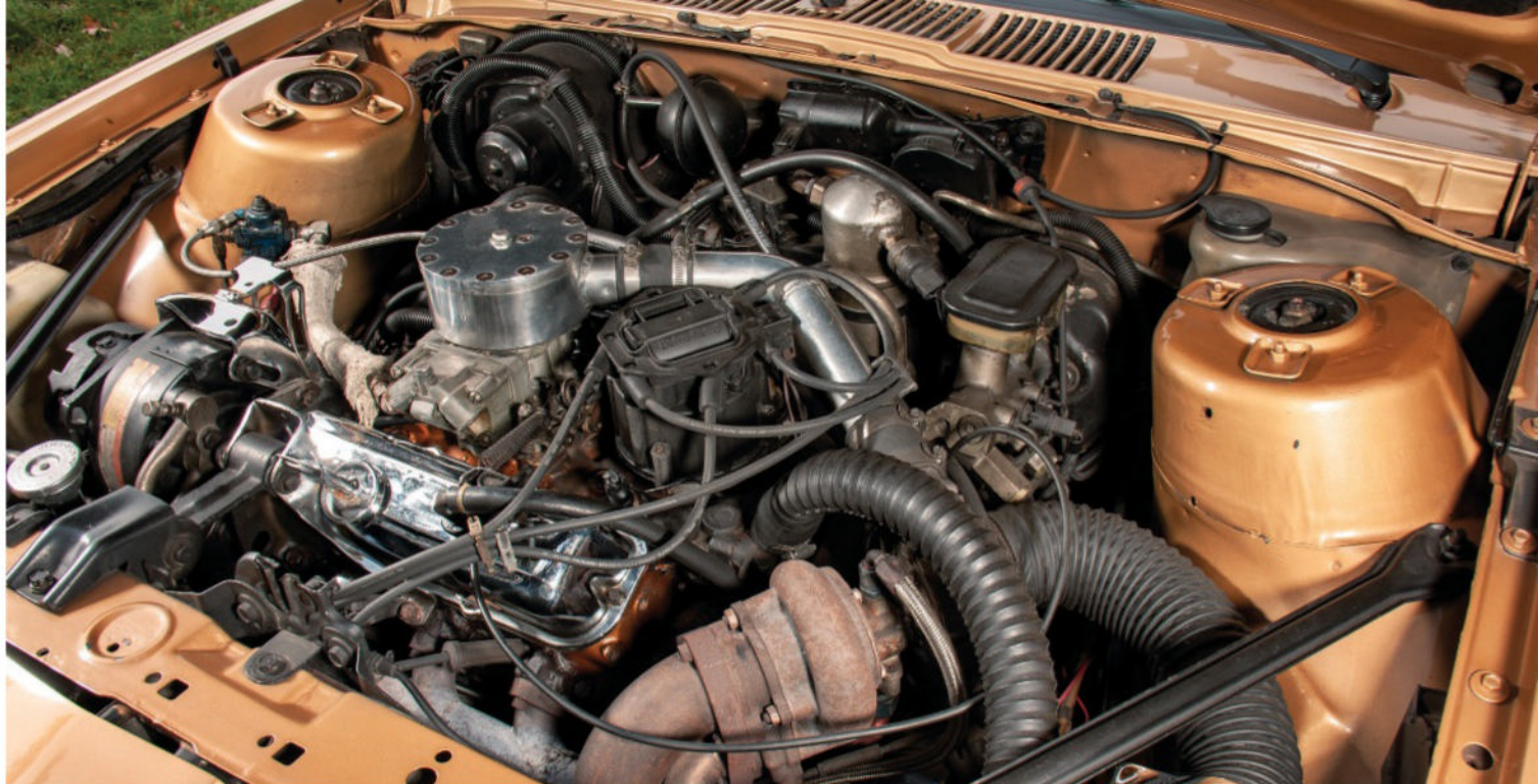
ABOVE: A turbocharger installation and exhaust, valvetrain, and carburetion upgrades (and possibly more) increased the output of the 2.8-liter 60-degree V-6 engine for track duty.
