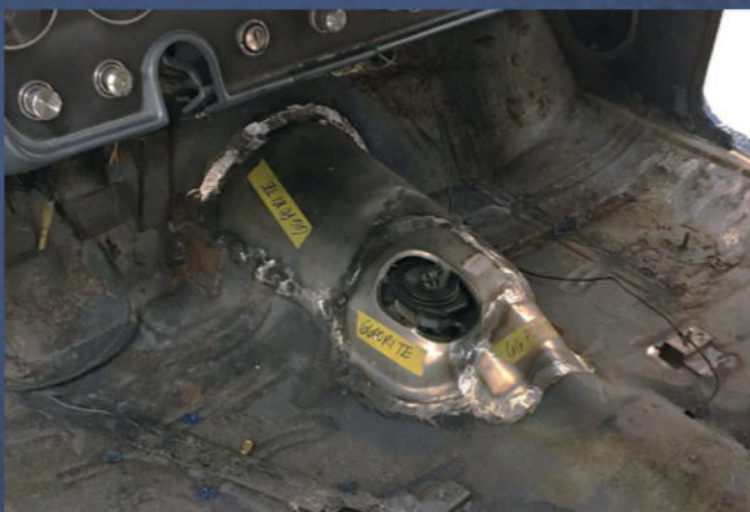
Once the painted body was reunited with the chassis, the transmission tunnel required some modification to fit the new Tremec TKO five-speed conversion.
