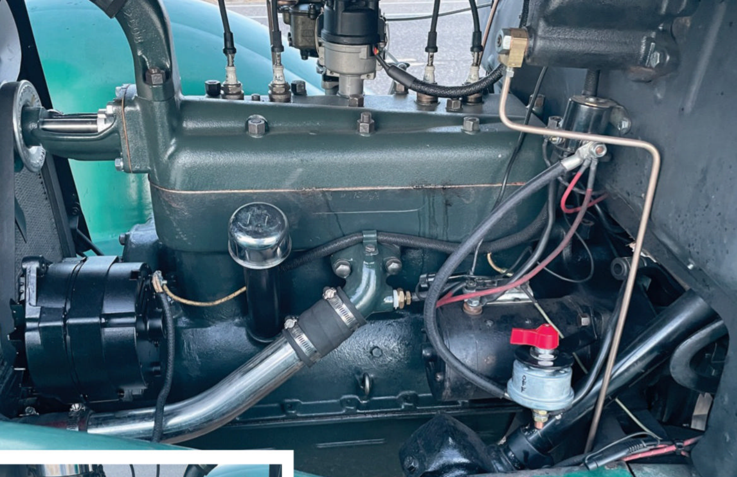
A modified GM 12-volt alternator, electric shutoff, electronic ignition, a downdraft intake, Ford/Holley 94 carburetor, and high-compression 5.5:1-compression cylinder head have all been added for power and reliability.
