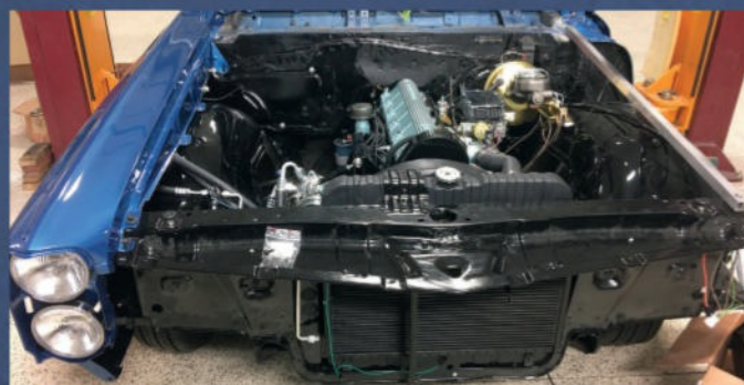
Final stages of the car's reassembly are taking place with radiator, radiator support, and fenders added. Later the stock radiator is sidelined in favor of a modern aluminum unit with dual electric fans for improved cooling.
