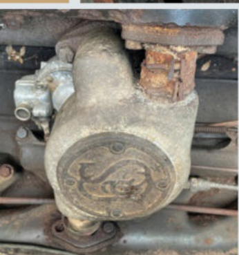
The new-for-1929 La Salle 328-cu.in. V-8 was a capable 85-hp engine that featured unmistakable identifying script. Though it doesn't look like it here, this unit was mechanically revived.
