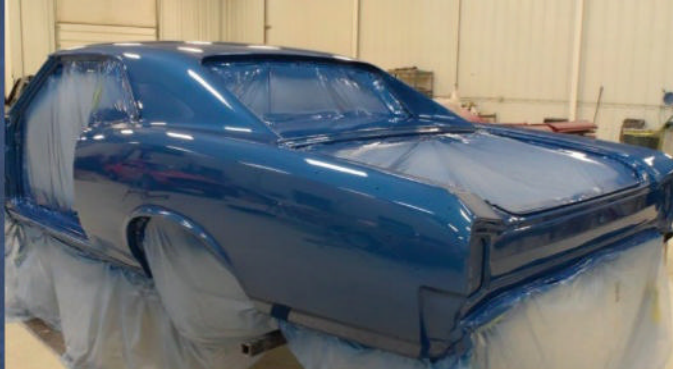
Three coats of PPG urethane matched to the factory Barrier Blue Metallic were applied, followed by four coats of urethane clear.
