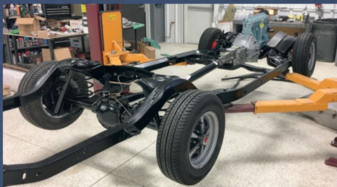
The rebuilt OHC-6 engine, new Tremec five-speed manual transmission, and rebuilt differential have been reunited with the chassis, as have the front and rear suspensions.
