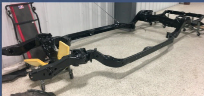
The original frame was stripped of all its components, taken to bare metal, and refinished in chassis black paint.
