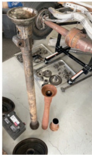
Above Left: A look at the internals suggested that they were clean, and possibly .030 over. Above Right: The torque tube was trimmed to accommodate the Borg-Warner T-5. Right: Making sure those '40 Ford steelies were straight.
