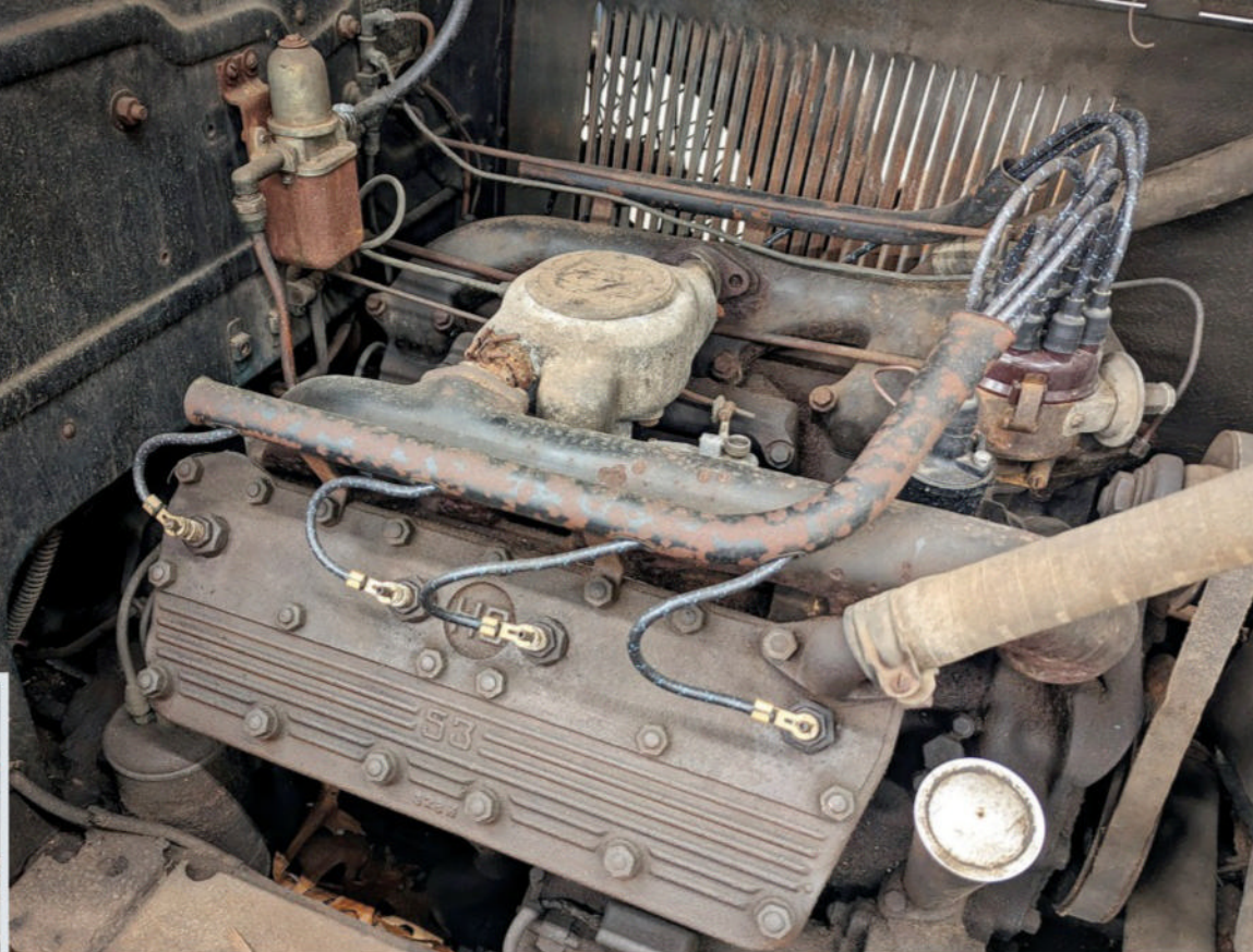
The new-for-1929 La Salle 328-cu.in. V-8 was a capable 85-hp engine that featured unmistakable identifying script. Though it doesn't look like it here, this unit was mechanically revived.
