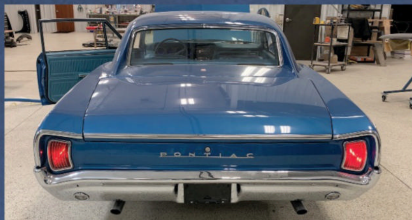
The finishing touches included freshly replated bumpers, polished trim throughout, and restored taillamps that employ LED bulbs from Dakota Digital.
