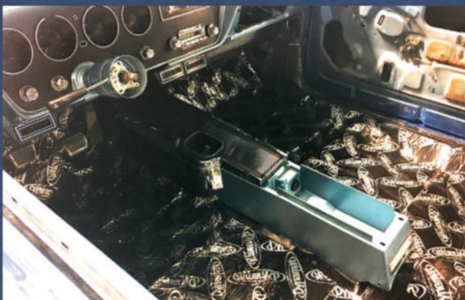
A Dynamat insulation kit was installed prior to fitting new carpeting and reupholstered bucket seats.
