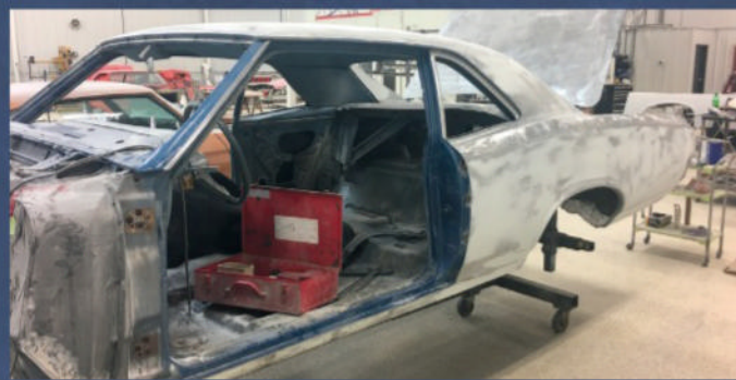
Much of the bodywork has been completed. Happily, no replacement panels were needed. Once this stage is done, the body will receive epoxy primer sealer.
