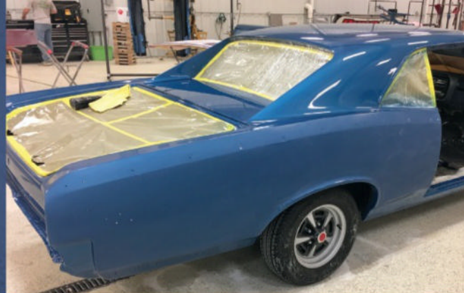
After sufficient cure time, the clearcoat was wet sanded using progressive grits of 800 to 3000 and then machine compounded for a brilliant show quality finish.
