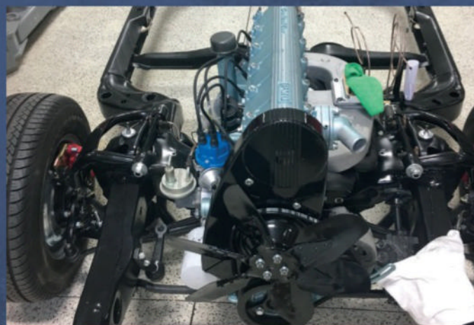
More ancillary engine components are added prior to mounting the body back on the frame. Despite all the upgrades, Rick chose to use the original non-powered steering system.
