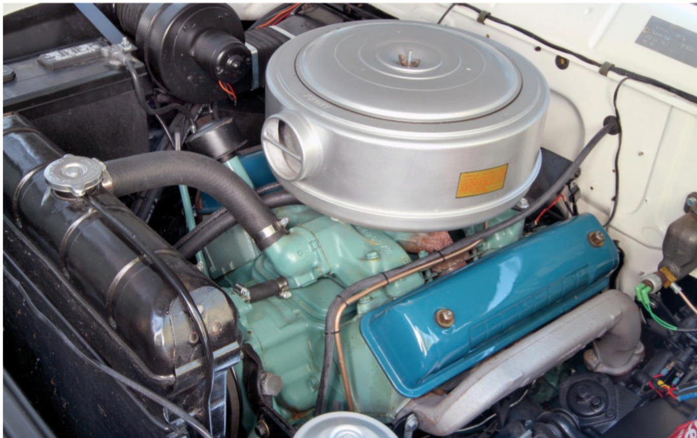
Powering this Meteor is a date-correct, Ford 312-cu.in. Y-block V-8 engine. It was rebuilt to OE specifications during the car's restoration.
