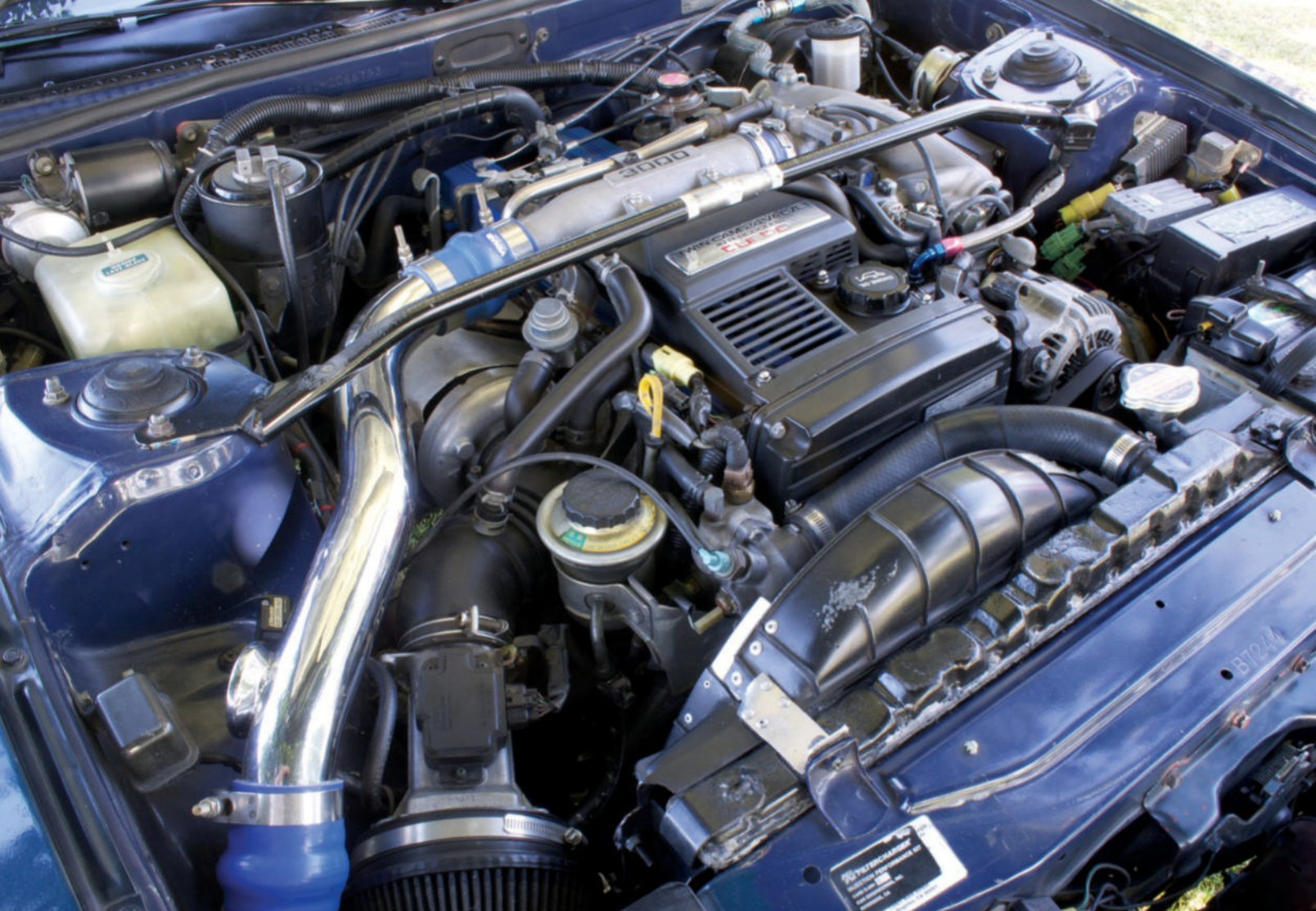
A smorgasbord of factory-stock Toyota bits adorn the 7M-GTE six-cylinder short-block under the hood, including a 24-valve cylinder head and a turbocharger, to help create 230 hp.
