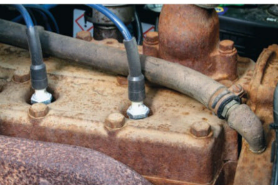
This warhorse flathead engine is Pontiac's venerable 239-cu.in. six-cylinder that boasted 93 hp.
