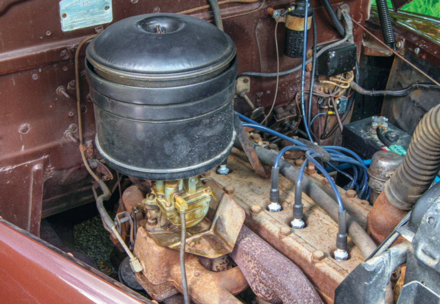
This warhorse flathead engine is Pontiac's venerable 239-cu.in. six-cylinder that boasted 93 hp.
