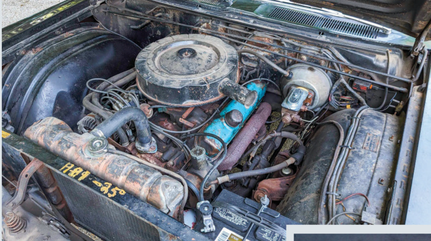
Engine is a 383-cu.in V-8. (BELOW) The black hardtop's fetching gold interior, dash-mount compass, and floor mats all added to its '60s charm.
