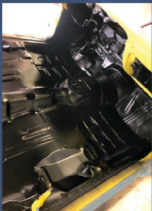
Rotted quarter panel sections were cut from the body shell prior to media blasting. New quarters were then fabricated and welded into position, after which the entire body shell received several coats of primer and paint.
