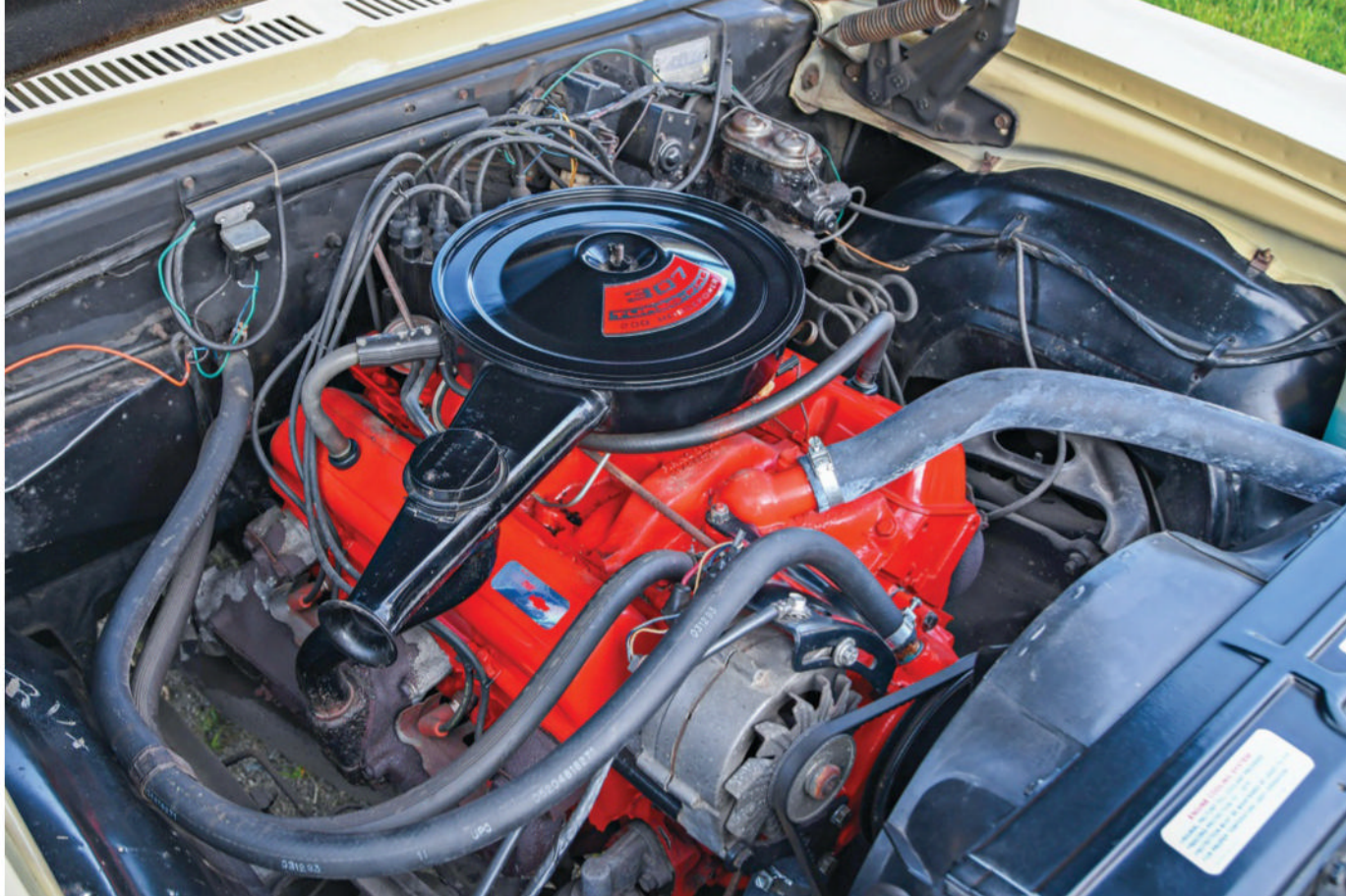
Chevrolet's entry-level V-8 in 1970 was the oft-overlooked 307, with the bore size of the 283 and the stroke length of the 327.
