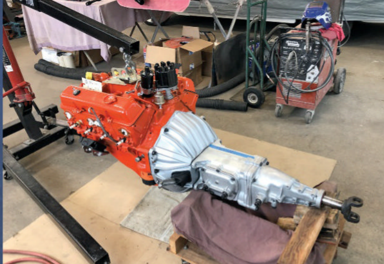
The Malibu's numbers-matching 350-cu.in. engine and four-speed manual transmission were rebuilt by noted first-generation Camaro specialist Jerry MacNeish. The only deviation from stock was the installation of a camshaft from a 350-hp 327 cu.in. V-8.
