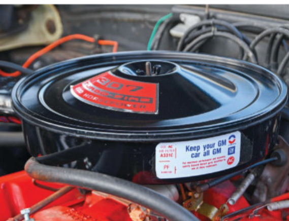
Chevrolet's entry-level V-8 in 1970 was the oft-overlooked 307, with the bore size of the 283 and the stroke length of the 327.
