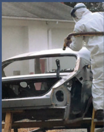
Rotted quarter panel sections were cut from the body shell prior to media blasting. New quarters were then fabricated and welded into position, after which the entire body shell received several coats of primer and paint.
