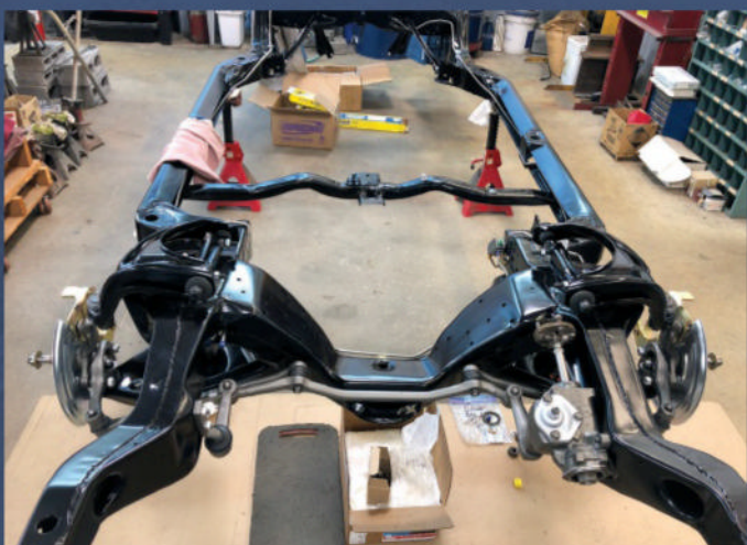
Following proper paint cure time, chassis reassembly began, which included the installation of the rebuilt original steering box, several suspension components, and the original two-piece rotors.
