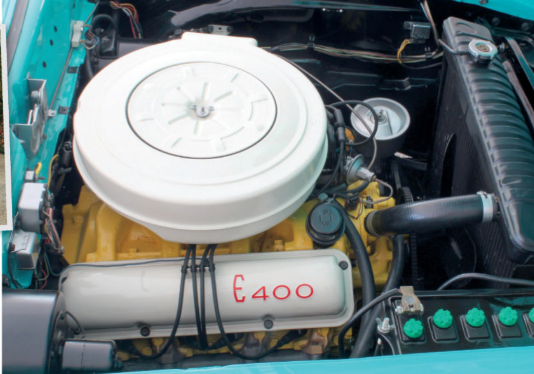
The 303-hp E-400 was Edsel's 361-cu.in. V-8, named for its 400 lb-ft torque rating. The yellow paint is correct for this engine. All Edsels featured a front-hinged hood.
