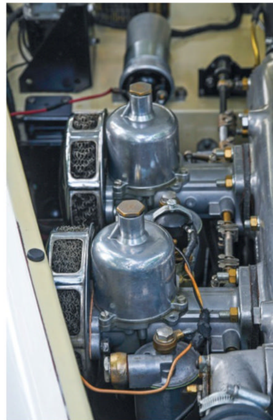
A 3.4-liter twin-cam six-cylinder helped make the Jaguar XK120 an icon of British-built motoring, but in SE guise, such as our featured example, a higher-lift camshaft helped nudge another 20 horsepower out of the engine, making the improved model a fine steed for the American market.
