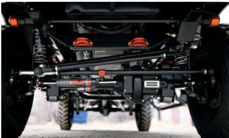
A close look at the undercarriage reveals that instead of leaf-sprung period 4x4 tech, this Apache is underpinned by a state-of-the-art Roadster Shop RS4 chassis.
