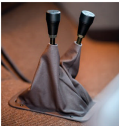
Twin shifters control an Atlas transfer case, permitting selection of two- or four-wheel-drive and high and low ranges.
