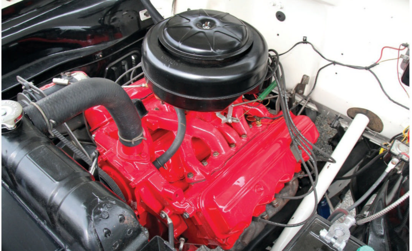
The Dodge Sweptside featured standard half-ton equipment behind the limited-production bodywork, including the installation of a 204-hp, 315-cu.in. V-8 engine, the largest available V-8 in any domestic half-ton.
