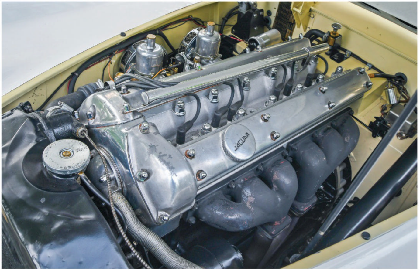
A 3.4-liter twin-cam six-cylinder helped make the Jaguar XK120 an icon of British-built motoring, but in SE guise, such as our featured example, a higher-lift camshaft helped nudge another 20 horsepower out of the engine, making the improved model a fine steed for the American market.
