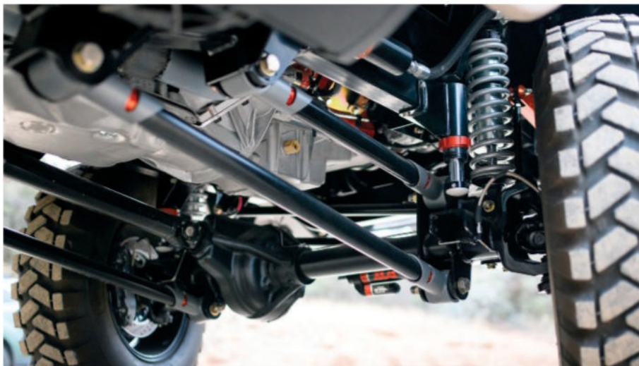
A close look at the undercarriage reveals that instead of leaf-sprung period 4x4 tech, this Apache is underpinned by a state-of-the-art Roadster Shop RS4 chassis.
