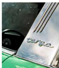
Vertical cabin air outlets on the roll-over hoop improved ventilation in the Targa
