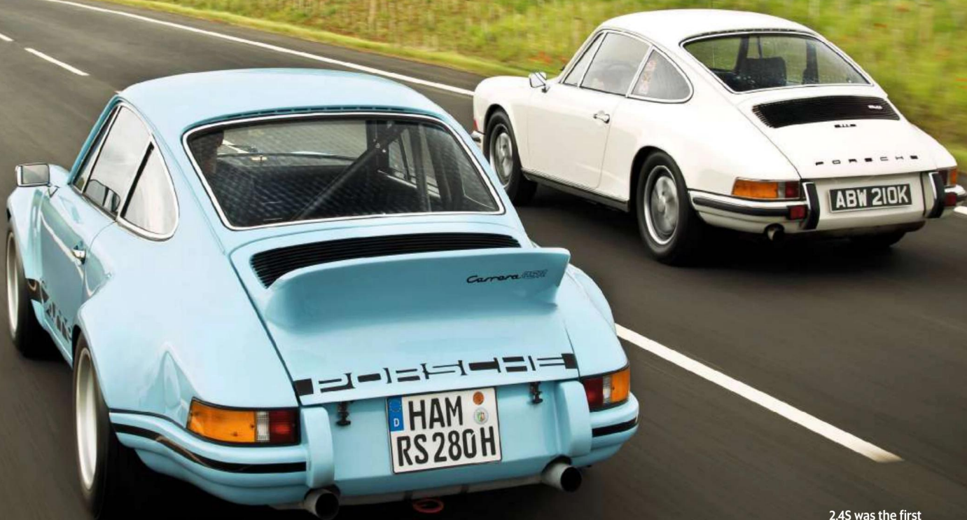
2.4S was the first road 911 to wear a front spoiler; 2.8 RSR used the ducktail from the 2.7 RS
