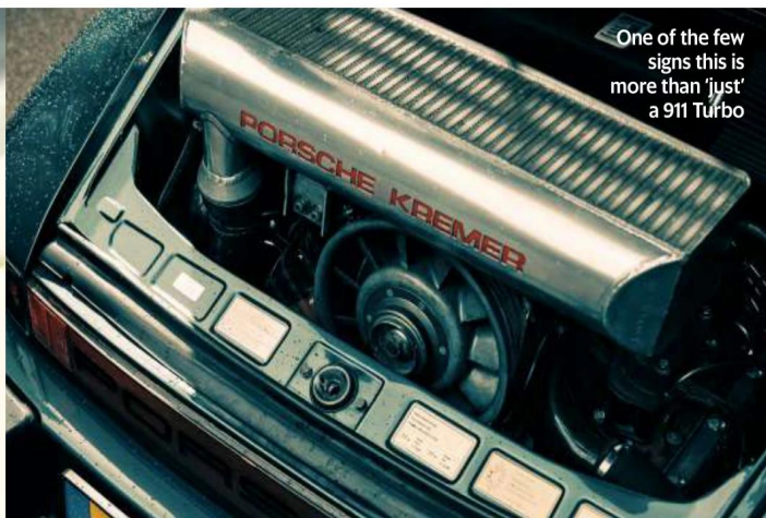
Kremer K7 turbo helps it to deliver 389bhp
