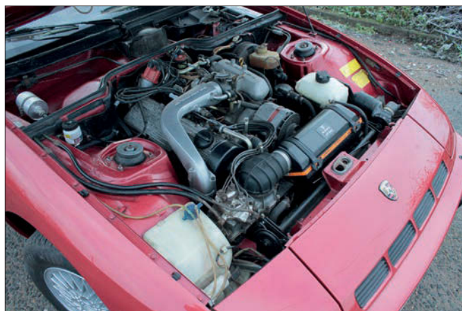
This Turbo is an import: UK cars had the four spoke Lux wheel. Forced induction meant 170bhp... and turbo lag!
