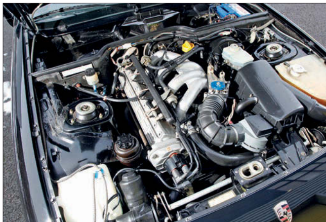
The 924S used a detuned 944 engine, not the earlier EA831.
