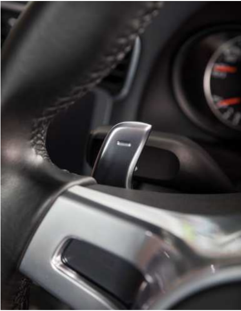
ABOVE PDK serves as an excellent tool for extracting big power from the Turbo S's 560hp 9A1 engine when called upon, also offering the dexterity of a 16 per cent improvement in MPG
