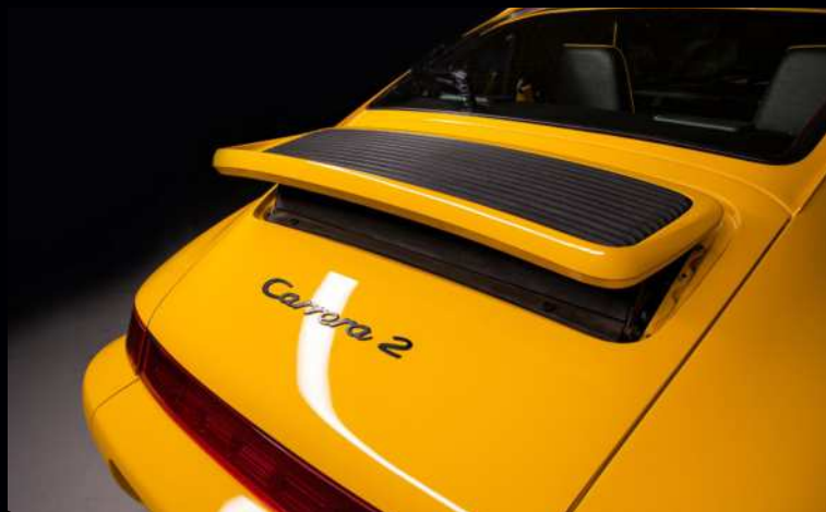
ABOVE New active rear wing raised at 50mph, lowering again at 6mph. Twin-plug flat six boosted power and efficiency, and inside, the 911's ventilation was at last simplified
