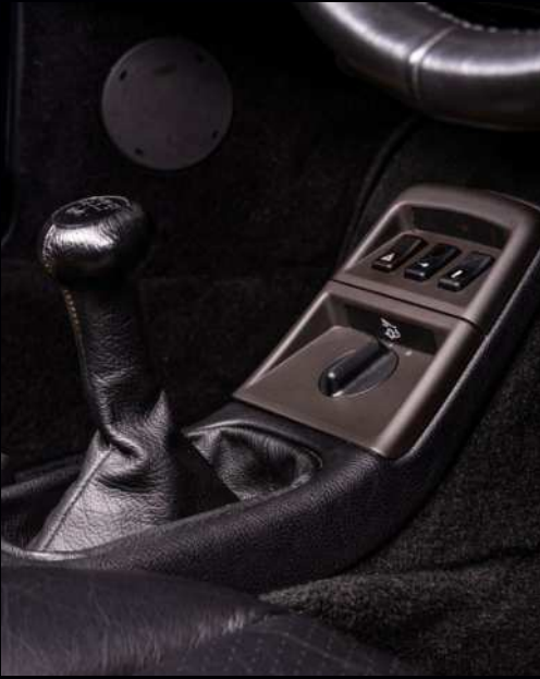
ABOVE New centre console with shorter gear shifter was taken conceptually from the 959
