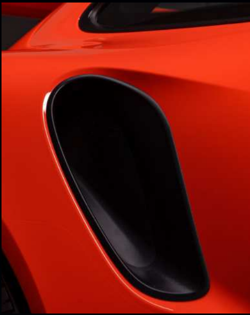
ABOVE Turbo-wide body used its side intakes to feed air directly to the engine for the first time on a 911 Rennsport
