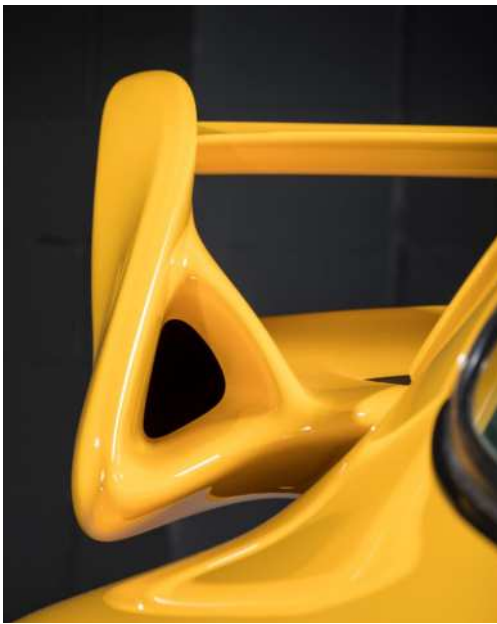
ABOVE Bi-planed wing was unique to the Clubsport; Comfort RSs had a flatter one-piece item
