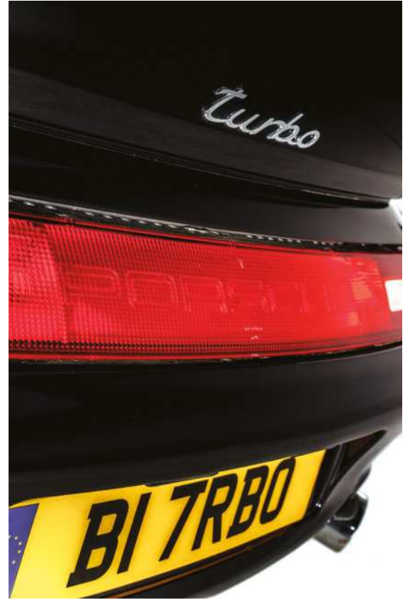
The reflective strip connecting the rear clusters also housed the reverse and fog lights, and wouldn't appear on a 911 again until the 996 C4S, 997.2 C4 and the new 991 C4
