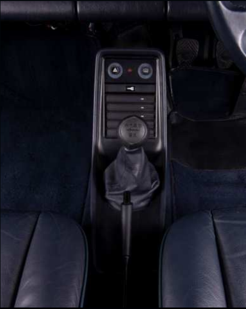
ABOVE G50 gearbox (above) is more desirable than the 915 gearbox, where reverse is down and right
