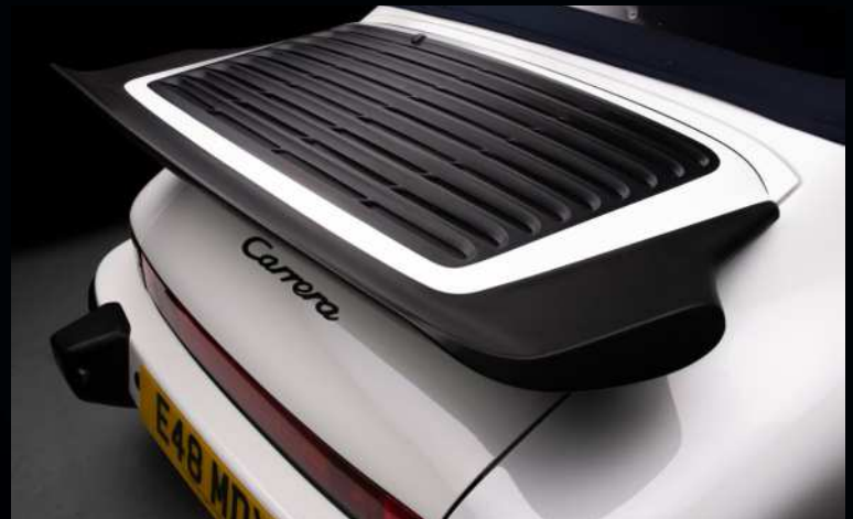
ABOVE Tea tray rear wing and front lip spoiler were part of the optional 'Sport' package
