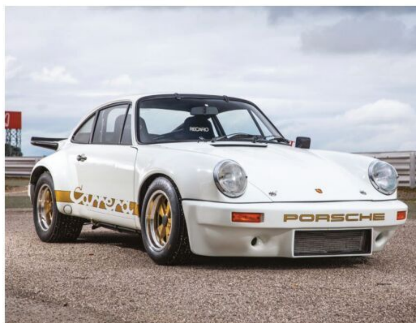
ABOVE Whale tail would later find its way onto the 930 3.0, though RS 3.0's was wider
