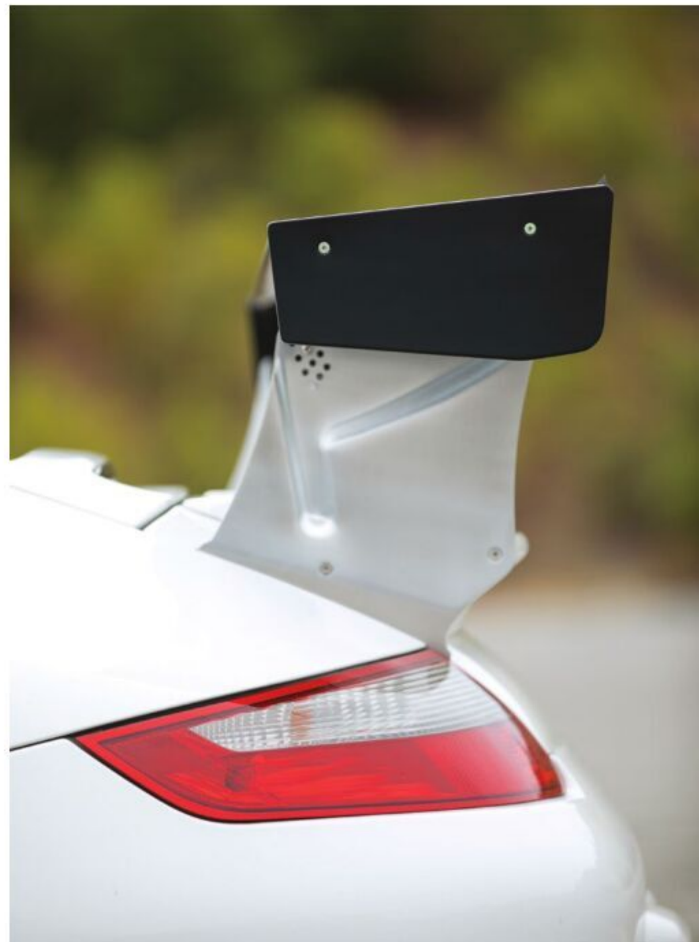
ABOVE 997.1 GT3'S aero package includes hero downforce-spec Cup wing
