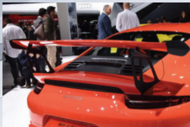
A carbon fibre rear wing sits higher than any previous Rennsport, helping the new GT3 RS produce twice as much downforce as the RS 4.0.
