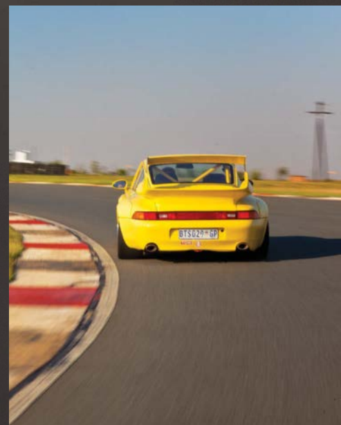
Right: ...while the huge bi-planed rear wing aids downforce when the 993 reaches big speeds
