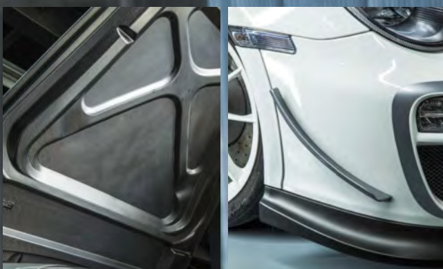
Lightweight plastics and carbon fibre again made up the body of the very last 997 GT3 RS, paired with a reworked engine and better aerodynamics
