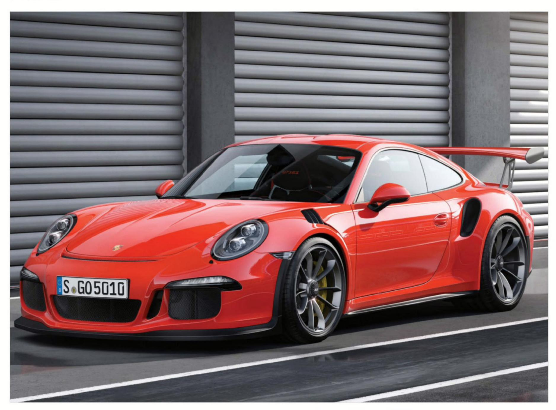
The latest GT3 RS adopts the Turbo's ultra-wide body and packs a four-litre DFI engine with a new crankshaft over the 991 GT3. Lighter than a GT3 thanks in part to a magnesium roof and front bonnet.
