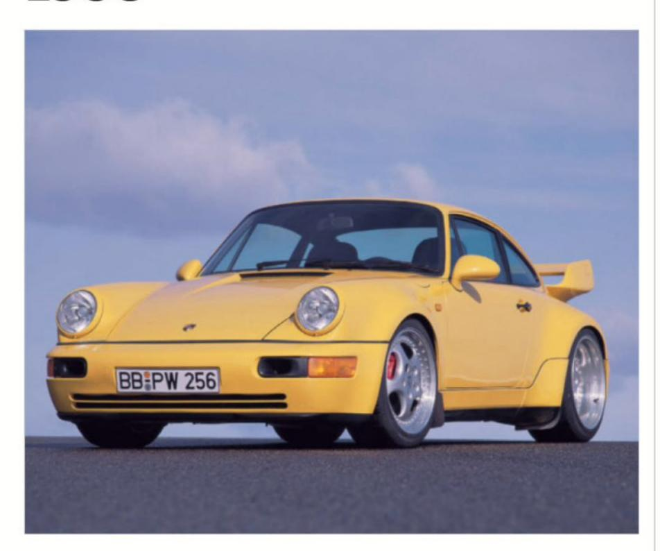
Identifiable by a lightweight Turbo bodyshell, large rear spoiler and 18-inch Speedline wheels. Power came from a new 3.8-litre unit with hot-film air sensor and twin exhaust.
