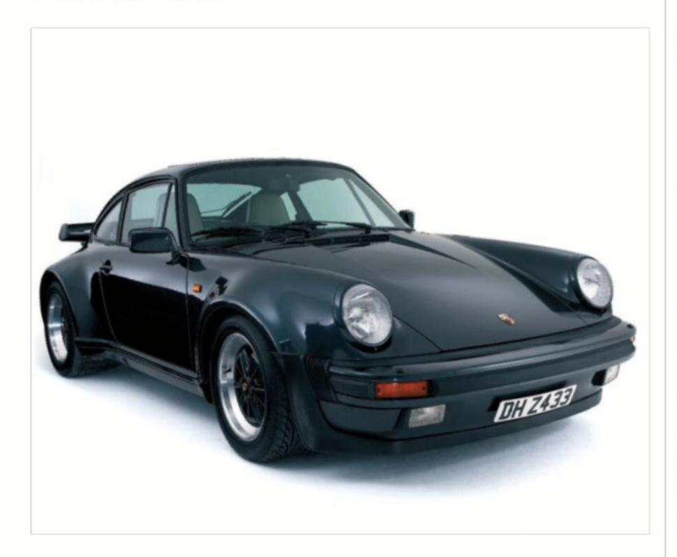
Larger engine resulted in an extra 40bhp, and an intercooler on top of the engine led to the adoption of a new 'tea tray' spoiler. Brakes were upgraded from 917 racer.
