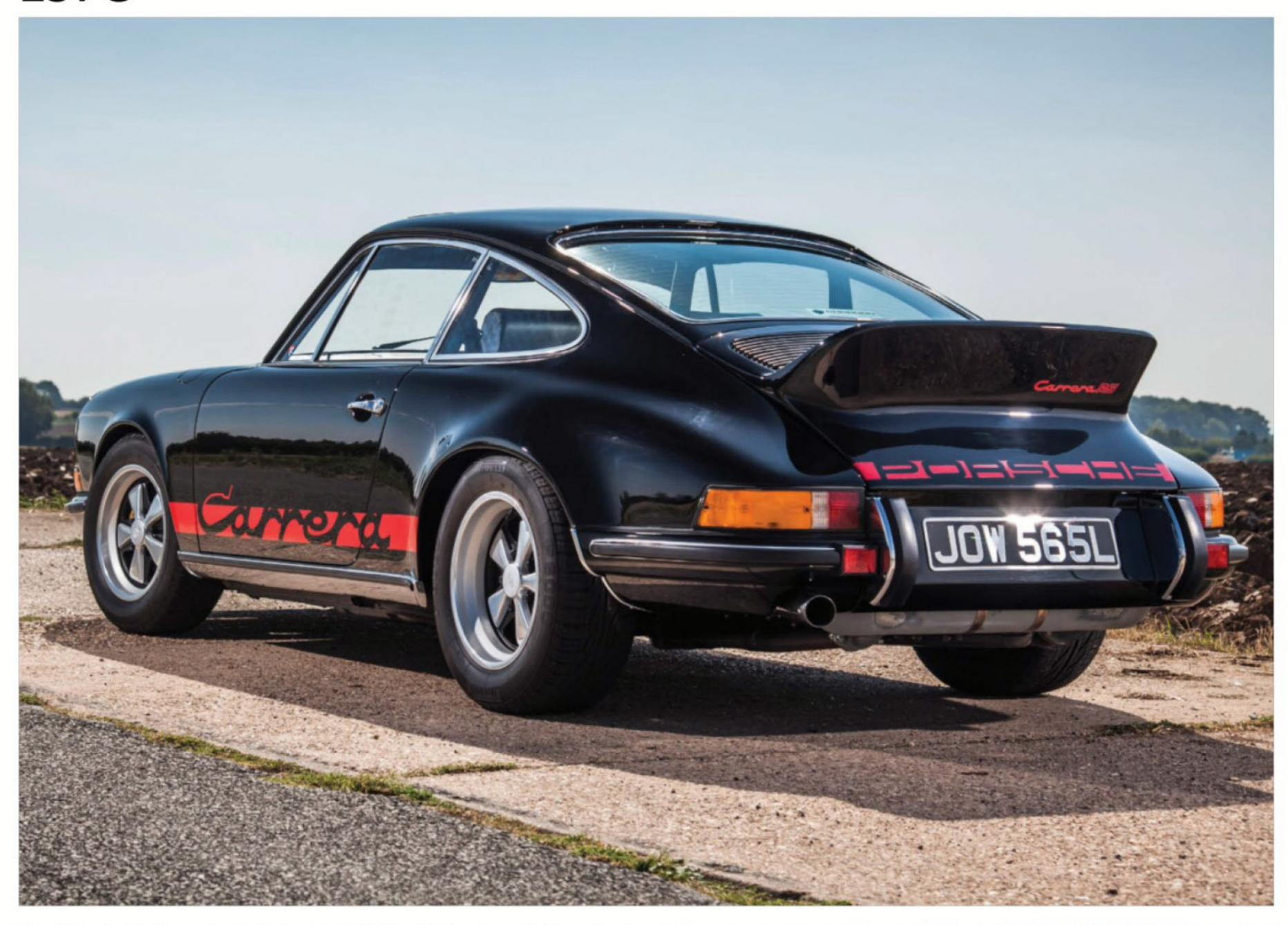
The RS had a 2,687cc engine that developed 210bhp. The body was lightened and fitted with flared rear arches and an optional ducktail spoiler. Sport and Touring versions available.
