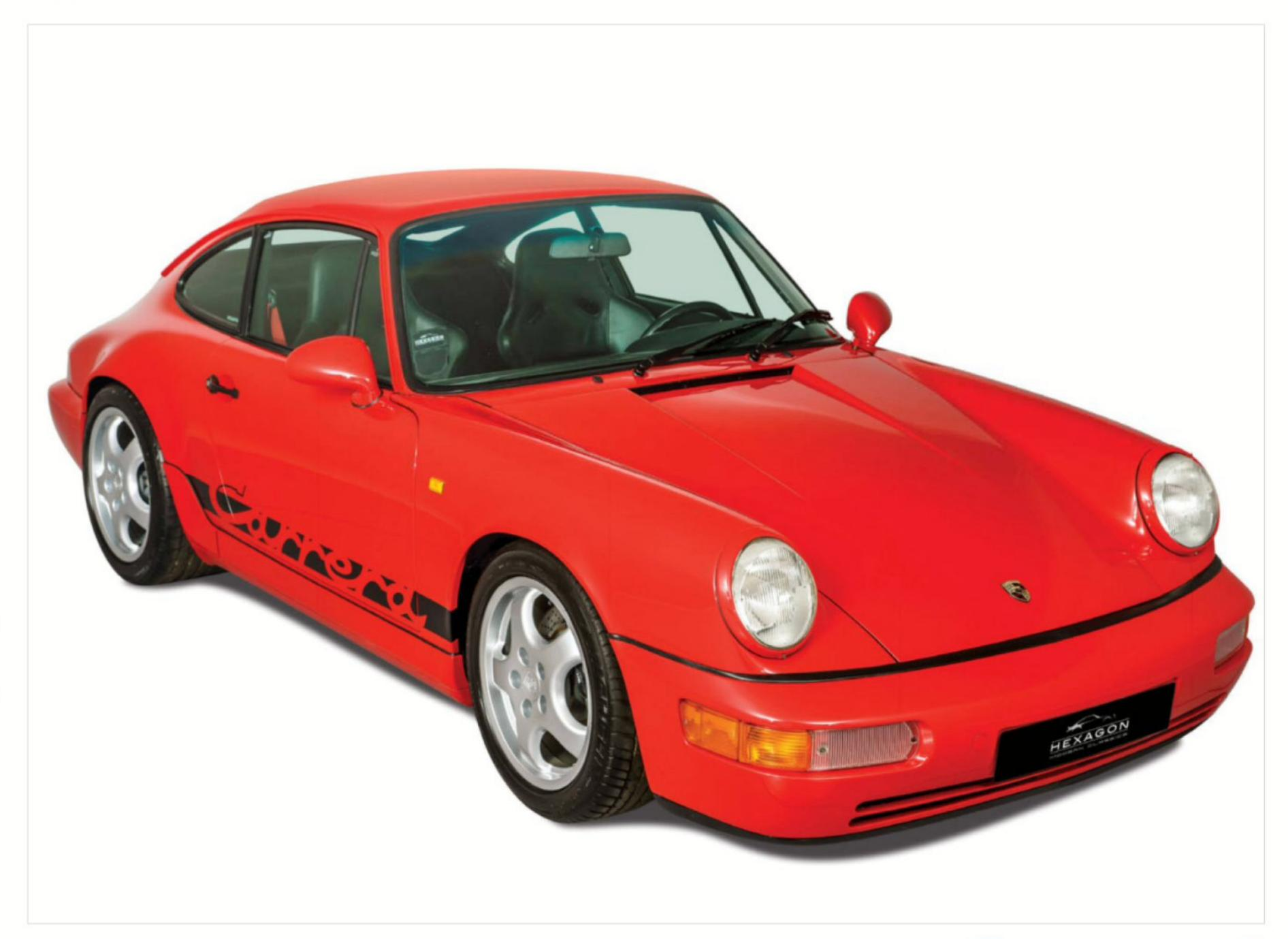
Around 120kg saved by deleting 'luxuries' and fitting magnesium Cup wheels. Power was boosted by 10bhp, suspension lowered by 40mm and uprated, as were brakes.
