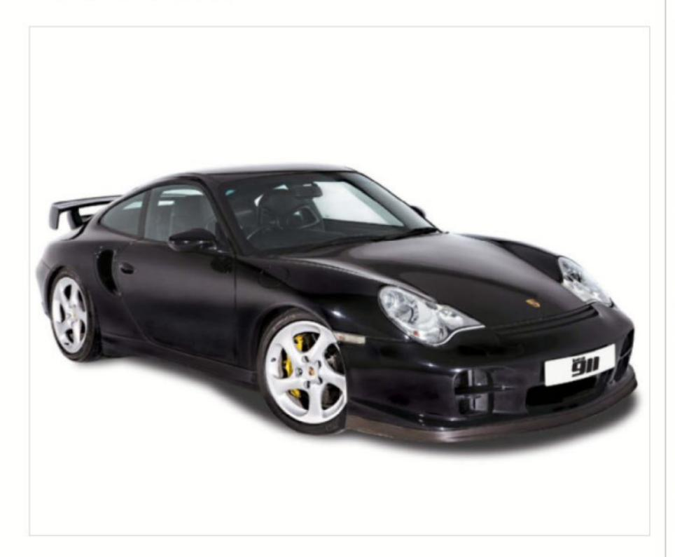
A lightweight, Turbo-bodied 996 with uprated turbocharged engine and suspension. PCCB was standard. Revised ECU later gave an extra 21bhp.
