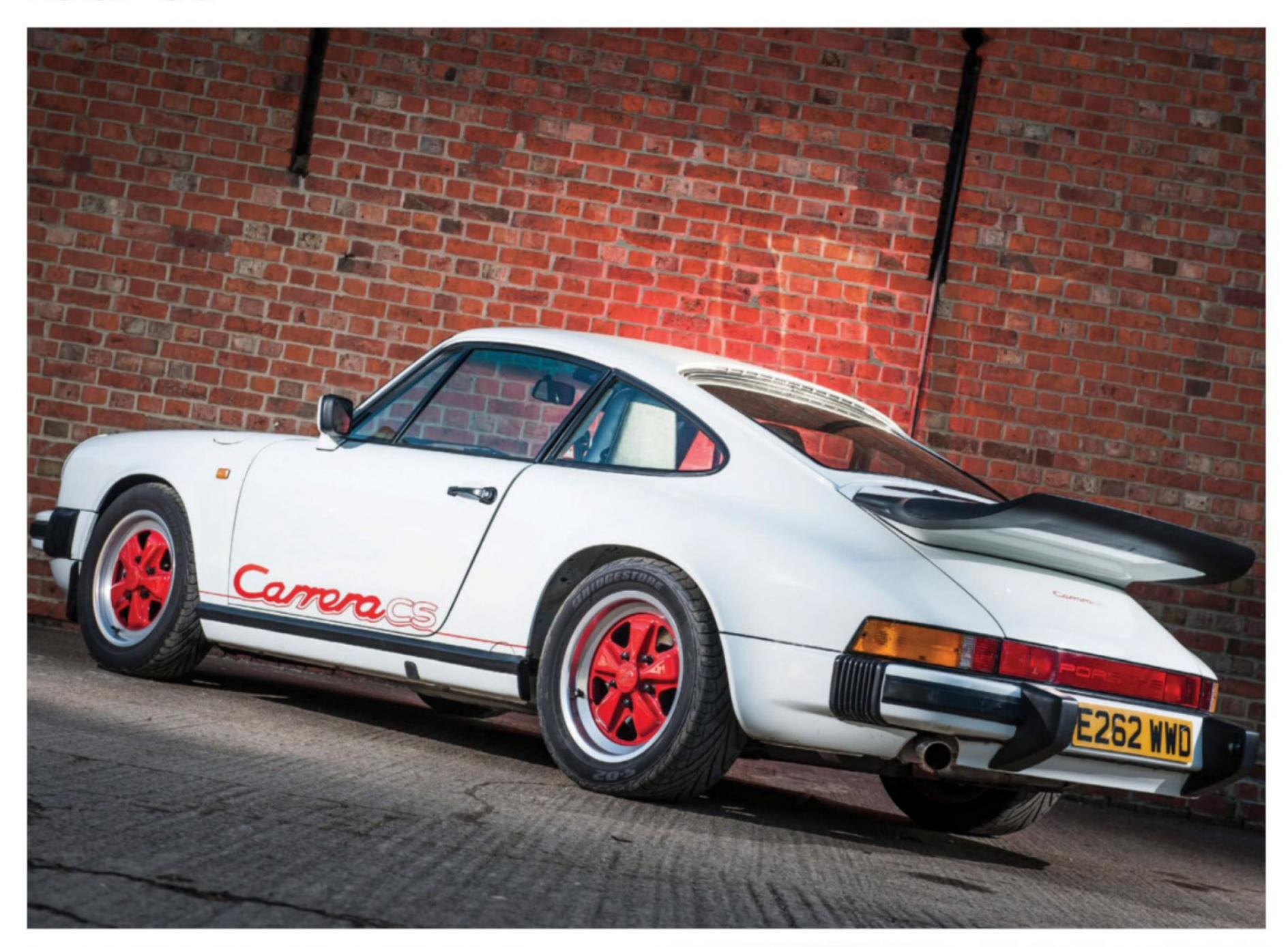
Removing 'luxuries' sliced off around 40kg of weight. Revised engine management gave a higher rev limit of 6,840rpm. Suspension uprated and LSD standard.
