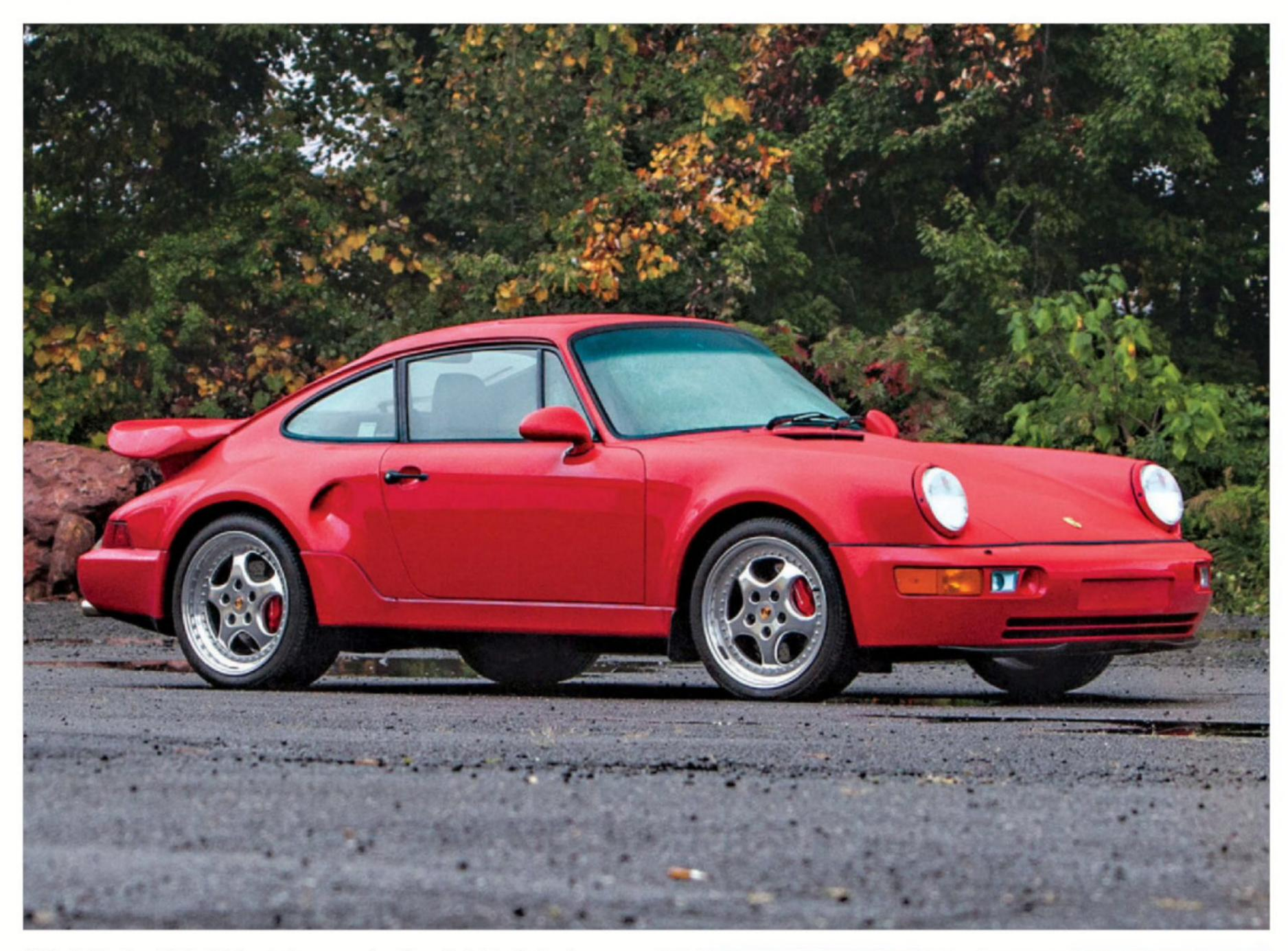
180kg lighter than Turbo. Intakes in the rear arches funnelled air to the brakes, while the engine power was boosted by 61bhp. RS-spec uprated suspension.
