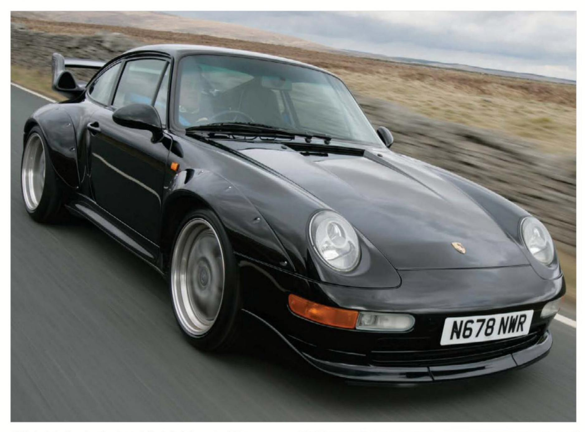
911 Turbo, but with reduced equipment. Also included rear-wheel-drive, making it a better track car. Fitted with huge front and rear spoilers and bolt-on arch extensions.
