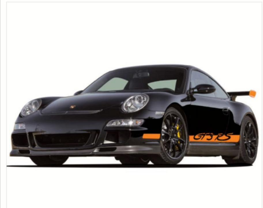
Similar to GT3, with inclusion of wider rear bodyshell of the Carrera S. 20kg of weight saved from GT3 thanks to carbon engine cover and rear wing, and plastic rear window.
