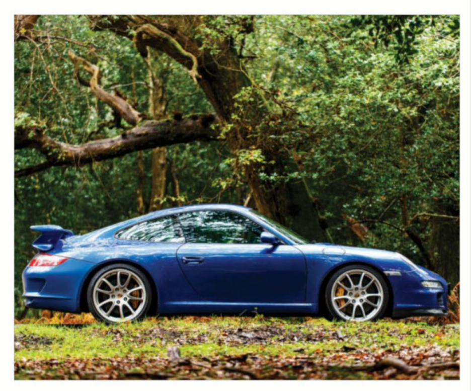
Track-focused, but based on narrow-bodied Carrera with reworked 996 GT3 engine. PASM standard, revs to 8,400 rpm, 200 higher than the Gen 2996 GT3.
