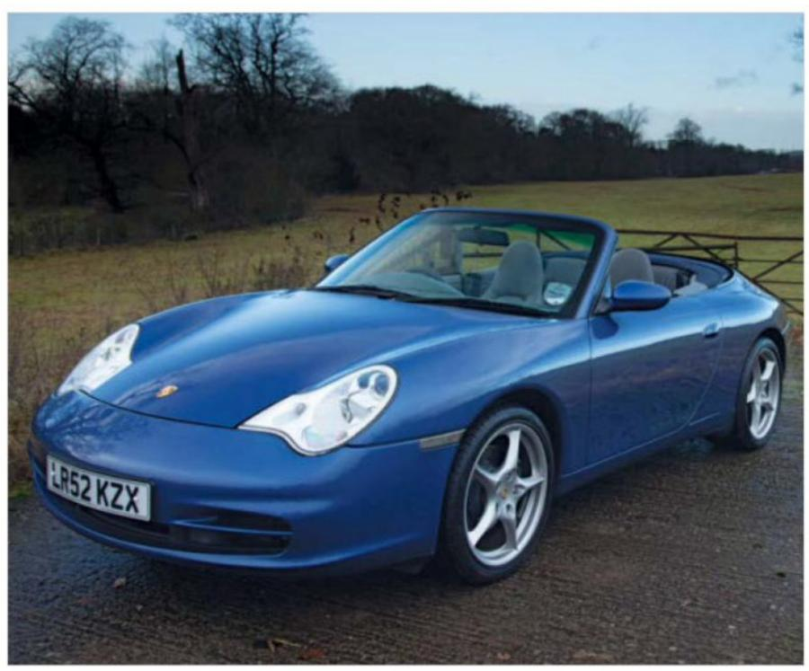
Facelifted with Turbo-style headlamps and revised front and rear bumpers, fitted with more powerful 3.6-litre engine and VarioCam Plus. Manual and Tiptronic 'boxes updated.
