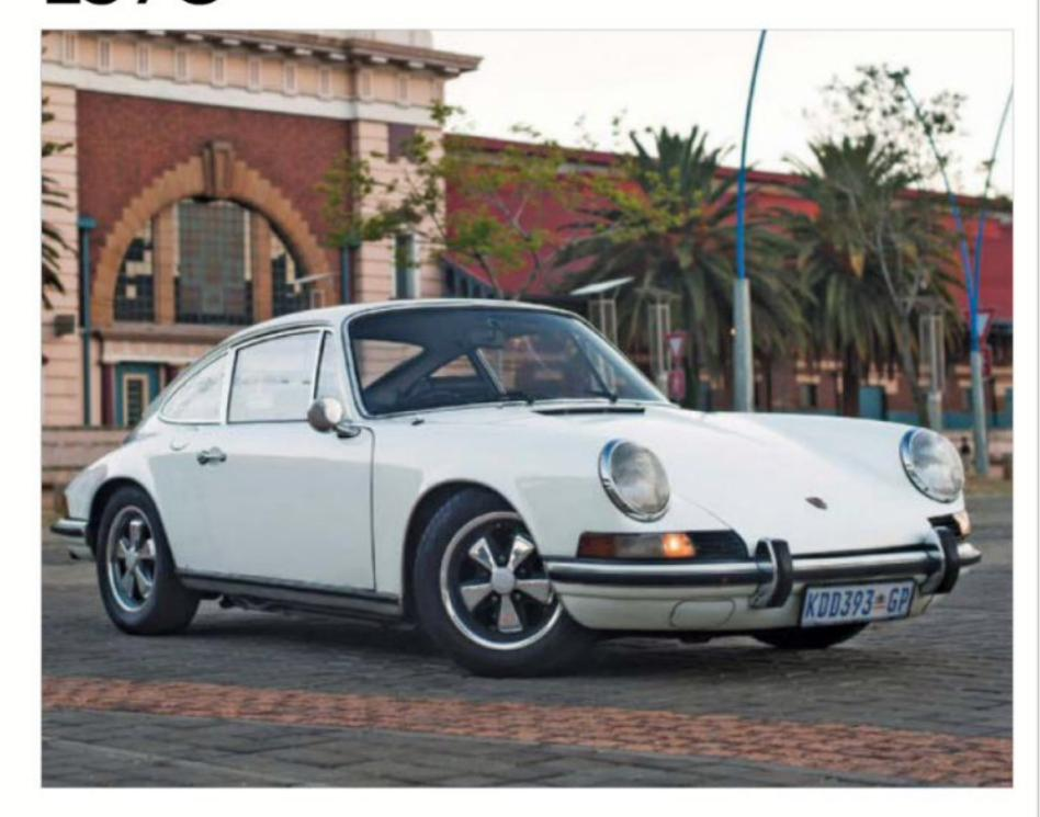
After incidents of people filling E series 911s with petrol via the external oil-filler, the filler returned to under the engine decklid. Fitted with the front spoiler of the 911S.
