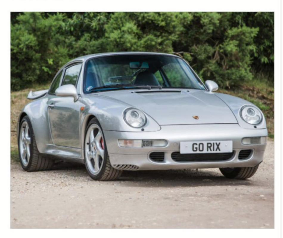
Fitted with two KKK turbochargers in order to reduce lag. Power went to all four wheels using the Carrera 4's transmission system. Brakes were 'Big Reds'.
