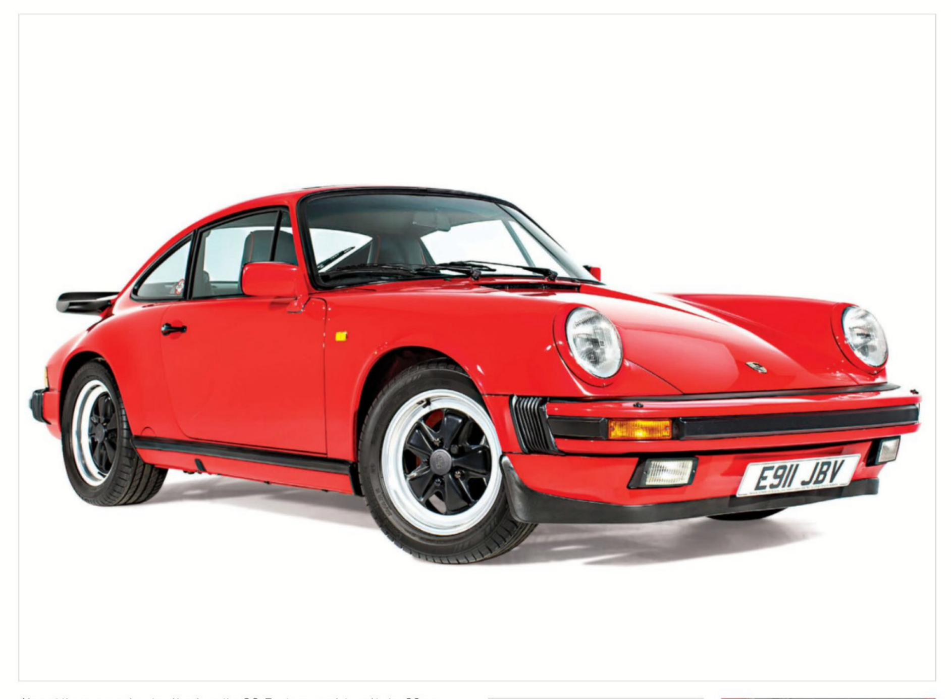
Almost the same galvanised body as the SC. Engine was claimed to be 80 per cent new, and the first production 911 to feature an ECU to control ignition and fuel systems.
