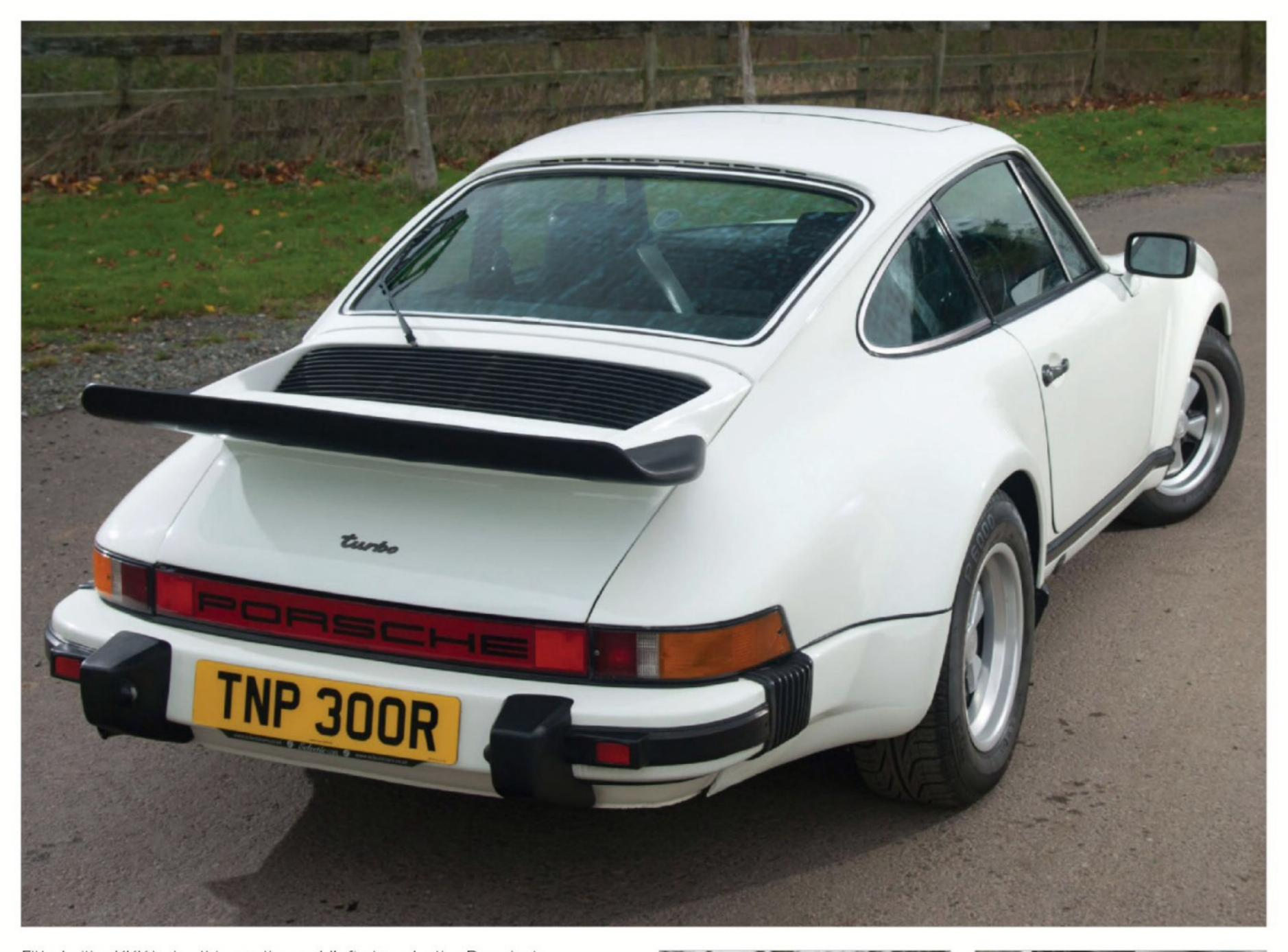
Fitted with a KKK turbo, this was the world's first production Porsche to be turbocharged. Flared arches, whaletail spoiler and four-speed gearbox were standard.
