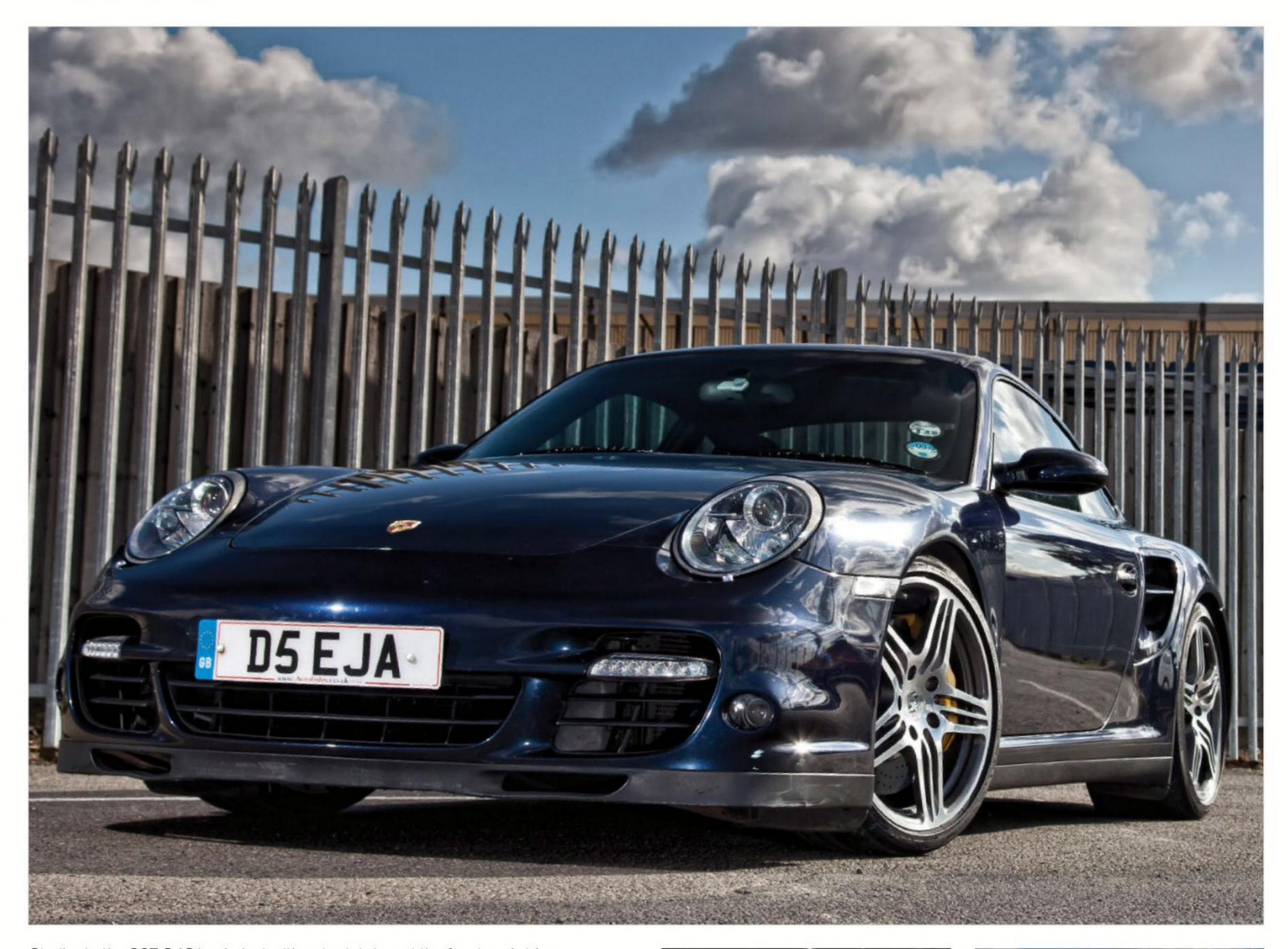
Similar to the 997 C4S body, but with extra intakes at the front and sides. Essentially the 996 Turbo engine, but with all-new twin turbos. VTG gave the best of small and large turbos.
