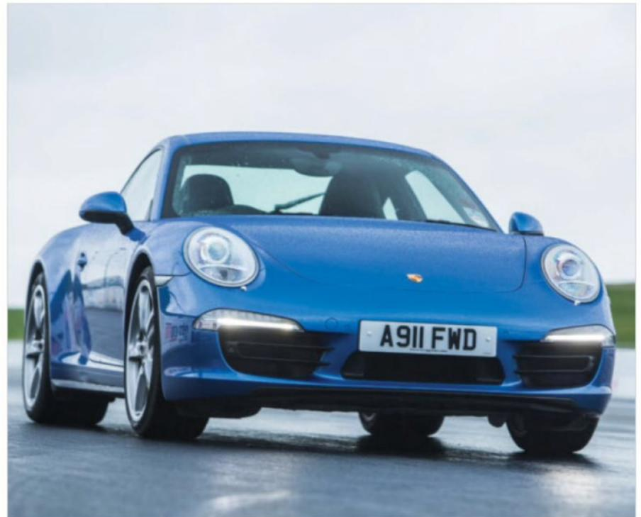
Same wider body styling as Carrera 4, coupled to a 3.8-litre 400bhp engine. Also features six-piston brake calipers at front, as opposed to four.
