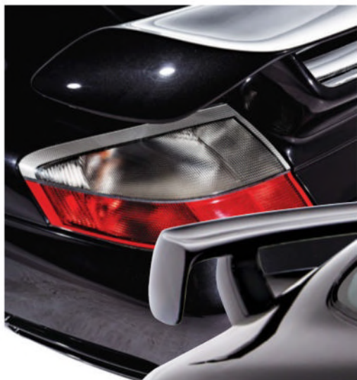
The rear bumper was lifted from the Turbo, but the dual rear spoiler was unique, with the top section being adjustable through five degrees
