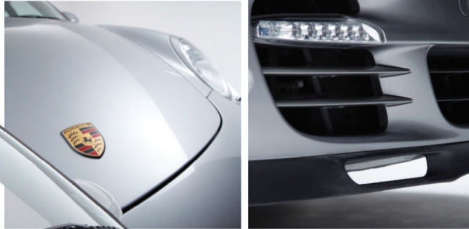
The front spoiler aids aerodynamics and feeds air to the brakes
