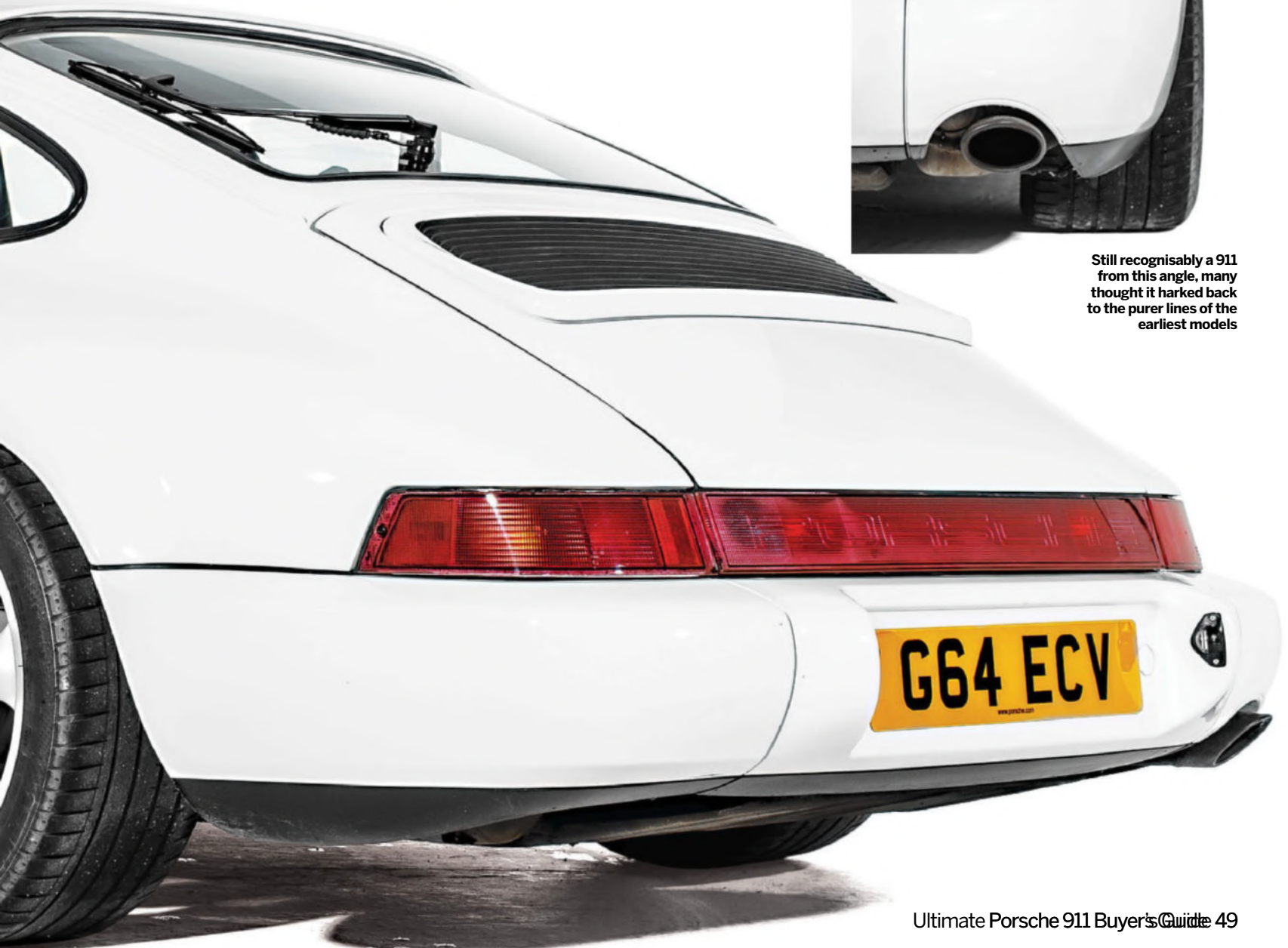
The trademark fixed rear spoiler disappeared on the 964, replaced by this pop-up item that helped with engine cooling
