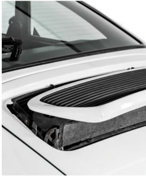
The trademark fixed rear spoiler disappeared on the 964, replaced by this pop-up item that helped with engine cooling
