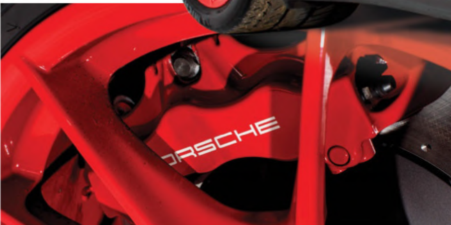
Centre-locking wheels hide huge 380mm brake discs and iconic Big Red callipers
