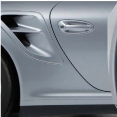
The wider Turbo body caters for vents in the rear arches that feed air to the intercoolers
