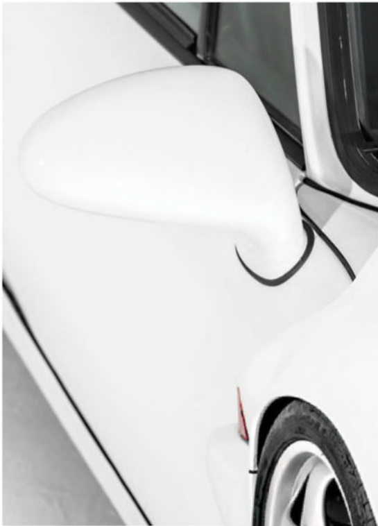
Teardrop mirrors were a more modern touch and contributed to the impressive aerodynamics
