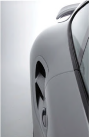
The wider Turbo body caters for vents in the rear arches that feed air to the intercoolers
