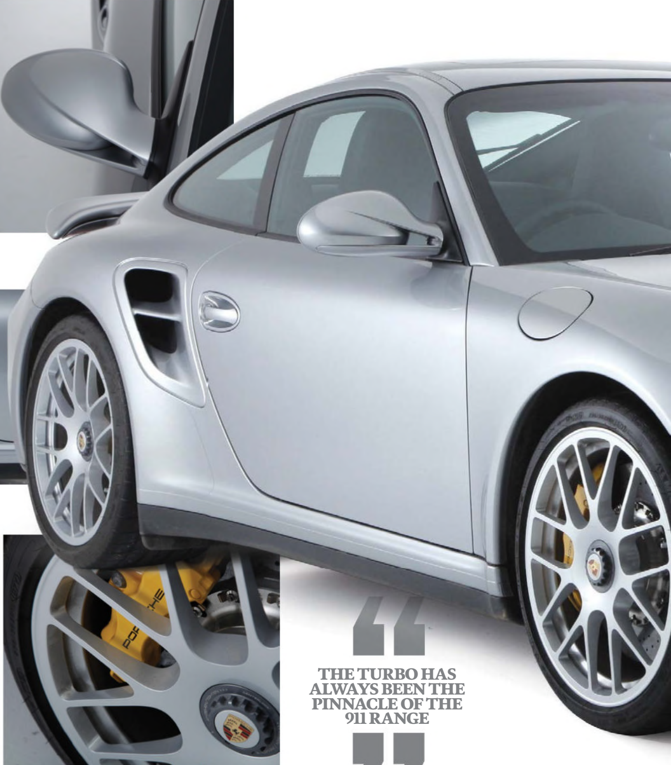
Big yellow brake calipers are another sure sign of a Turbo S, while ceramic discs eliminate brake dust
