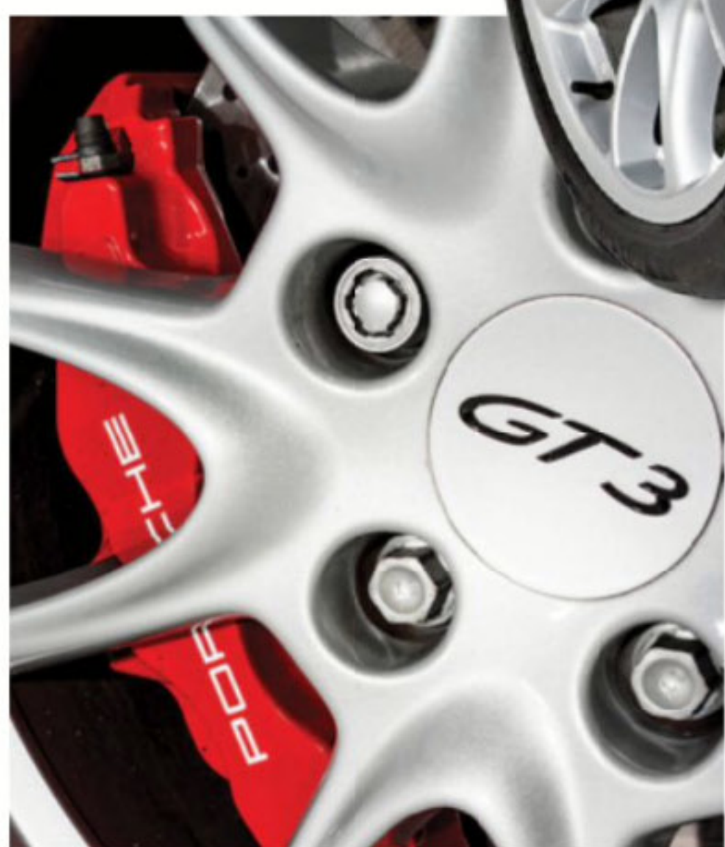
Five-stud, 19-inch wheels came on the 997.1 GT3. Centre-locking items were used on the facelift
