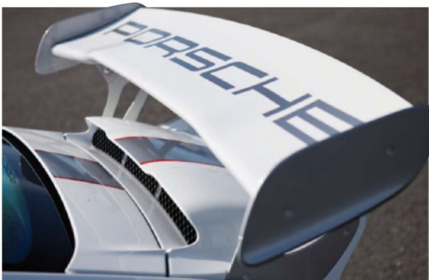
Rear wing is more steeply raked (left) than before and works in conjunction with front 'flics' to give greater downforce
