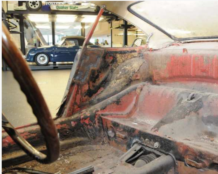
LEFT More than 50 per cent of the car's original metalwork could be saved, despite heavy rust BELOW A leather sleeve around chassis 57's gear shifter was unique to 901s of this vintage
