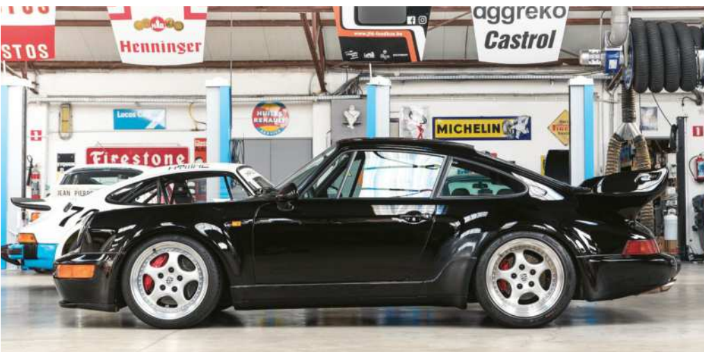
LEFT Wide body, fixed wing and Speedline wheels visually mark the 3.8-litre RS from the 3.6
