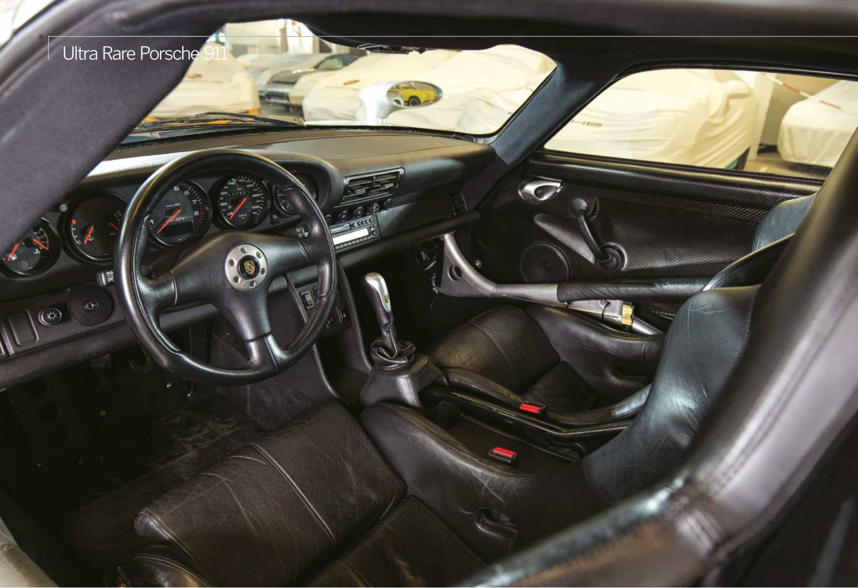
Above Inside the GT1, the steering wheel, dashboard, five dials, gearlever and even the seats are all reminiscent of a 993 RS specification. Note the 996-generation door handles, however Below Large intake above cockpit feeds air into the mid-mounted, 3.2-litre flat six engine behind the driver and passenger. Entire rear of carbon kevlar body can be opened with a key in each B-pillar
