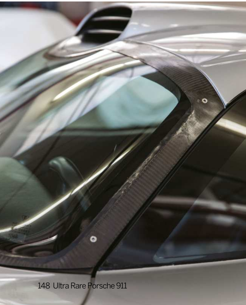
Above Inside the GT1, the steering wheel, dashboard, five dials, gearlever and even the seats are all reminiscent of a 993 RS specification. Note the 996-generation door handles, however Below Large intake above cockpit feeds air into the mid-mounted, 3.2-litre flat six engine behind the driver and passenger. Entire rear of carbon kevlar body can be opened with a key in each B-pillar
