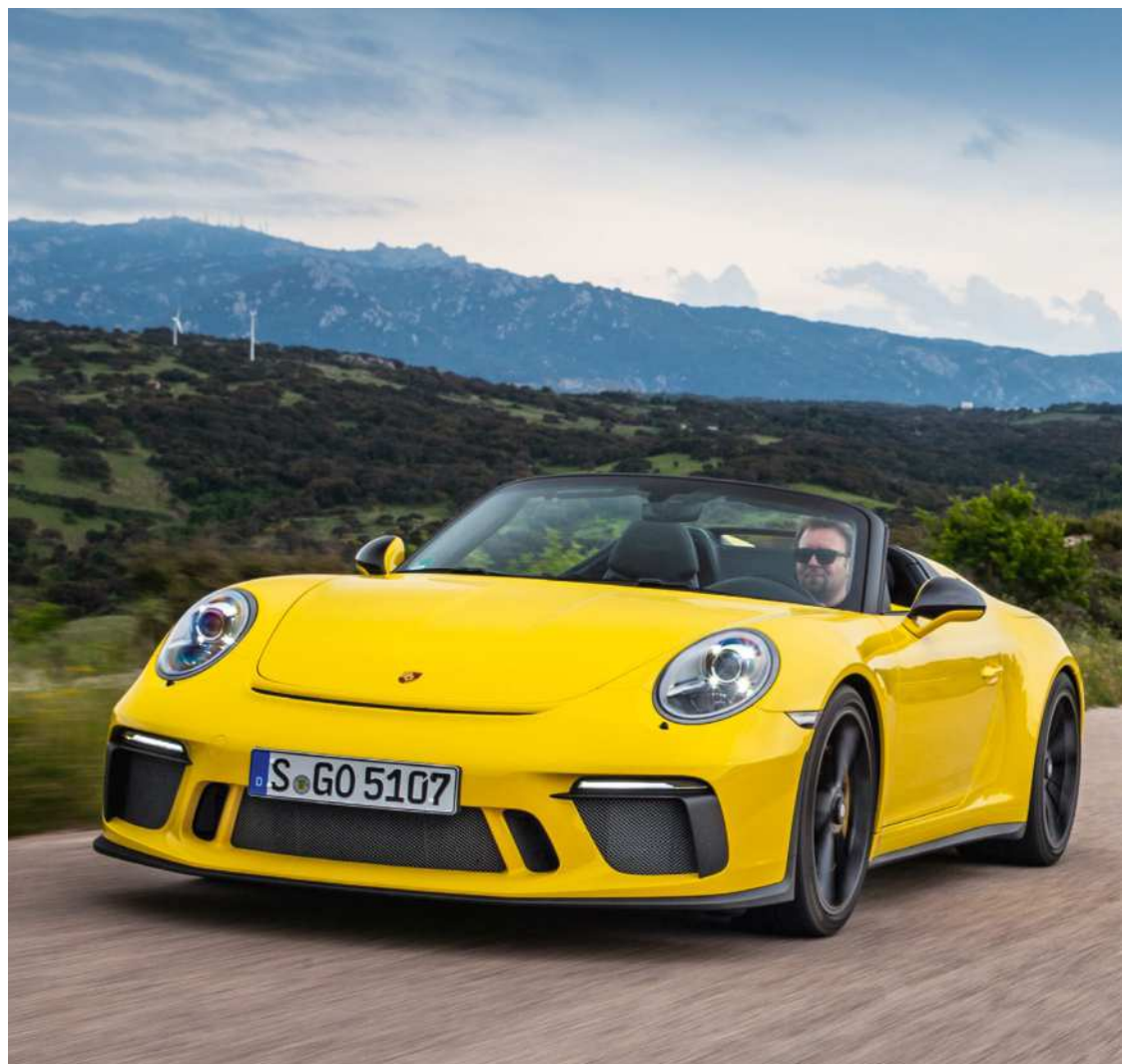
BELOW 991's windscreen is shorter and more steeply raked, in true Porsche Speedster fashion
