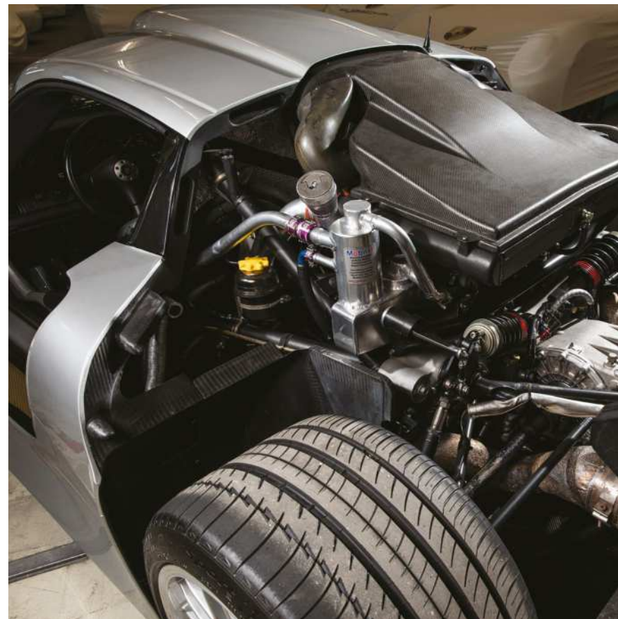
Above Inside the GT1, the steering wheel, dashboard, five dials, gearlever and even the seats are all reminiscent of a 993 RS specification. Note the 996-generation door handles, however Below Large intake above cockpit feeds air into the mid-mounted, 3.2-litre flat six engine behind the driver and passenger. Entire rear of carbon kevlar body can be opened with a key in each B-pillar
