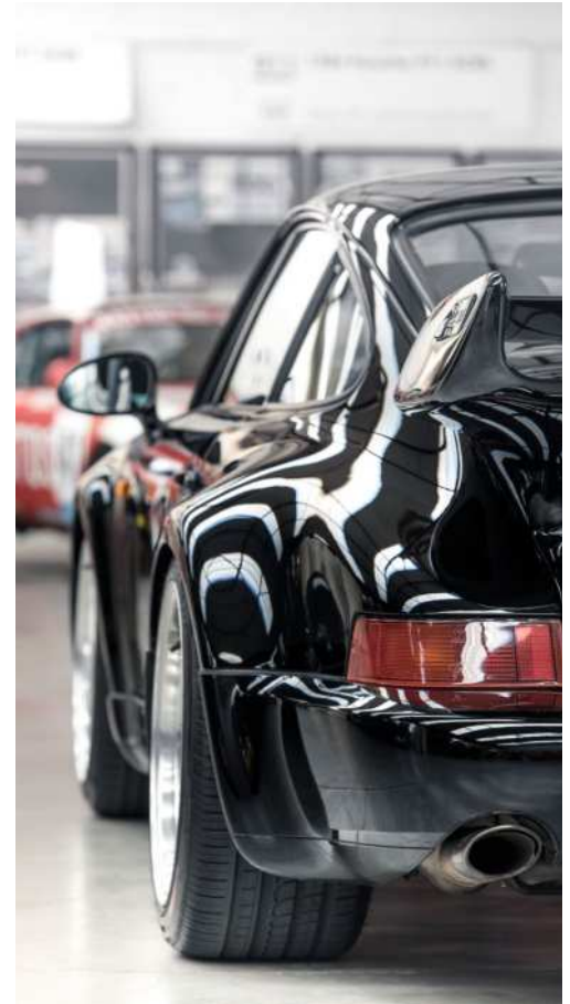
LEFT Wide body, fixed wing and Speedline wheels visually mark the 3.8-litre RS from the 3.6
