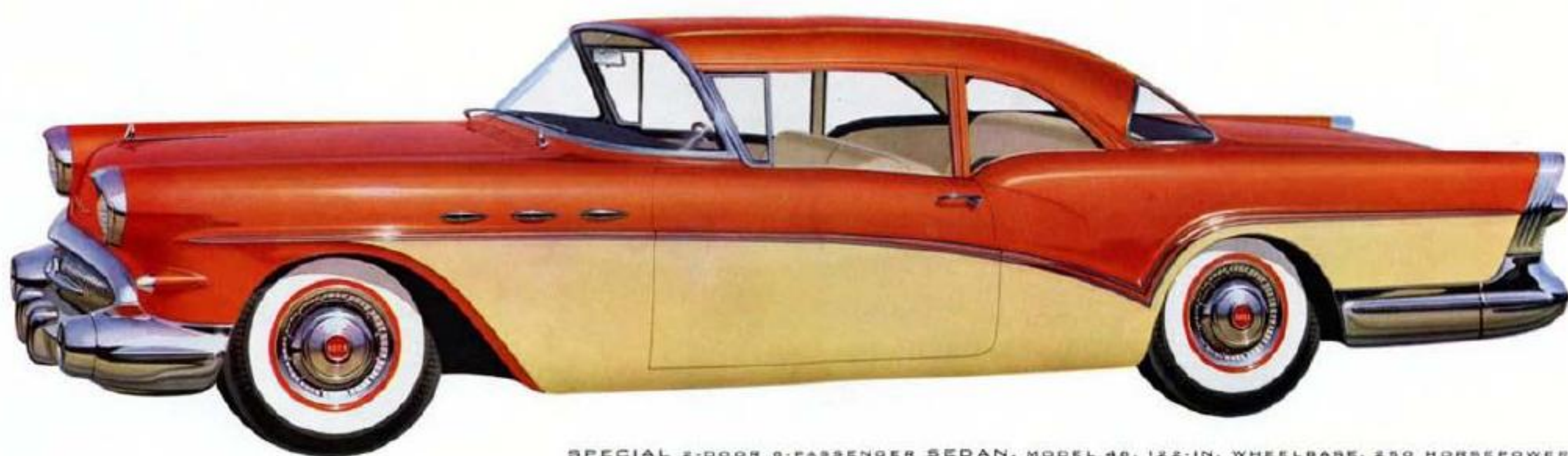
SPECIAL 2-DOOR 6-PASSENGER SEDAN, MODEL 46, 122-IN. WHEELBASE, 250 HORSEPOWER
