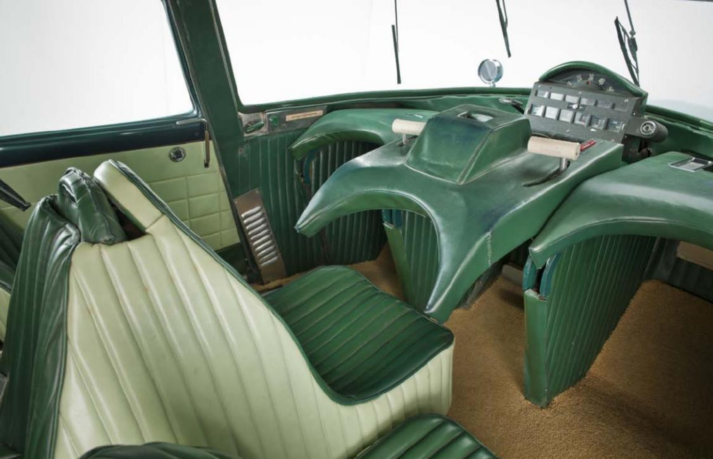
The Cornell Liberty car interior. Note web-style head restraints, wrap around seats and loads of crash padding. Driver sat in the middle of the car. Steering was by the two, white handled levers.
