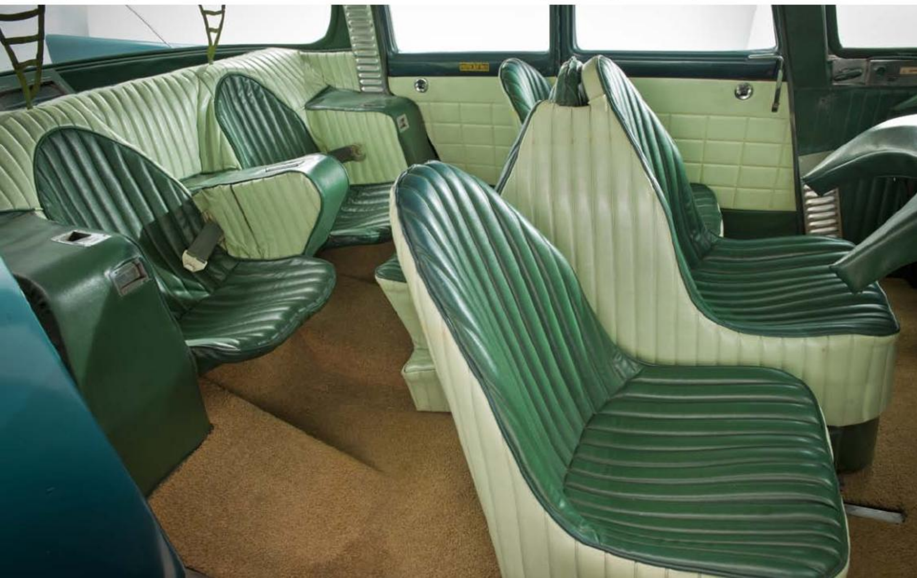
The Cornell Liberty car interior. Note web-style head restraints, wrap around seats and loads of crash padding. Driver sat in the middle of the car. Steering was by the two, white handled levers.
