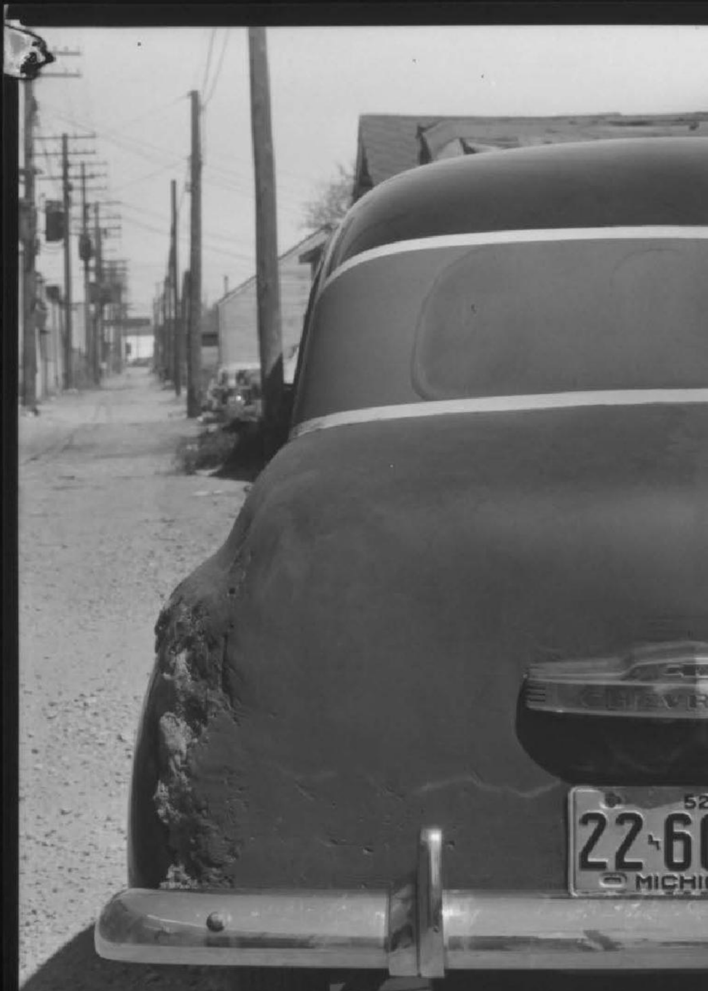
FG Holden: The modelling clay can be seen clearly in this photo. The car is not finished on the left side and has Chevrolet badge on the boot lid. The outline of the FX rear window can again be seen under the fake wrap around window.
