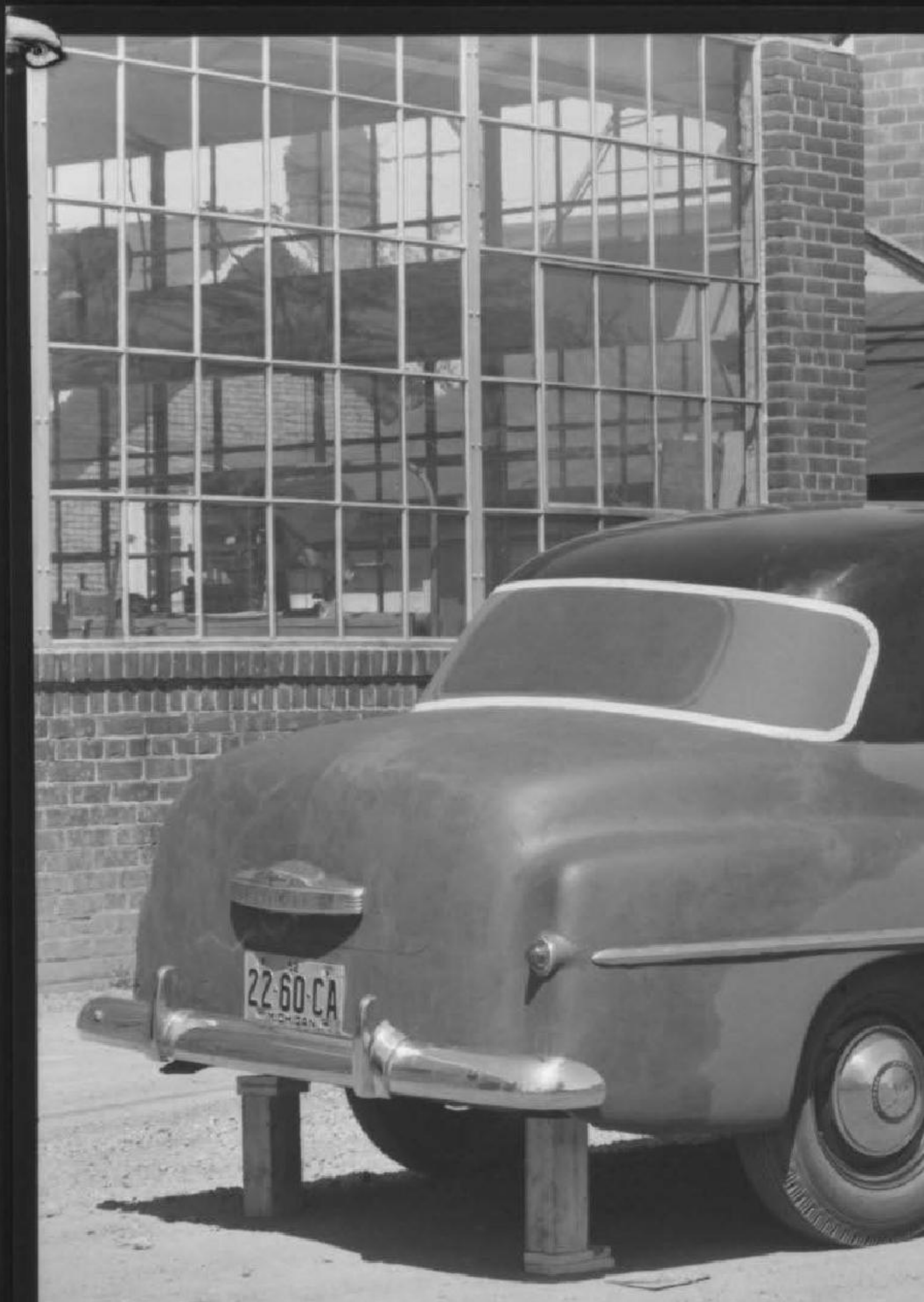
FG Holden: GM stylists have applied clay over the rear of an FX to reshape the car. The clay is so heavy it needs two wooden blocks to support its weight, otherwise it will break off when the clay dries. Note the FX rear window shape is visible through the fake wrap around window.
