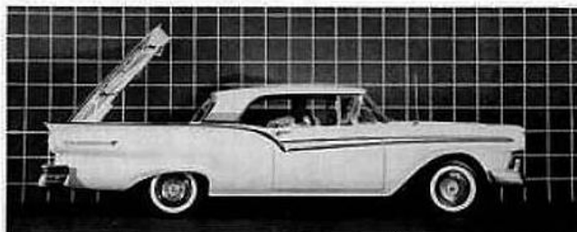
2. Smoothly, electric motors lift the rear deck lid . . .
