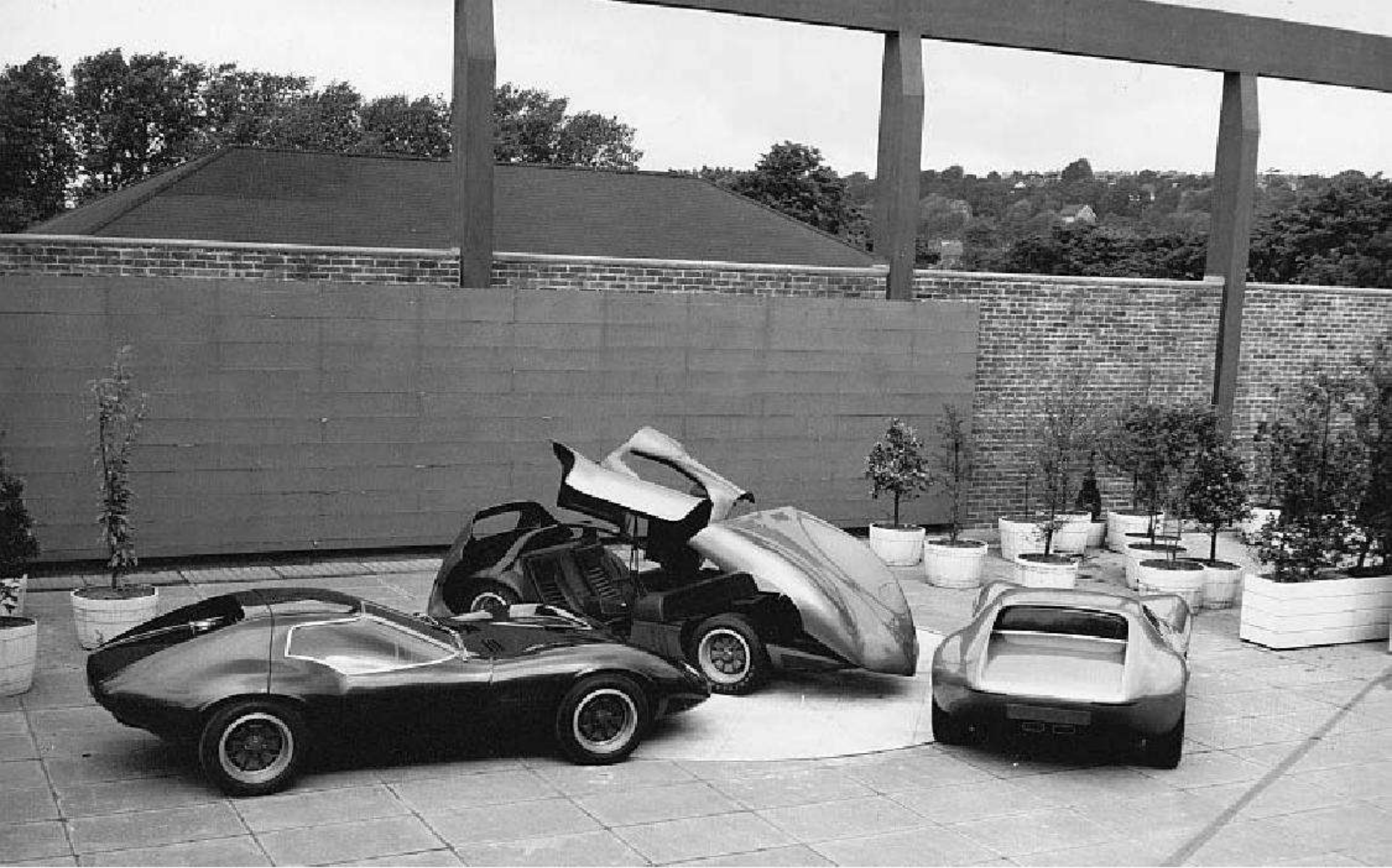
Above and below: Just four hinged openings allowed access to the entire car.
