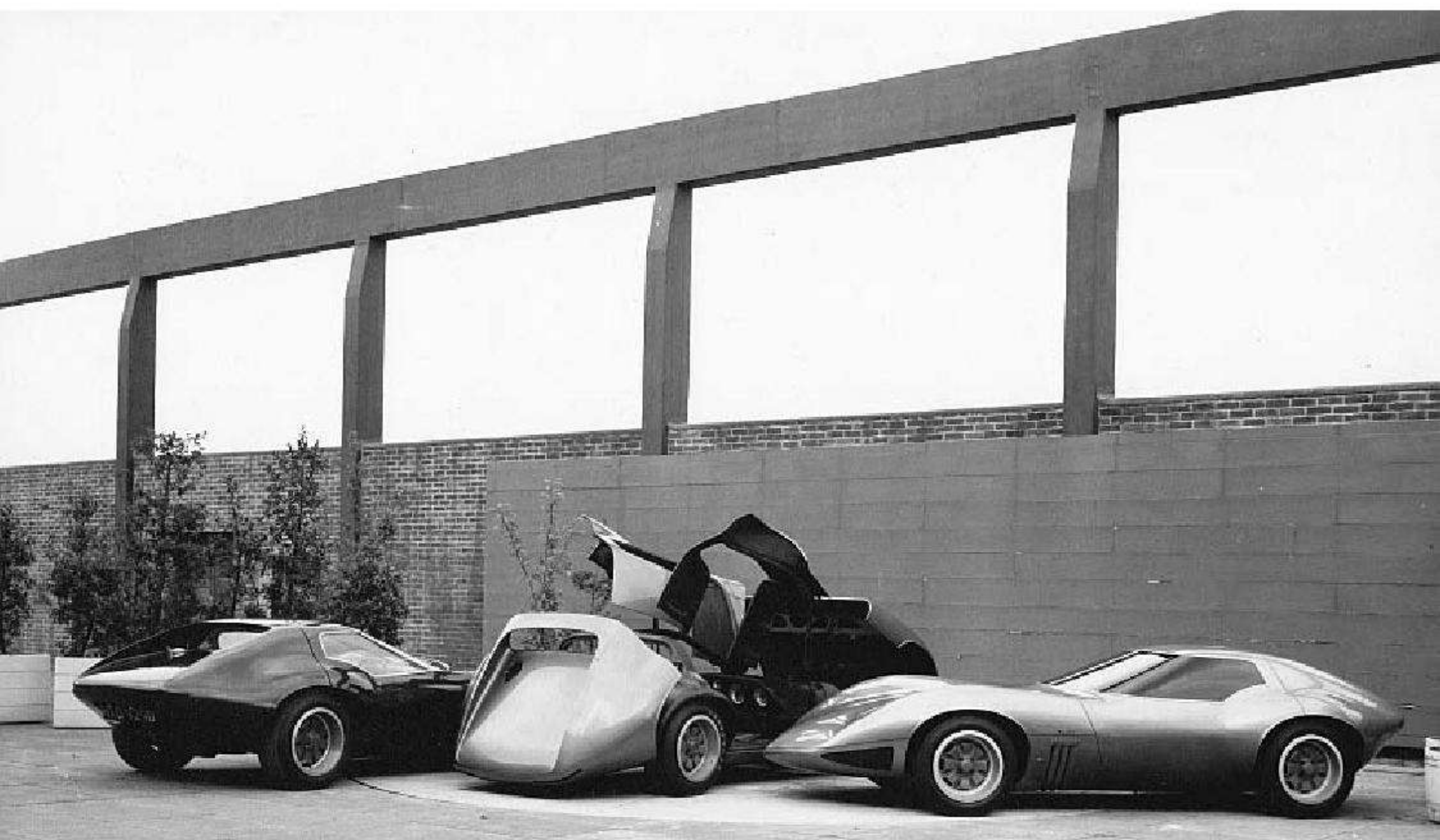
Above and below: Just four hinged openings allowed access to the entire car.
