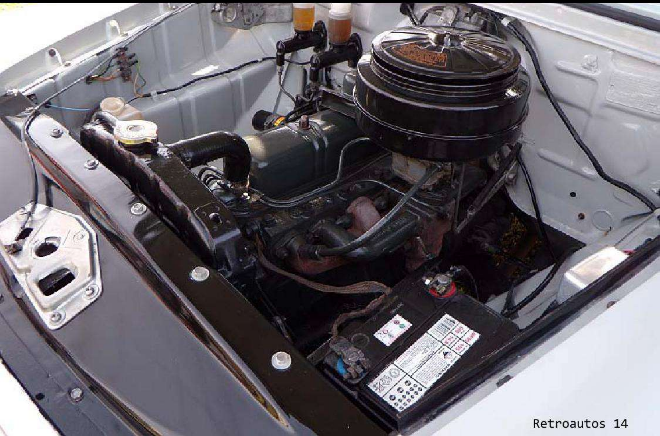
Above: A wide open chromed grille for a wide open country. Below: The 'grey' six cylinder engine that powered all Holdens from 1948 to 1962.
