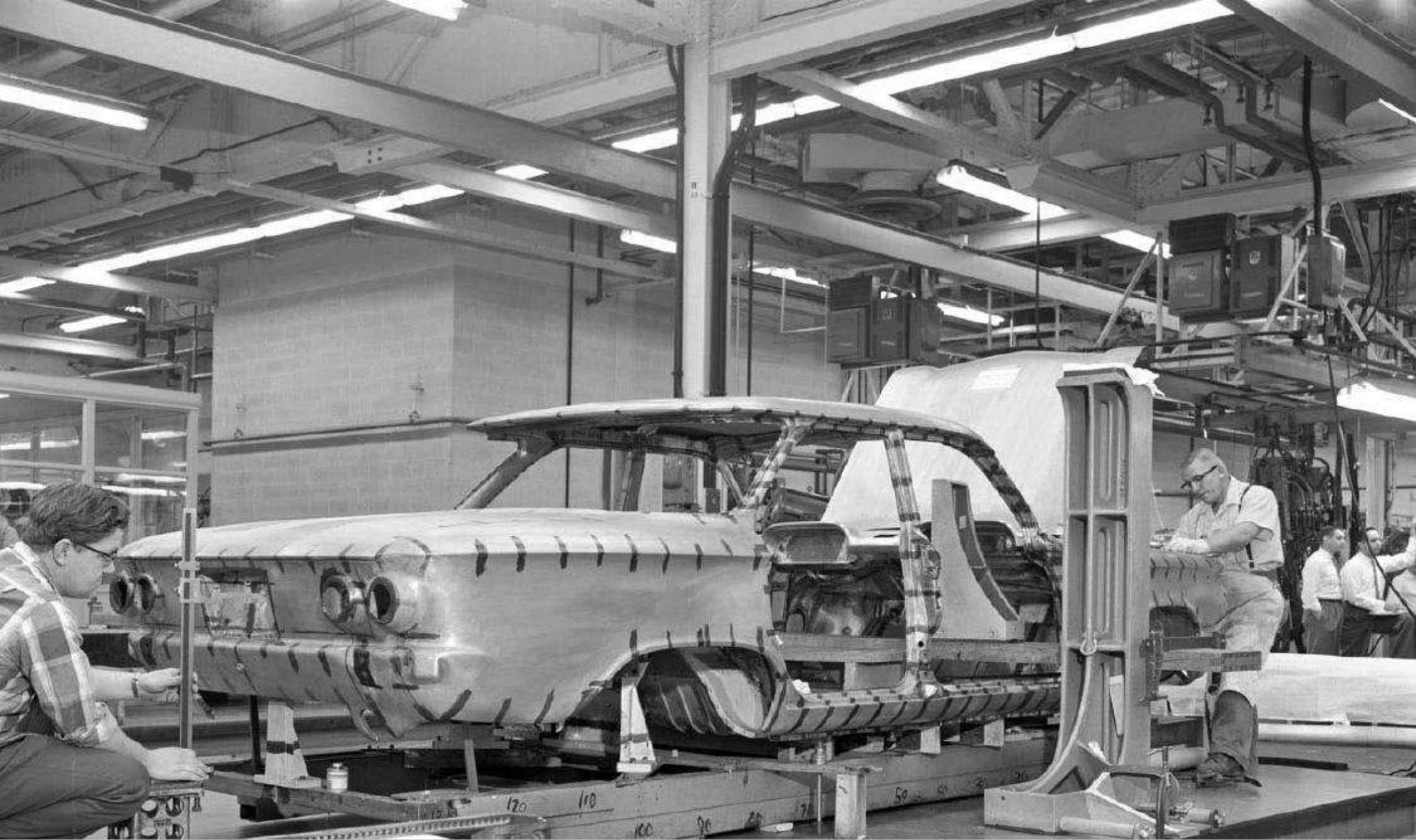
Top: The first Corvair prototype body being welded together at Fisher Body in Detroit. Below: The 1955 Chevrolet Biscayne dream car, which provided styling inspiration for the Corvair. The Biscayne also influenced the front of the 1963 Buick Riviera.
