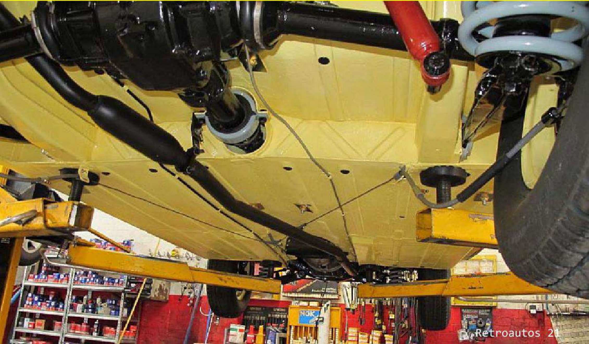
Above: The Combi sports distinctive red and white upholstery. Below: The unusual enclosed drive shaft of Borgwards is very evident here, along with the swing rear axles.
