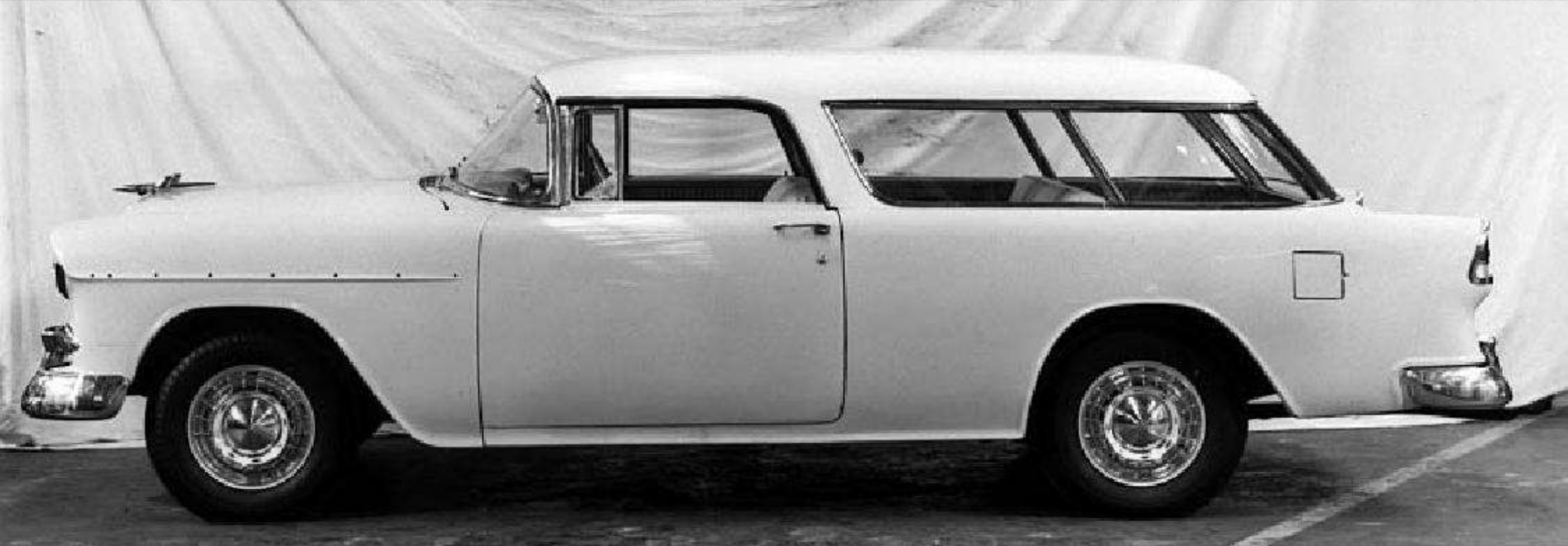
Top: This 3 rd November, 1954 image still has the rear wheel cut outs similar to the standard wagon. The slanted "B" pillar has more rake and curvature to it than the production version. Above: The first production Nomad, minus the front mudguard chrome trim. Below: The Bel Air wagon, Chevrolet sold 24,313 of them in 1955, compared to 8346 Nomads.
