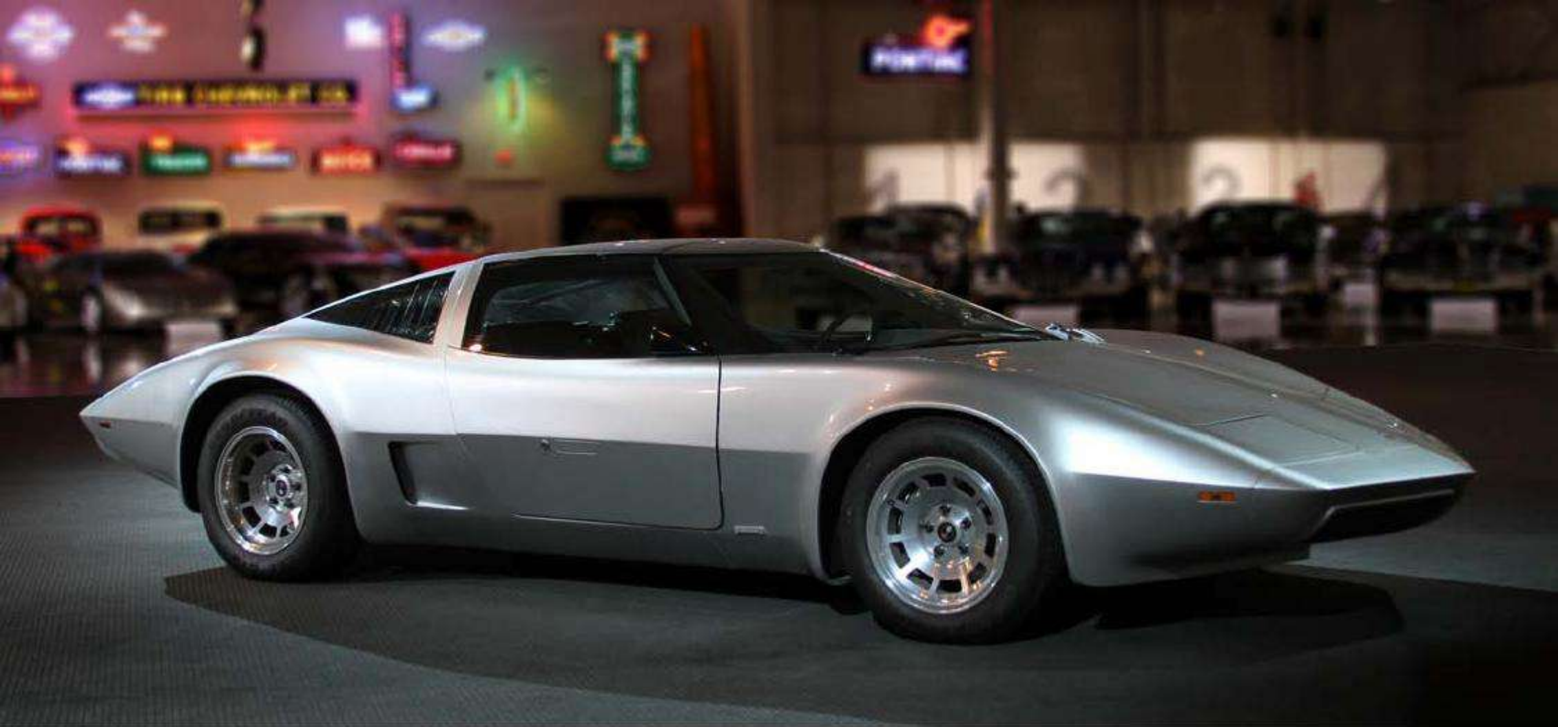
The 1973 Chevrolet Corvette Aerovette. Built to accommodate a rotary engine mid-ship, it now has a V8 behind the seats. The car's V shaped windscreen owes much to Vauxhall's XVR.
