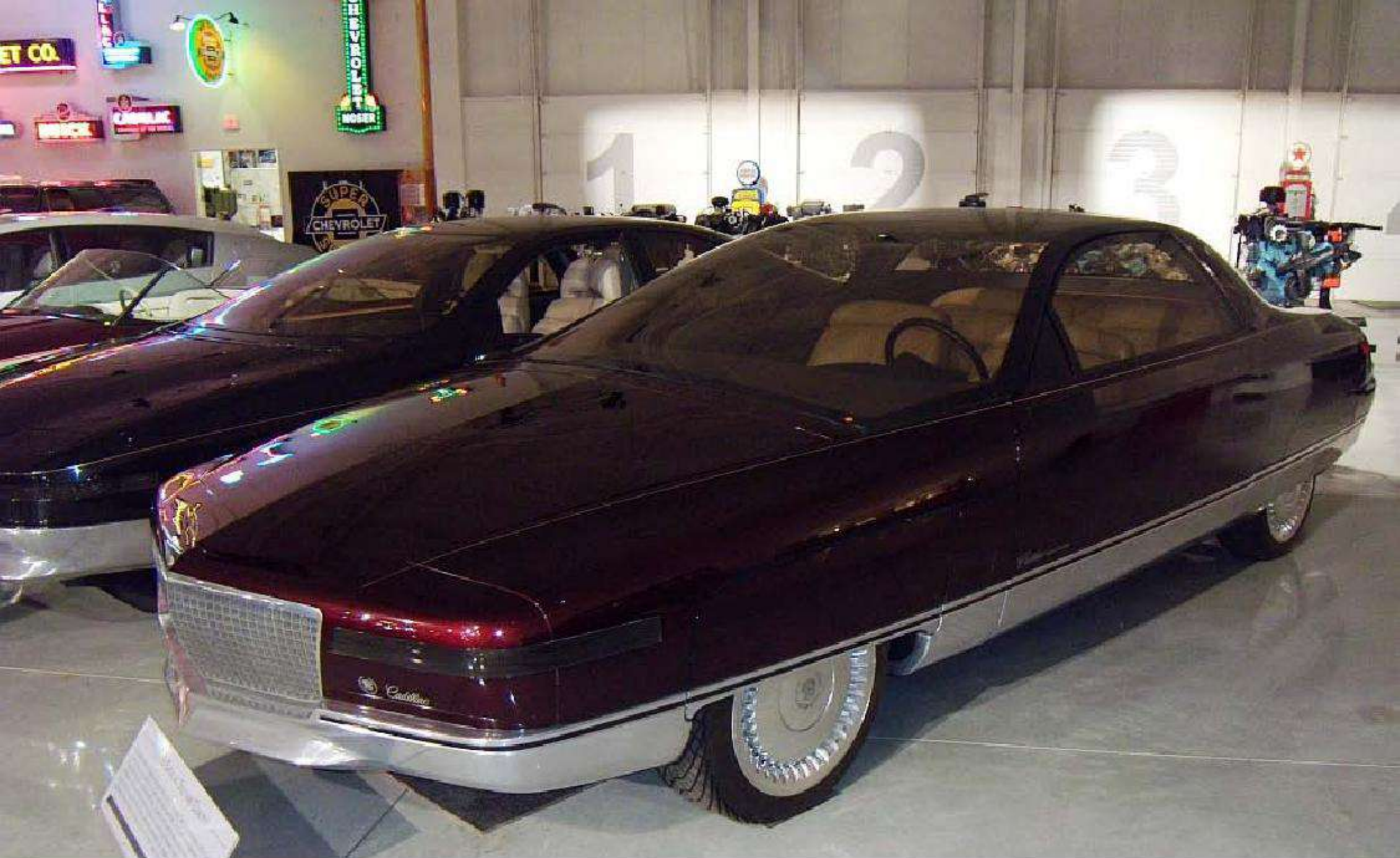
The 1989 Cadillac Solitaire concept has a .28 co-efficient of drag. Power is from a 60-degree, 48-valve, dual overhead camshaft, V12. The Solitaire features include electrically-powered articulating doors. Two miniature video cameras take the place of rear view mirrors.
