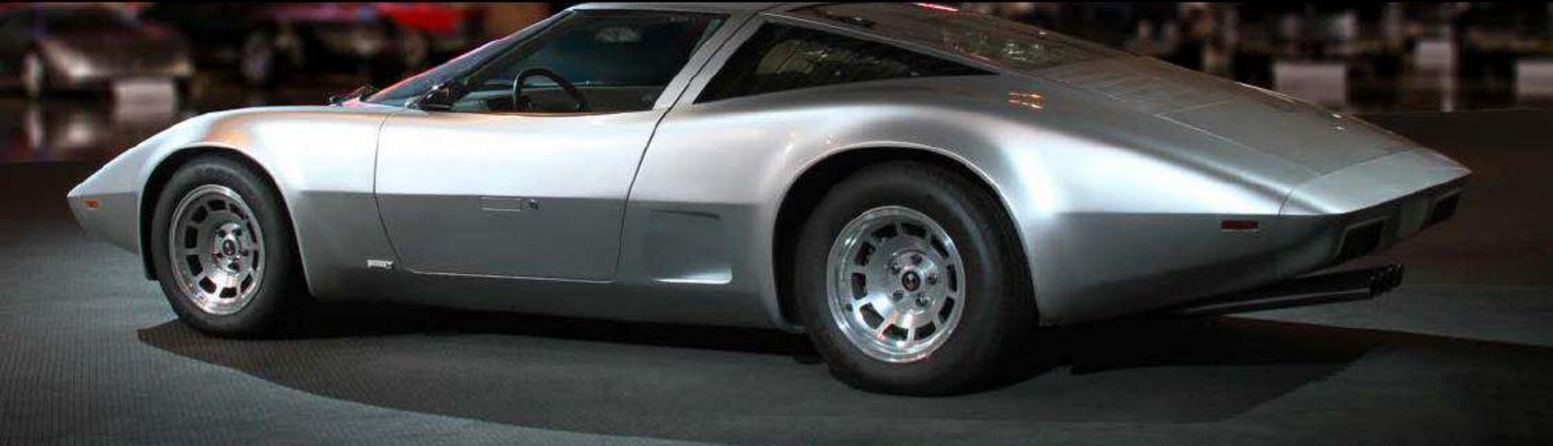
The 1973 Chevrolet Corvette Aerovette. Built to accommodate a rotary engine mid-ship, it now has a V8 behind the seats. The car's V shaped windscreen owes much to Vauxhall's XVR.
