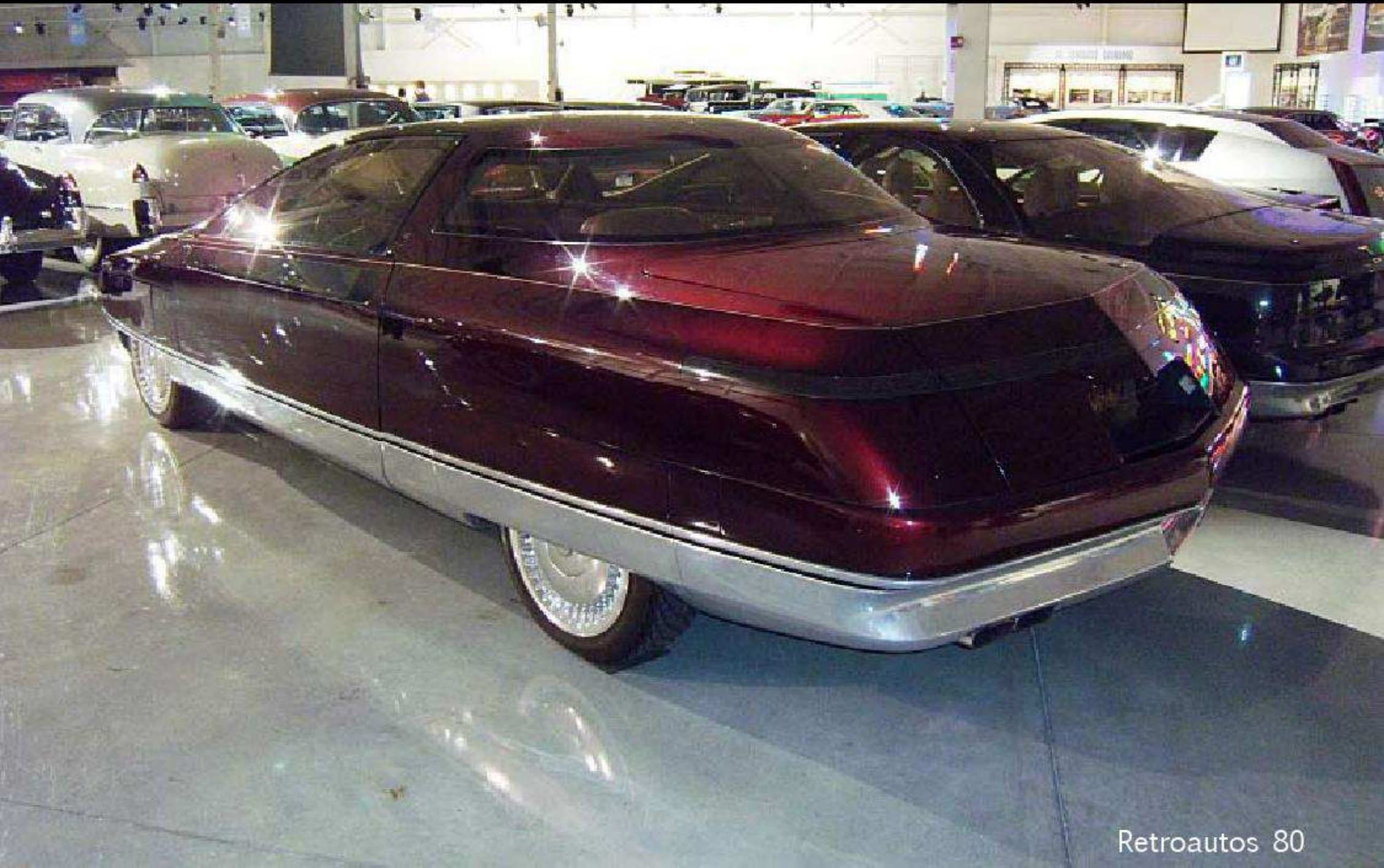
The 1989 Cadillac Solitaire concept has a .28 co-efficient of drag. Power is from a 60-degree, 48-valve, dual overhead camshaft, V12. The Solitaire features include electrically-powered articulating doors. Two miniature video cameras take the place of rear view mirrors.
