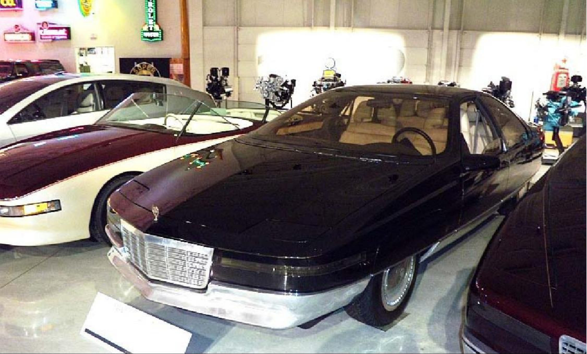
1988 Cadillac Voyage. The idea here is a big, luxury highway four door “coupe”, similar to a Mercedes CLS . It had an early version of computer controlled allocation of power to front and rear wheels, depending on the type of road surface and traction conditions.
