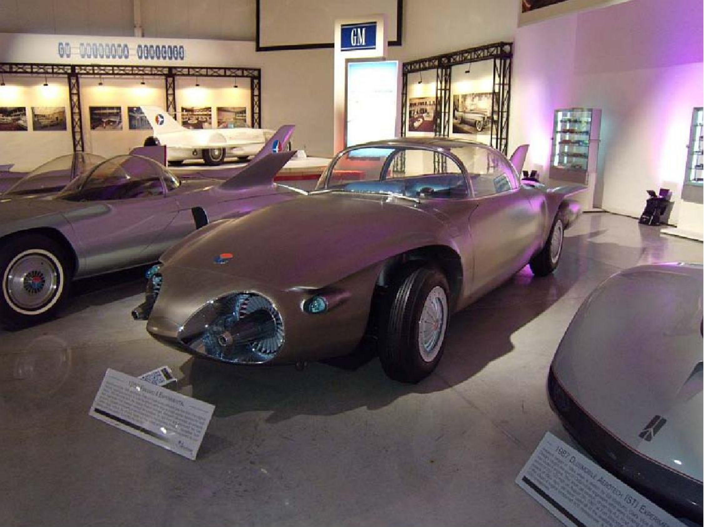
1956 Firebird II. This is a four seater, and drivable. Gas turbine powered, it has four wheel disc brakes. The body is made out of titanium, which proved hard to shape and work with.
