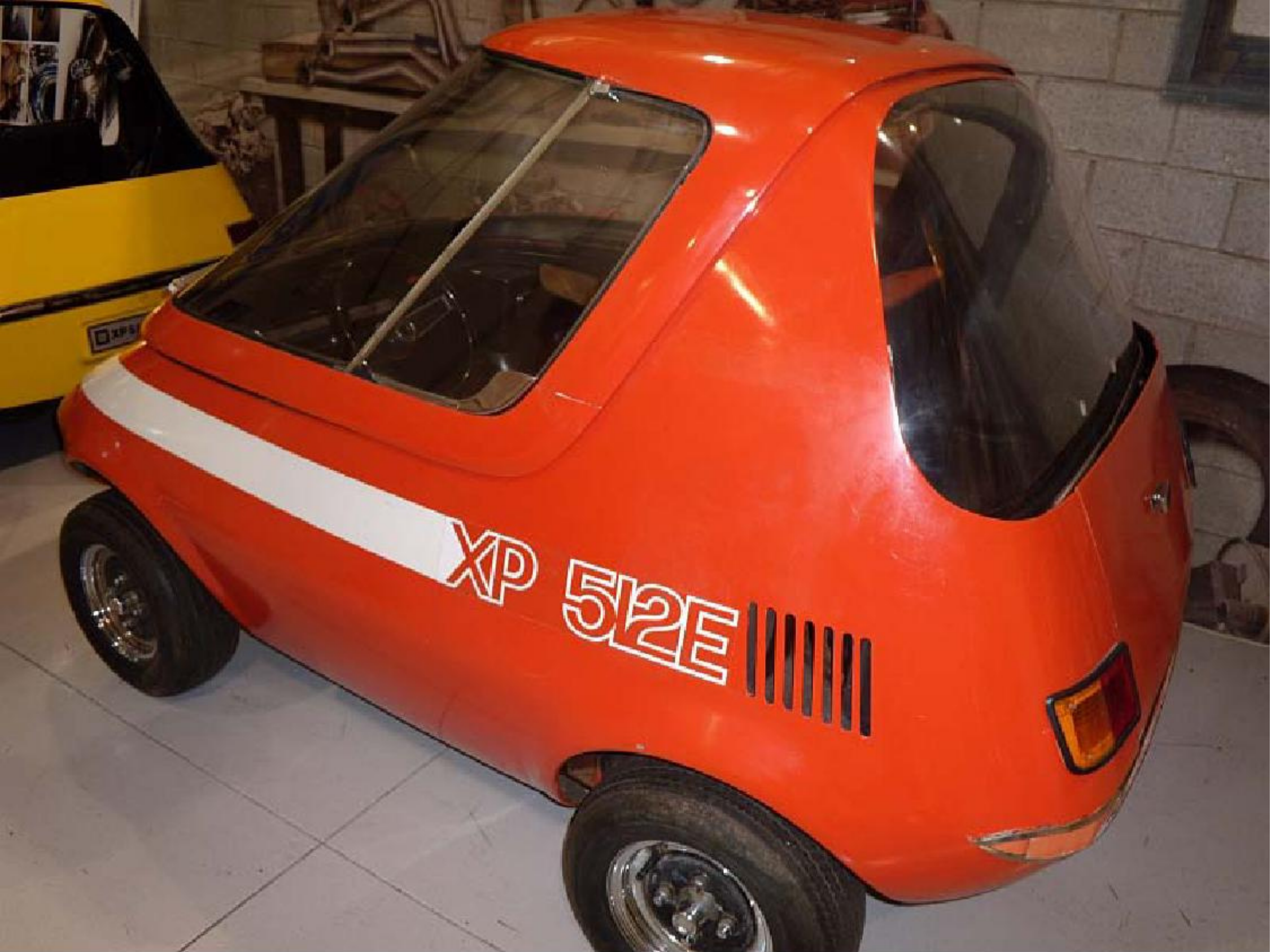
Above: More behind the scenes. This is an experimental electric powered city car GM built in 1969. It was one of three small “ideas” cars, the other two were petrol powered. Below: 1987 Buick GNX. One of the wildest muscle cars ever built, and a much sort after now.
