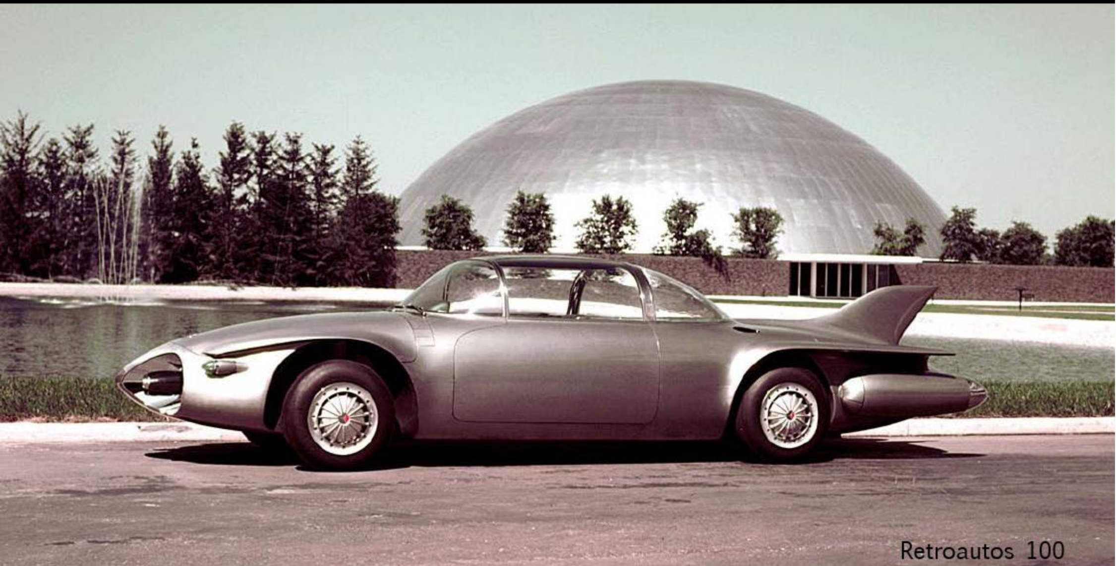
1956 Firebird II. This is a four seater, and drivable. Gas turbine powered, it has four wheel disc brakes. The body is made out of titanium, which proved hard to shape and work with.
