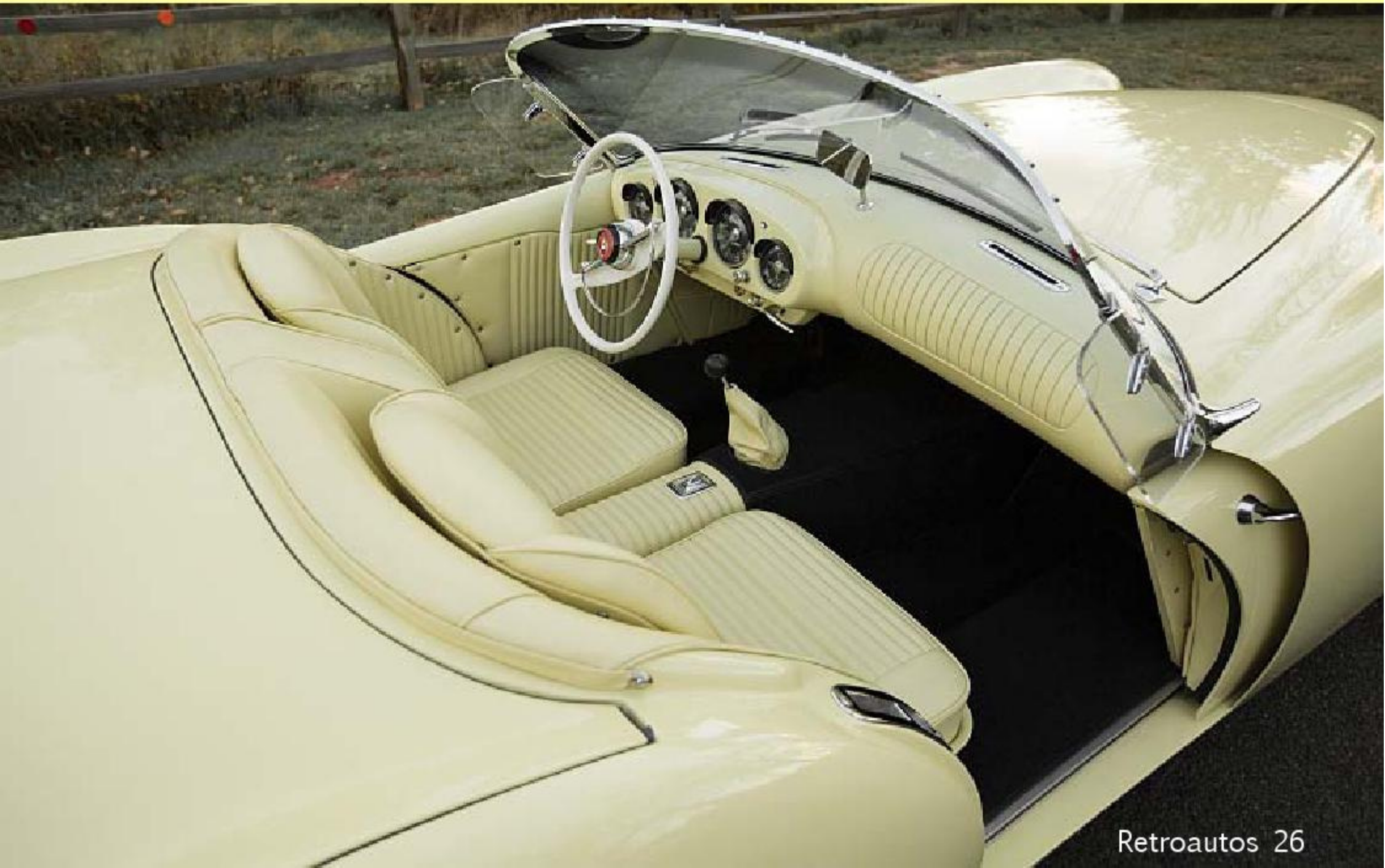
1954 Kaiser Darin. Made by Kaiser Frazer to cash in on the expanding sports/luxury market in the USA. The doors slid forward into the front mudguards. One of only 635 made. Image: RM Auctions.
