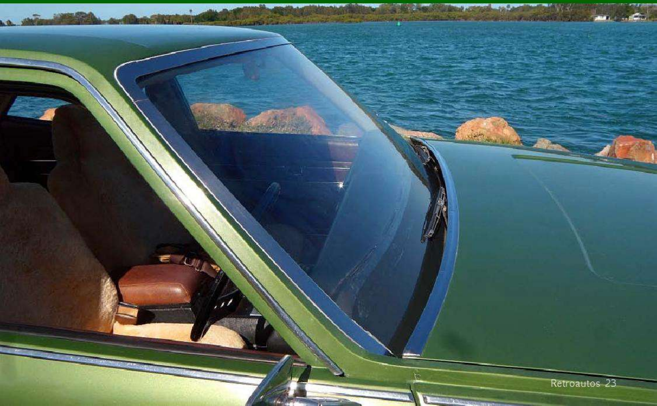
Above: The Targa Florio featured the highest level of interior appointments. Below: New for Australian built cars were hidden wipers and a glued-in windscreen.
