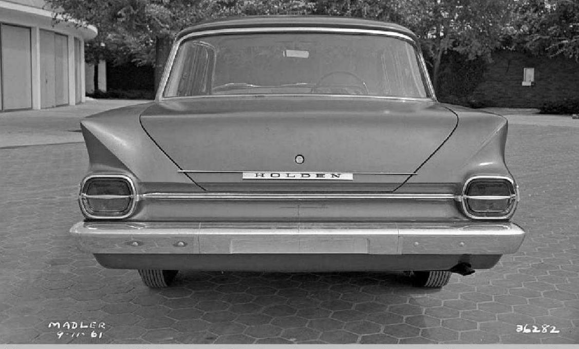
Theses images, dated 9<sup>th</sup> November 1961, show the changes made to the EJ prototype. Note how the rear mudguard shapes differ. The left side has a much sharper definition than the right side. Also evident here is the insertion of valance panels under the bumper bars, front and rear.
