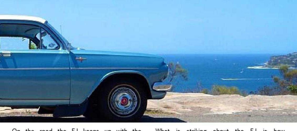
On the road the EJ keeps up with the traffic flow. "It is not as responsive as a modern car. The Hydramatic transmission sucks power out of the motor and it has drum brakes which mean longer stopping distance, so I have to think ahead of the traffic," Sam says. It lopes along nicely and the bucket seats do a great job of soaking up the bumps the suspension ignores.
