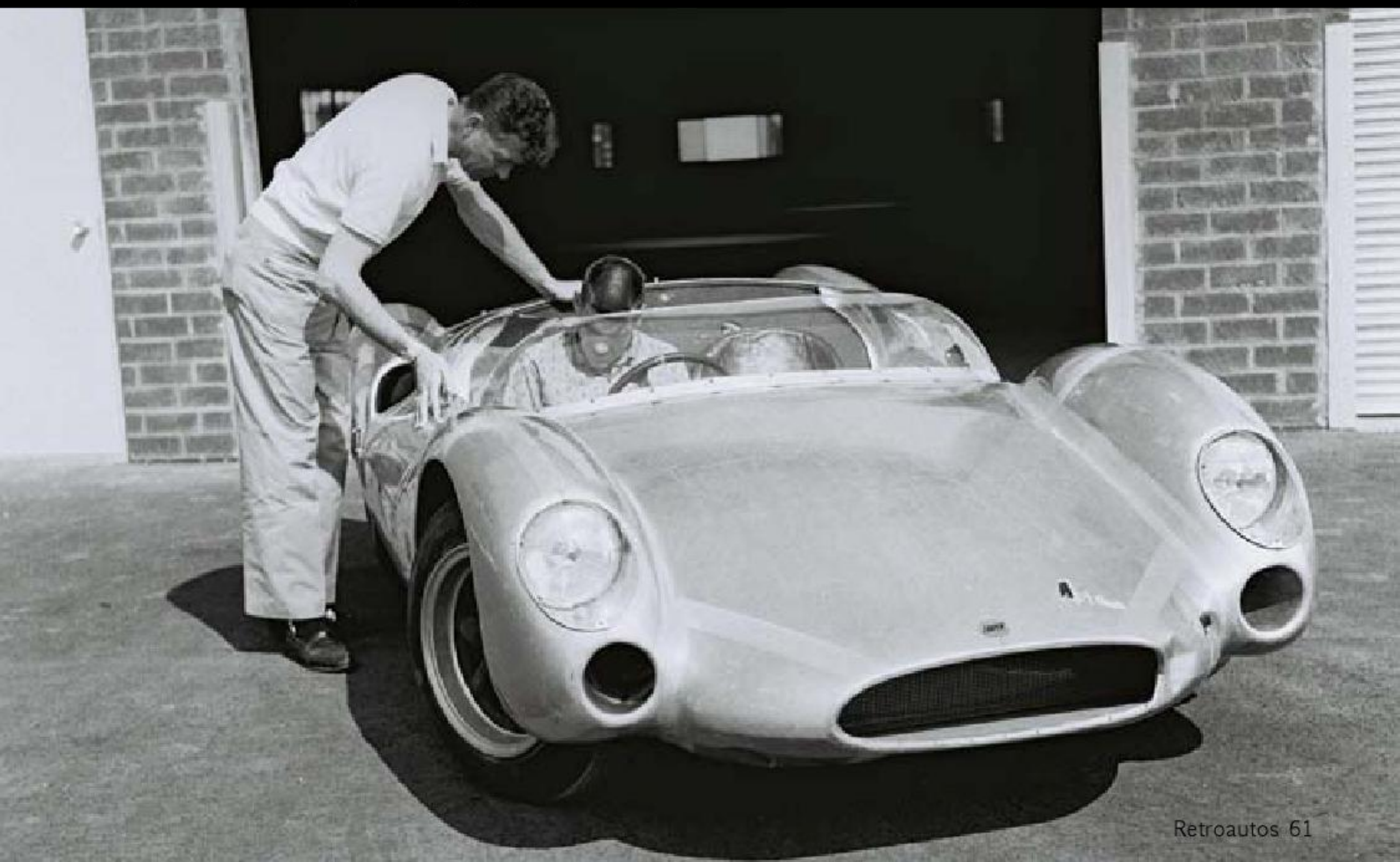
Above and below: Two previously unseen images of Carroll Shelby and Dave MacDonald trying out the newly built King Cobra before the Phoenix event. It was a rear engine Ford V8 powered car and derived from a Cooper design.
