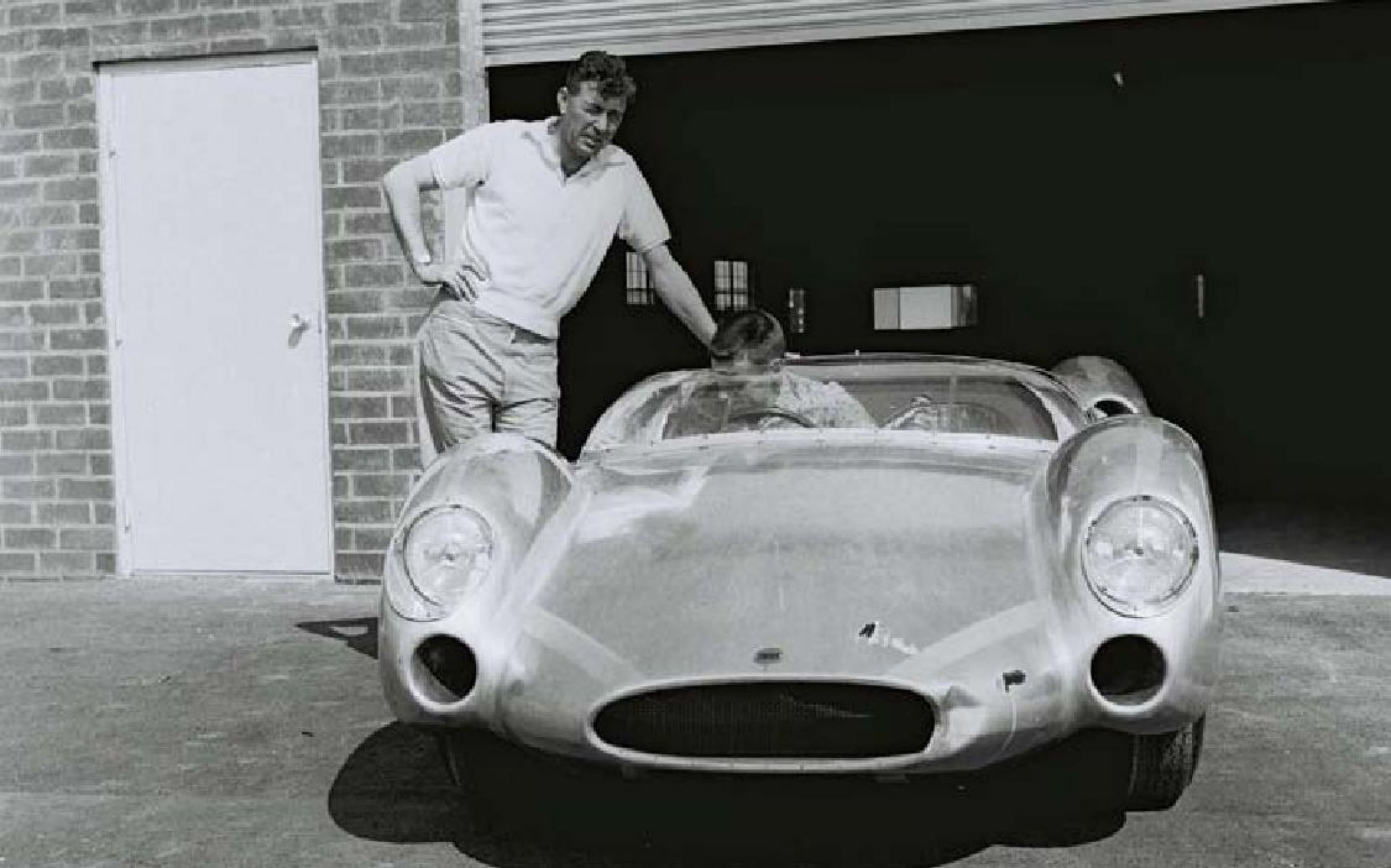
Above and below: Two previously unseen images of Carroll Shelby and Dave MacDonald trying out the newly built King Cobra before the Phoenix event. It was a rear engine Ford V8 powered car and derived from a Cooper design.
