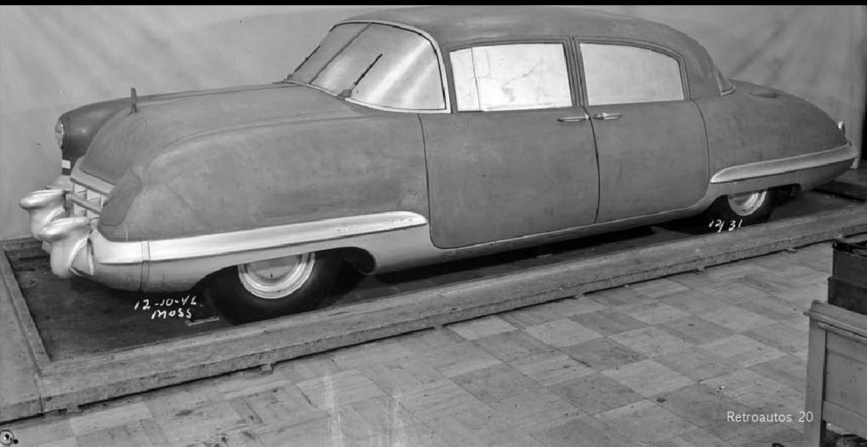
Above and below: Two ideas for the Interceptor/CO in October 1946. The right side has conventional headlights while the left side has them enclosed. Note suicide rear doors.
