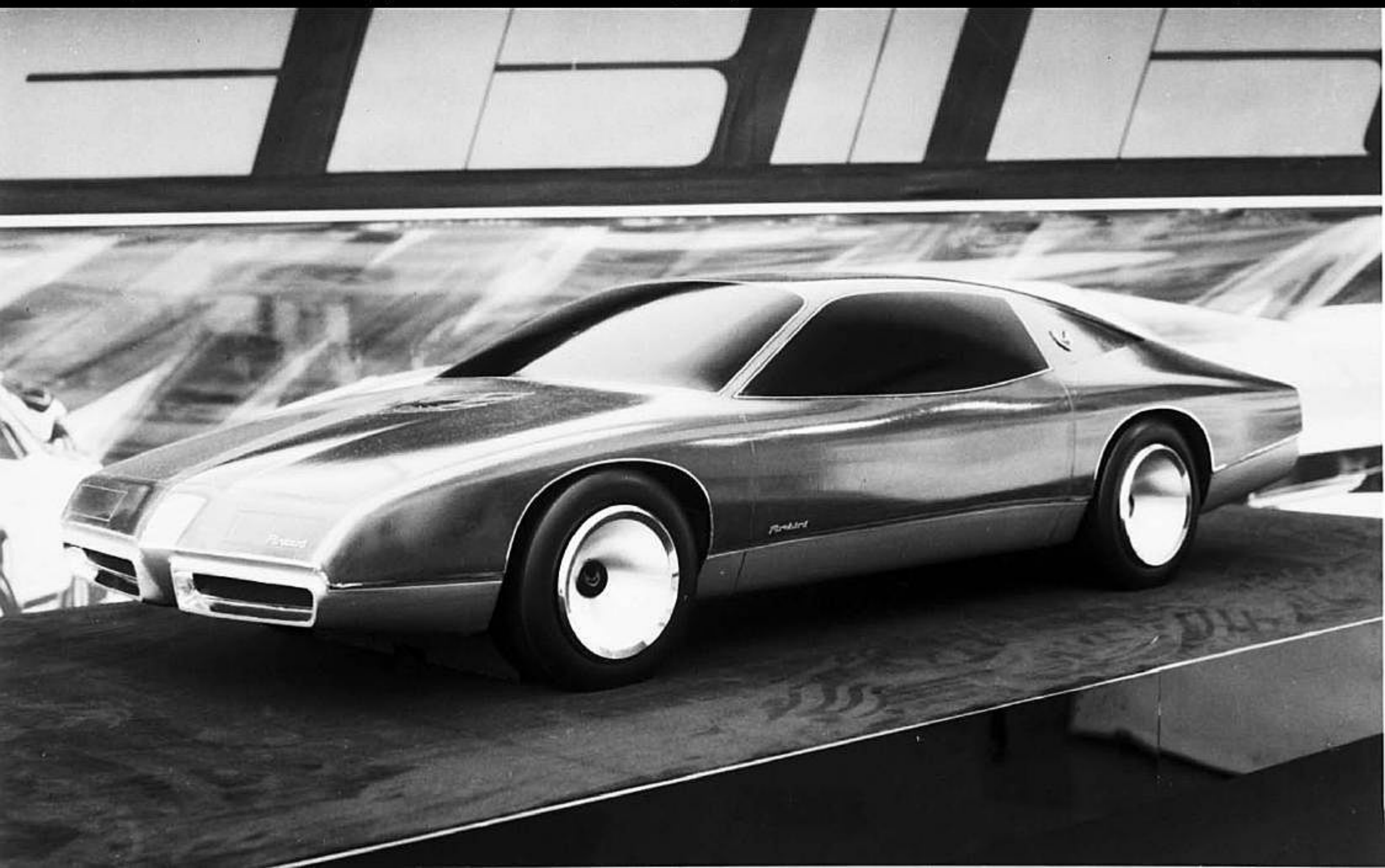
Above: A Chevrolet Camaro proposal, based on the X car platform. Below: This clay model reflects ideas for the 3 rd generation Firebird as a major facelift of the the 2 nd generation. This approach was ultimately rejected in favour of a "clean sheet" approach.
