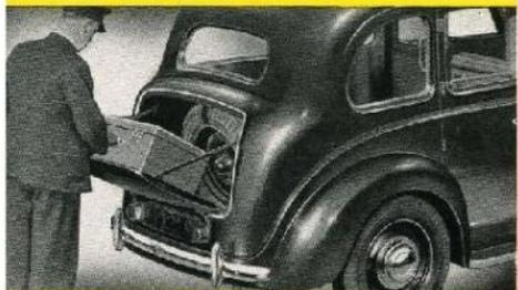
Built-in accommodation is provided at the rear of the Hire Car for the spare wheel and tyre, while the lid of the compartment can be used as a platform for luggage.
