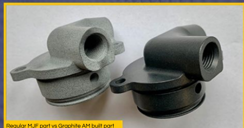
Regular MJF part vs Graphite AM built part
