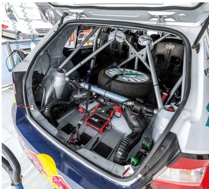
The battery pack sits in the floorpan within the footprint of the cage, its modules safely encased in a carbon fibre composite shell
