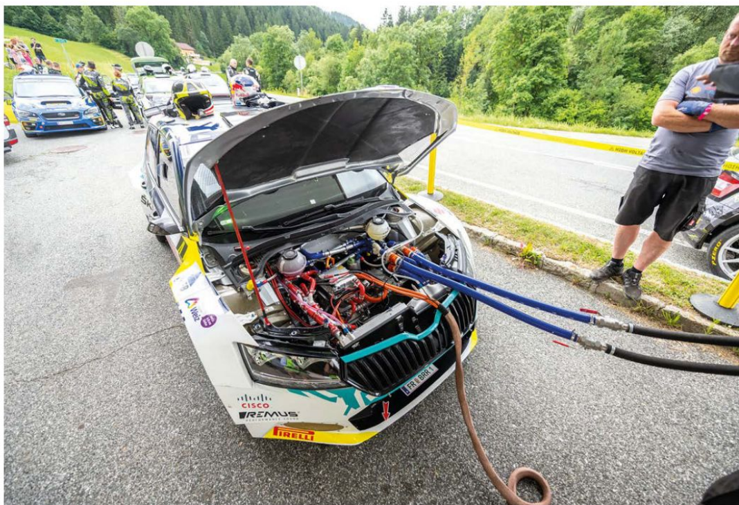
Kreisel has created a portable charging pack called Chimero, which can be easily transported to remote services where it can provide the RE-X1 with an 80 per cent charge in just 15 minutes
