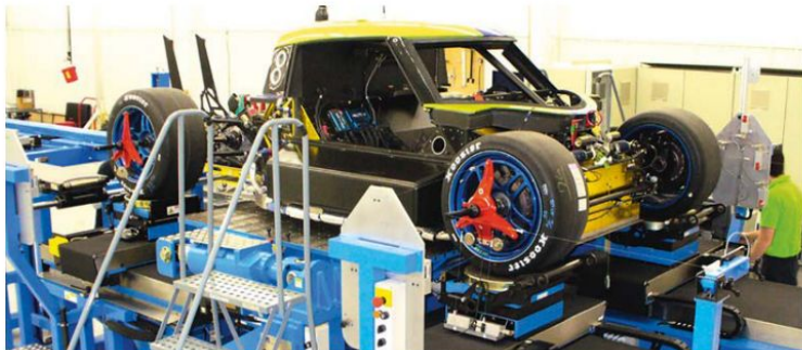
On a high-end rig the posts, which can be hydraulic or sometimes electronic rams, sit directly under the wheels of the test vehicle
