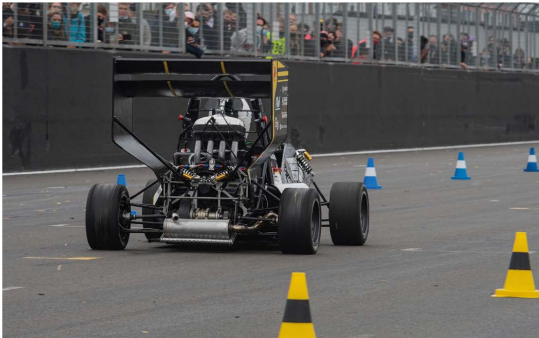
The inline 4-cylinder CBR 600 engine saw significant development to deliver more driveable torque in the optimum rev range, while the first gear was lengthened to help with the corner exits
