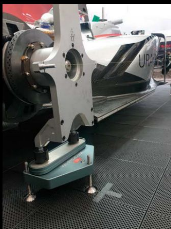
Wi-POD Intelligent Wireless Corner Weight Scales
