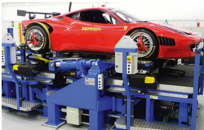
The advantage of a K&C rig over the pull-down type is that it can apply ground plane forces at the contact patches
