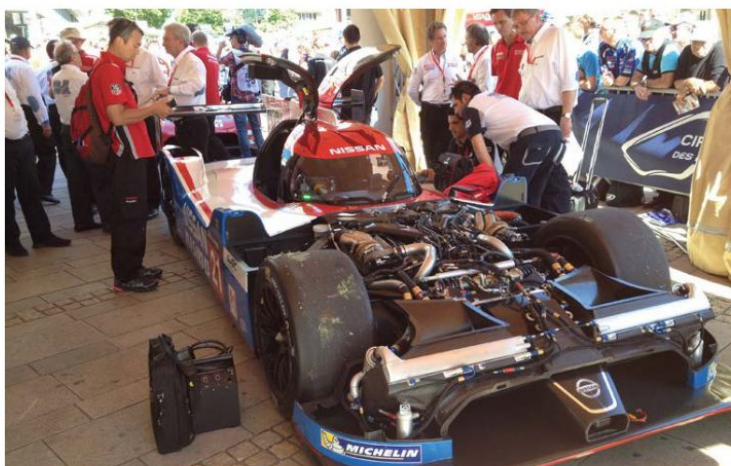
Scrutineering. Note that the radiators are part of the front splitter assembly; this caused big problems in the pits during the race
