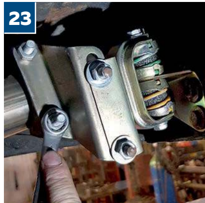
With the stainless pipework back where it belongs, Sean adjusted each mount to ensure a perfect fit and finish
