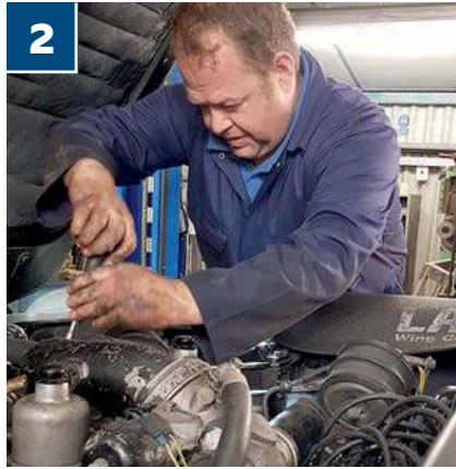
2 Non-related parts, including intake components, needed to be removed to allow access to the top of the outside exhaust manifold
