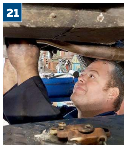
21 It was finally time to reinstall and fine-tune the Servicentre stainless steel exhaust system, safe in the knowledge that any disruption to gas flow (and any consequent loss of power) was a thing of the past
