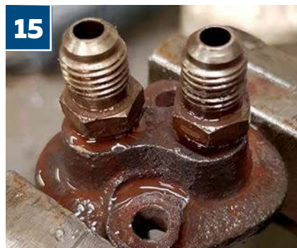
15 With the old nearside manifold rendered scrap, the heat exchanger took its place in Matt's vice, before he proceeded to clean the part in advance of its installation in the new manifold
