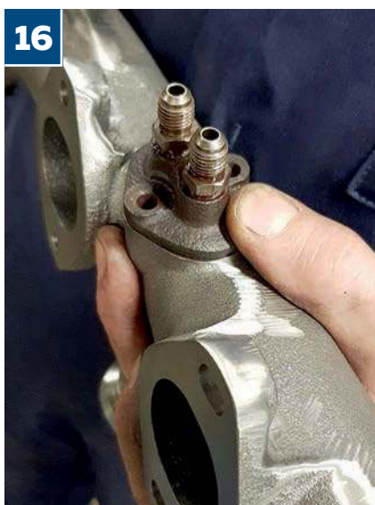
16 A snug fit for the heat exchanger in the shiny new nearside manifold!
