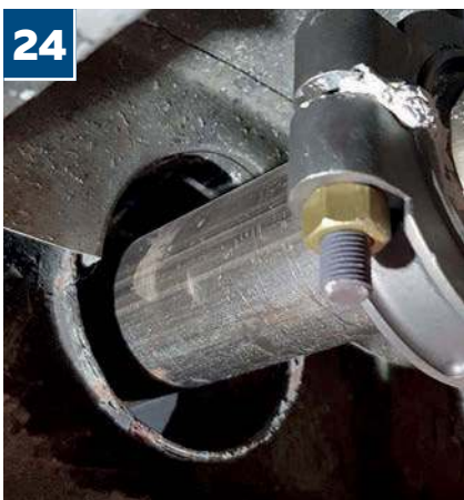
Get this part of the process wrong and you may find the height set by the mounts causes pipework to hit the chassis over bumps or when the engine is delivering heavy torque
