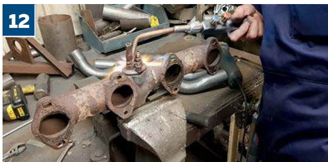
12 When working with old cars, things are never straightforward - which is why Matt brought out the big guns in order to apply heat to the heat exchanger to ensure its removal
