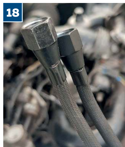
18 The heat exchanger is linked to the intake and choke assembly by two braided stove pipes, with these IntroCar items being pre-moulded to ensure a perfect fit, and bent using original factory equipment
