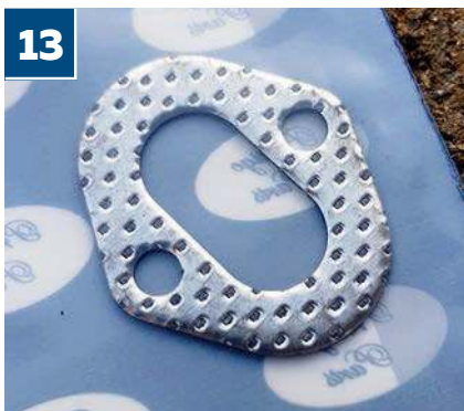
13 A removed heat exchanger requires a new gasket for installation on a new manifold (or reinstallation on a repaired manifold), and once again IntroCar was on hand to help
