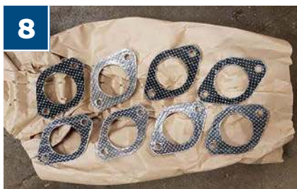
8 A fresh selection of new gaskets to accompany the new exhaust manifolds
