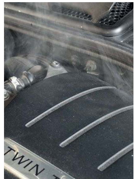
Smoke rising from the rear of the engine bay shows where the vacuum leak is
