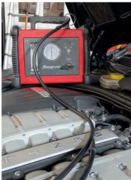
Stewart's Snap-On smoke tester is an expensive but invaluable piece of kit
