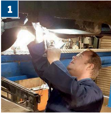
1 With the Servicentre stainless exhaust system's downpipes removed, Sean started the arduous task of freeing the old manifold bolts
