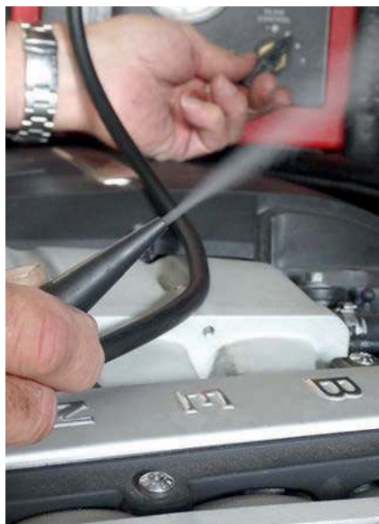
The smoke tester allows Stewart to accurately locate faults in the vacuum system
