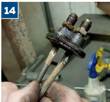
14 Ever wondered what the heat exchanger in your Silver Shadow II's nearside exhaust manifold looks like? Wonder no more!
