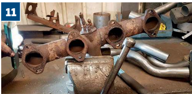
11 With the compromised nearside manifold removed, it could be placed in a vice for the extraction of its heat exchanger, which could then be fitted to the new manifold
