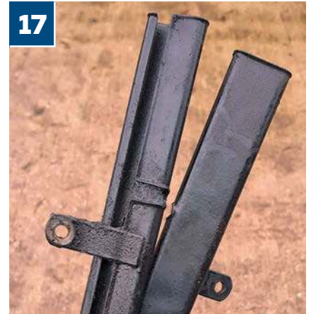
17 With the old ignition leads pulled clear, it was time to clean the tube assemblies in advance of them being united with the new set of IntroCar leads
