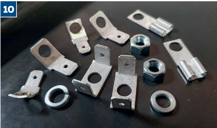
Here are the terminal connectors supplied with the IntroCar ignition coil...
