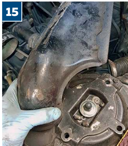
You also need to remove the hot air duct for the air cleaner, freeing the part from its position above the offside exhaust manifold
