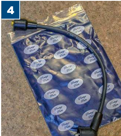
4 If buying a new set of ignition leads, check whether or not the kit you're investing in is supplied with a new king lead
