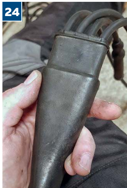
Dealing with dirt aside, perhaps the most challenging part of the job was feeding four chunky ignition leads through the very tight rubber cable support assembly
