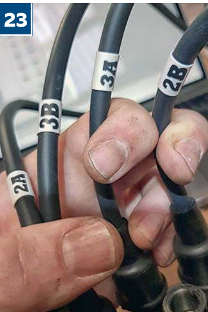
Observing the correct firing order and checking the vintage leads and distributor removed from the car, the helpfully labelled ignition leads were connected to the new cap
