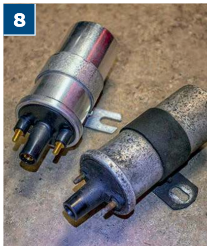
8 The new IntroCar ignition coil (left) and the old part side-by-side on the workshop floor
