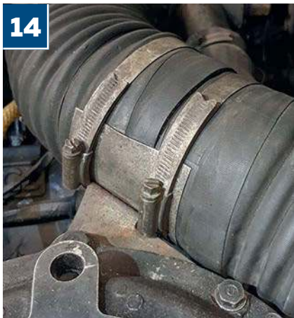
To gain access to all spark plugs on the offside bank, you'll need to remove intake pipework – a simple case of loosening jubilee clips and pulling hoses to one side
