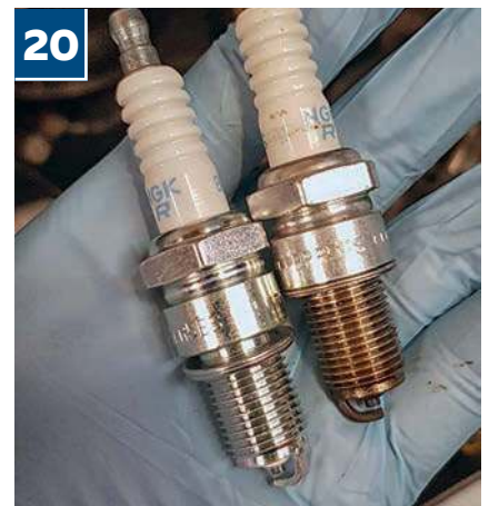
20 New and old spark plugs alongside one another; the colour of the used plug is to be expected after a long overdue tune-up following years of lack of use
