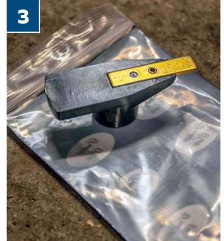
3 Rotor arms are a thorn in the side of many owners of classic cars, but replacing this oft-failed part is a quick, easy and cheap process
