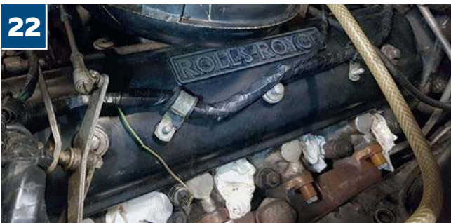
It won't win the car any concours competitions, but a wipe around in the engine bay removed most of the grime the new parts were otherwise likely to come into contact with
