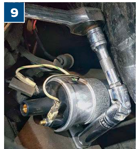
9 A universal joint on the end of a ratchet extension will assist with removal and installation of ignition coil mount bolts
