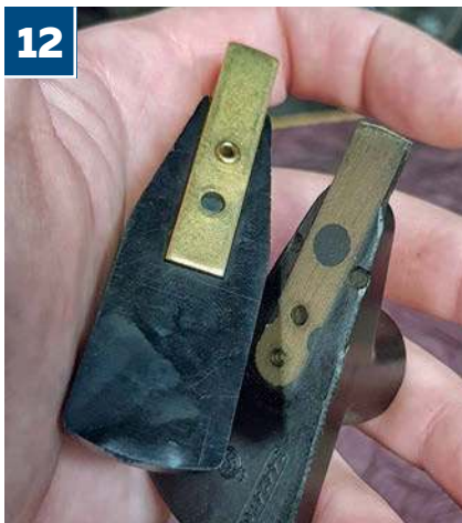
With the distributor cap unclipped and pulled to one side, the old rotor arm (right) could be removed and replaced with the new part (left)
