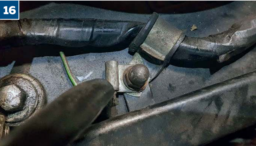
16 Earth straps are fastened to the rocker cover on each side of the engine, occupying the same spot as the rear mounting point for each ignition lead tube trunking
