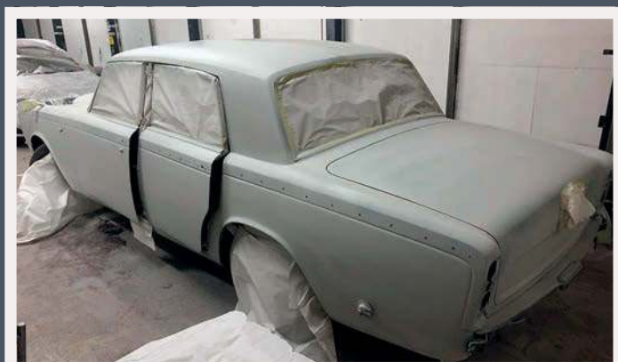
The bodyshell prepared and painted in primer, ready to receive several coats of Masons Black paint – a genuine Rolls-Royce colour
