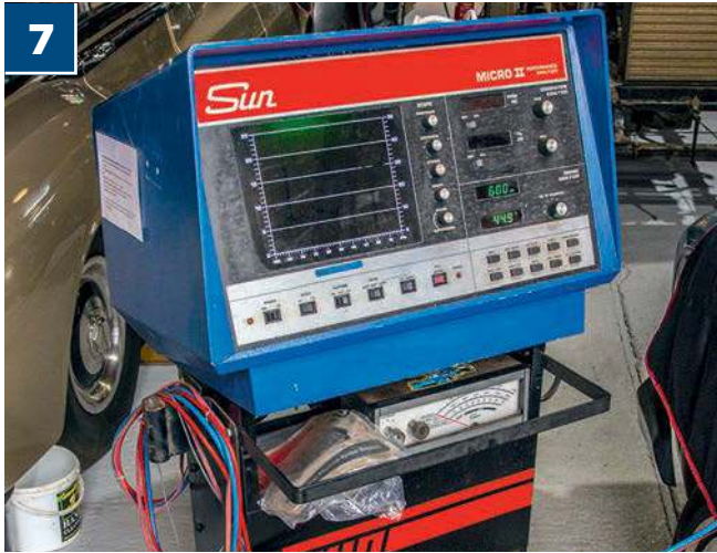
7 Time to bring out the big guns! Enter Daniel's classic Sun Micro II Performance Analyzer...
