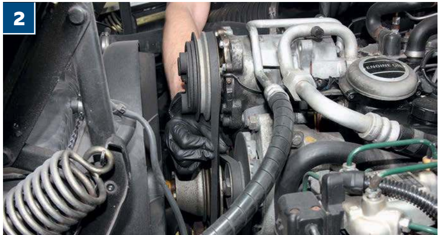
2 There are four auxiliary drive belts at the front of this engine, which drive components such as the power steering pump and alternator. Each belt should be sufficiently tight to twist it a quarter of a turn.
