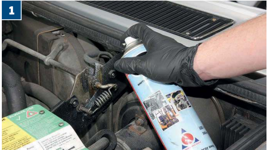
1 Spray white grease or a similar semi-thick grease over the bonnet release mechanism on each side of the engine bay to help prevent it seizing in the future.
