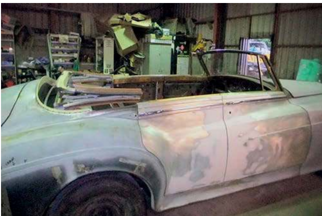
Creating a four-door convertible from a standard-wheelbase car was a challenge
