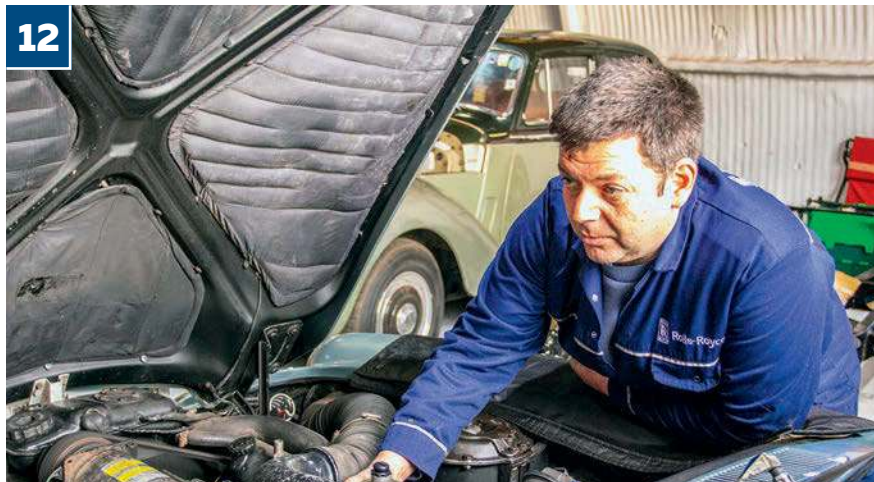
12 Daniel confirmed engine timing was as close to perfect as it could be, ruling out another possible cause for the presence of the blip under load; it was time to raise the car in the air for further scrutiny, as well as for an impromptu oil change
