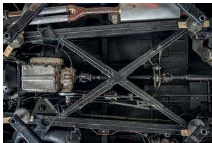
The chassis was restored, shot-blasted and repainted as part of the process
