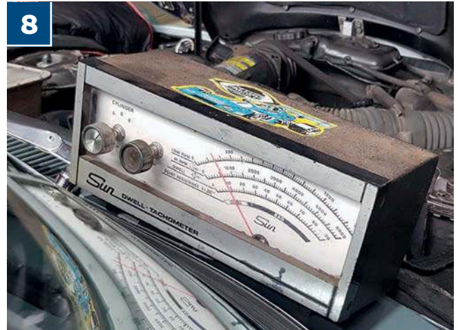
8 ...and his dinky Dwell Tachometer. Keep it steady Dan, and whatever you do, don't accidentally knock that shift lever into Drive mode, else that Twenty is going to need even more restorative work!
