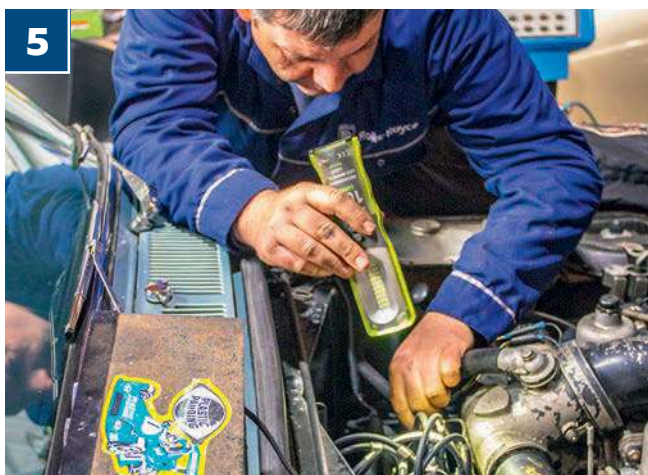
The time-served Rolls-Royce & Bentley specialist started by inspecting the new ignition components in order to rule out incorrect installation or faulty equipment
