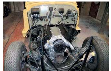
The car's engine and gearbox were stripped and rebuilt during the restoration
