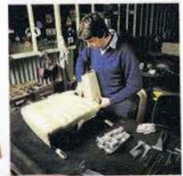
Far left. Perfectly matched holes of Connolly leather are carefully marked out and cut individually. Skilled machinists thenally sew in the shape of the seat. Every care is taken to ensure comfort and convenience. Electrically controlled mechanisms adjust the front seats in any plane at the touch of a switch. Above. Armrests are fitted to support or to fold away unobtrusively. It all adds up to a private and individual world as comfortable and practical as it is beautiful and luxurious.
