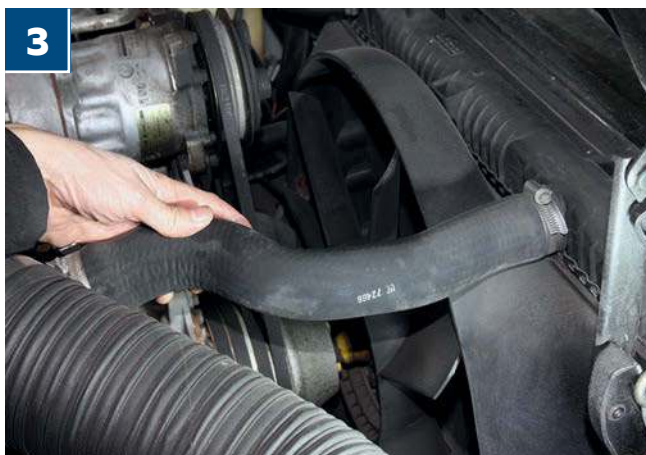
3 Rubber coolant hoses can perish during cold weather, resulting in leaks. When the engine is cold, pinch each hose to look for cracks. Check that all hose clips are secure, but avoid overtightening them, which risks cutting into the rubber.
