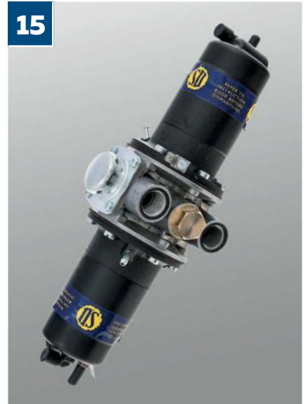
A conversation with the fuel system gurus at Burlen revealed the availability of original specification dual polarity pumps with points, as well as an updated version of the same kit using an electronic functionality
