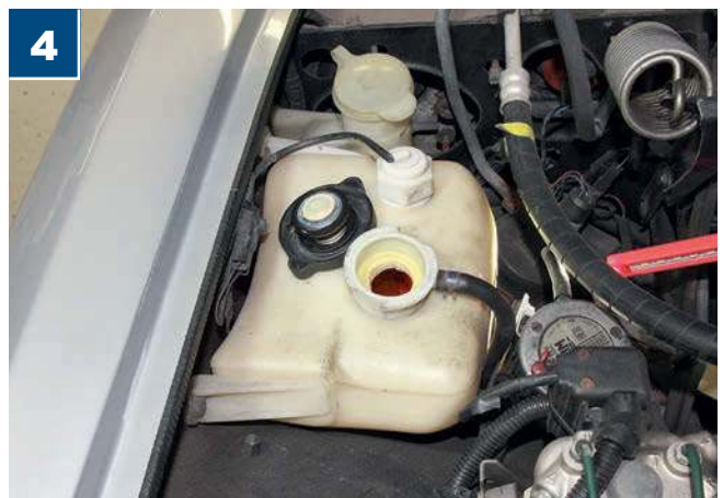
4 The coolant expansion tank is located on the nearside front of the engine bay. There are minimum and maximum markings on the side to help check the level. Top up with whatever colour of coolant has been used before.
