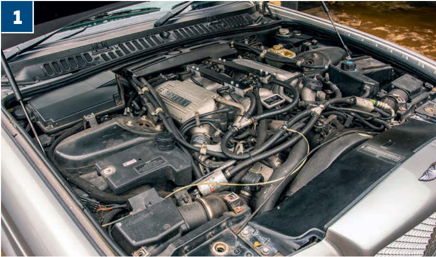
1 Removing the engine covers was necessary to access the LPG system's front-located components, including filter housings, the electronic valve protection pump and diagnostic port; the LPG injector rails can be seen positioned above the intake manifold
