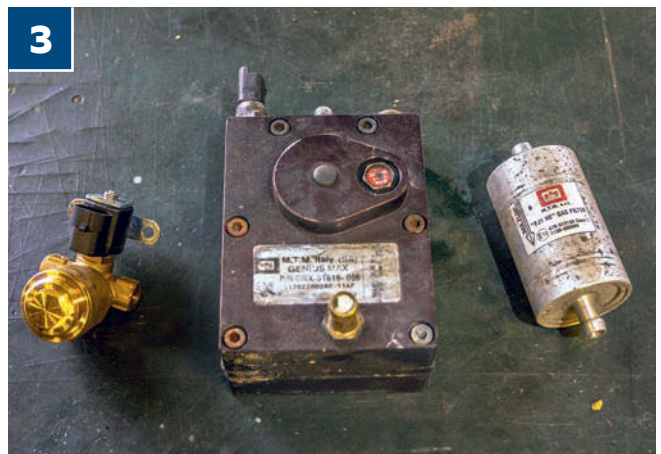
3 Tore serviced the system's vaporiser and installed a new liquid gas solenoid valve assembly
