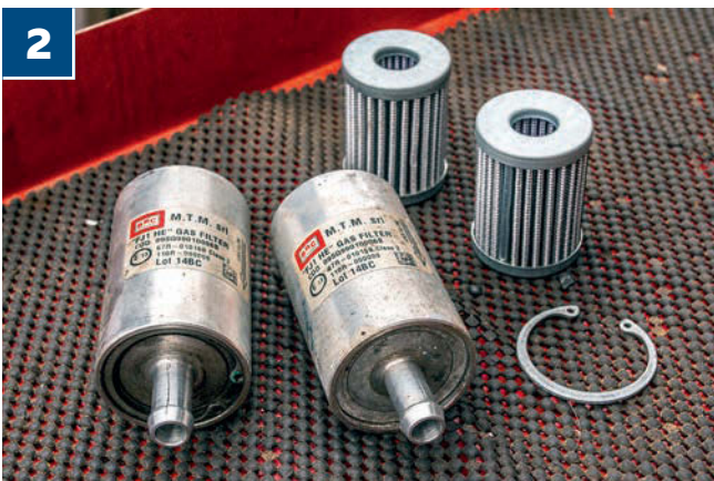
2 The system's new glassfibre filters are a direct swap for the old filters fitted inside original BRC metal housings; there's no need to ditch each complete assembly
