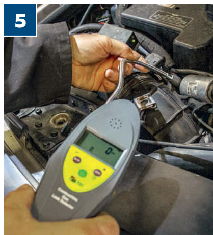
5 Tore whipped out his LPG leak detector after installing the new parts and, as expected, the results were perfect, demonstrating a system safe for continued operation
