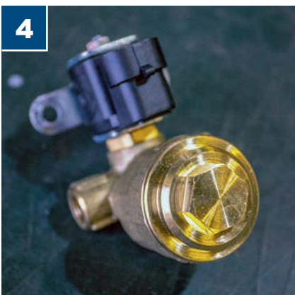
4 The liquid gas solenoid valve body houses its own filter; the assembly works with the vaporiser in a process whereby liquid gas is fed from the fuel tank in the spare wheel well and turned to vapour, subsequently sent to the system's injectors in the engine bay
