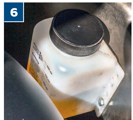
6 The reservoir containing the system's lubrication fluid is mounted in the spare wheel well, alongside the LPG tank; this unappetisingly coloured additive is sent towards the front of the car, where it passes through a small pump managed by an electronically programmable controller
