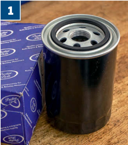
1 A new oil filter from IntroCar's Prestige Parts range was ready and waiting to replace the stuck component
