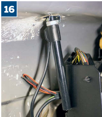
16 Much to everyone's surprise, the in-situ aerial was a manually operated mast – bent out of shape and not connected to the head unit!
