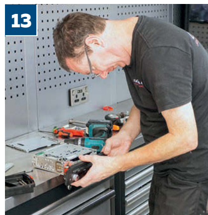
13 Gerry removed the body of the head unit from its home (hidden by a walnut panel in the dash) and proceeded to reattach the fascia as the first step to diagnosing the lack of radio reception
