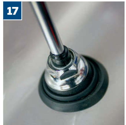
17 As a quick fix to enable immediate radio reception, Gerry replaced the duff aerial with a new manual mast until a decision is made regarding specification of the soon-to-be-revised entertainment system
