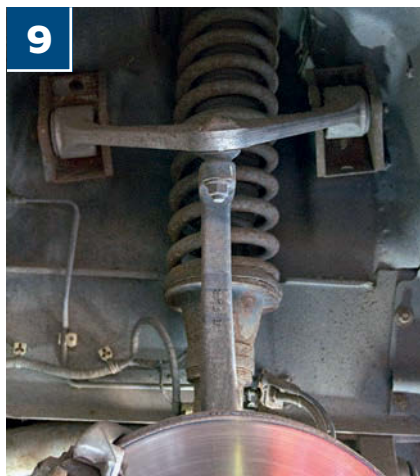
9 Next up was an examination of front-end suspension components after a knock was detected over bumps in the road
