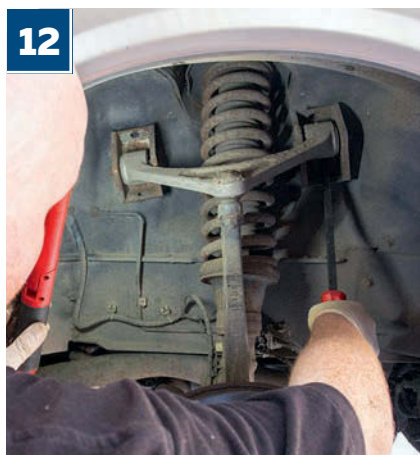
12 IntroCar offers a complete Arnage front suspension overhaul kit, featuring polyurethane upper and lower control arm bushes, all ball joints and copper grease
