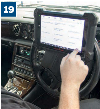
19 Before the car left London, Gary ran a diagnostic health check on the Bentley's electrical systems, searching for any recent or historic fault codes
