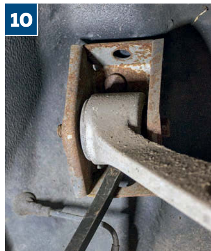
10 Gary confirmed the offside upper control arm bushes are worn, necessitating replacement
