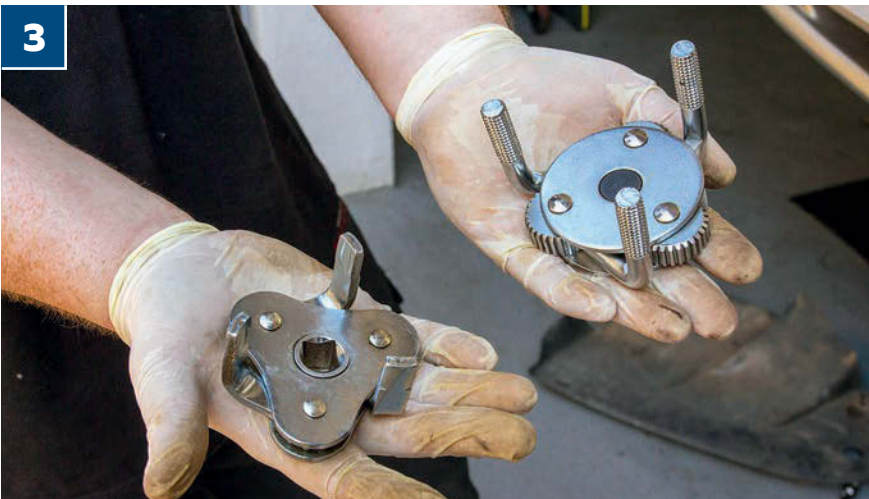
3 Gary's 'spider' oil filter removal tools are far better at shifting stuck filters than the classic chain-on-socket set-up, which can dent and bend stubborn filters
