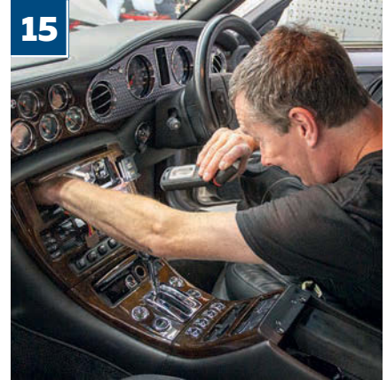
15 After reassembling the dismembered head unit, Gerry proceeded to check wiring managing and controlling the in-car entertainment system, including the suspect aerial
