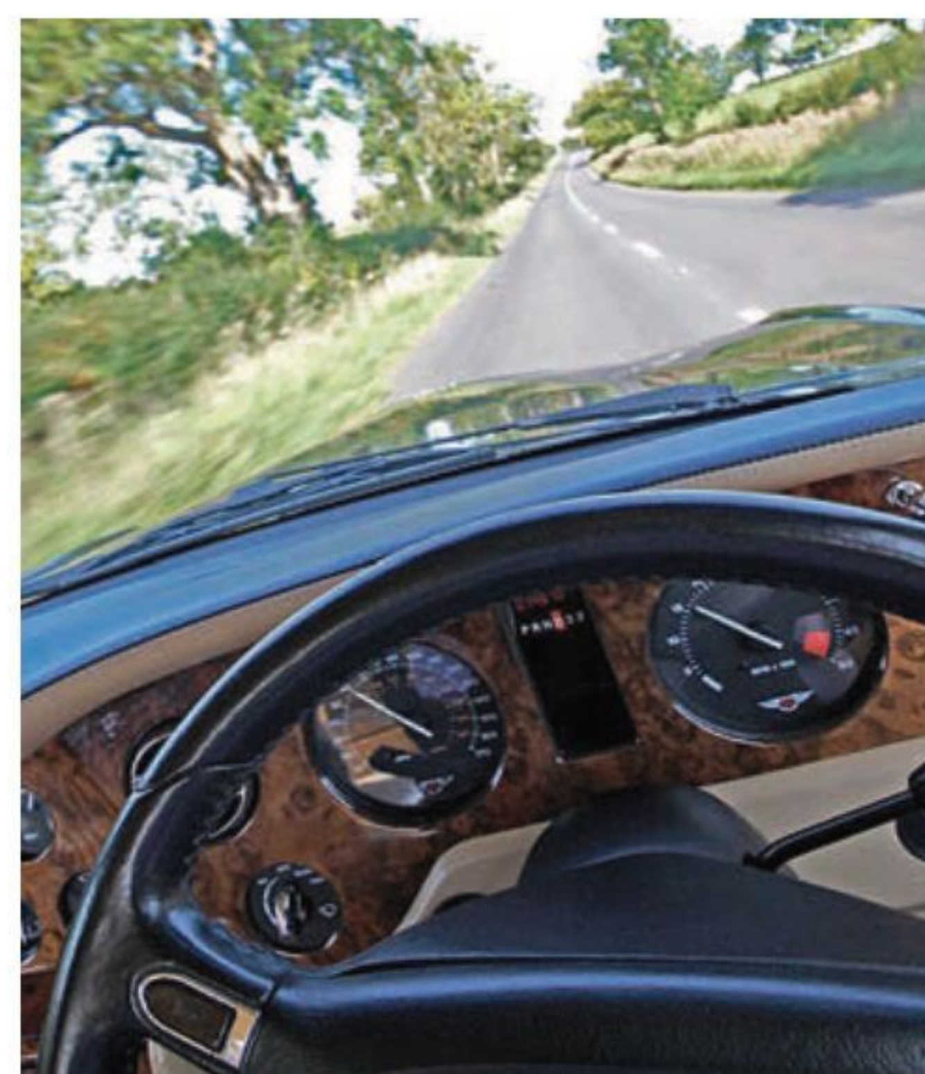
In top gear the Turbo RT does 40mph per 1000rpm, meaning the engine is barely above tickover (at 1500rpm) when travelling at 60mph
