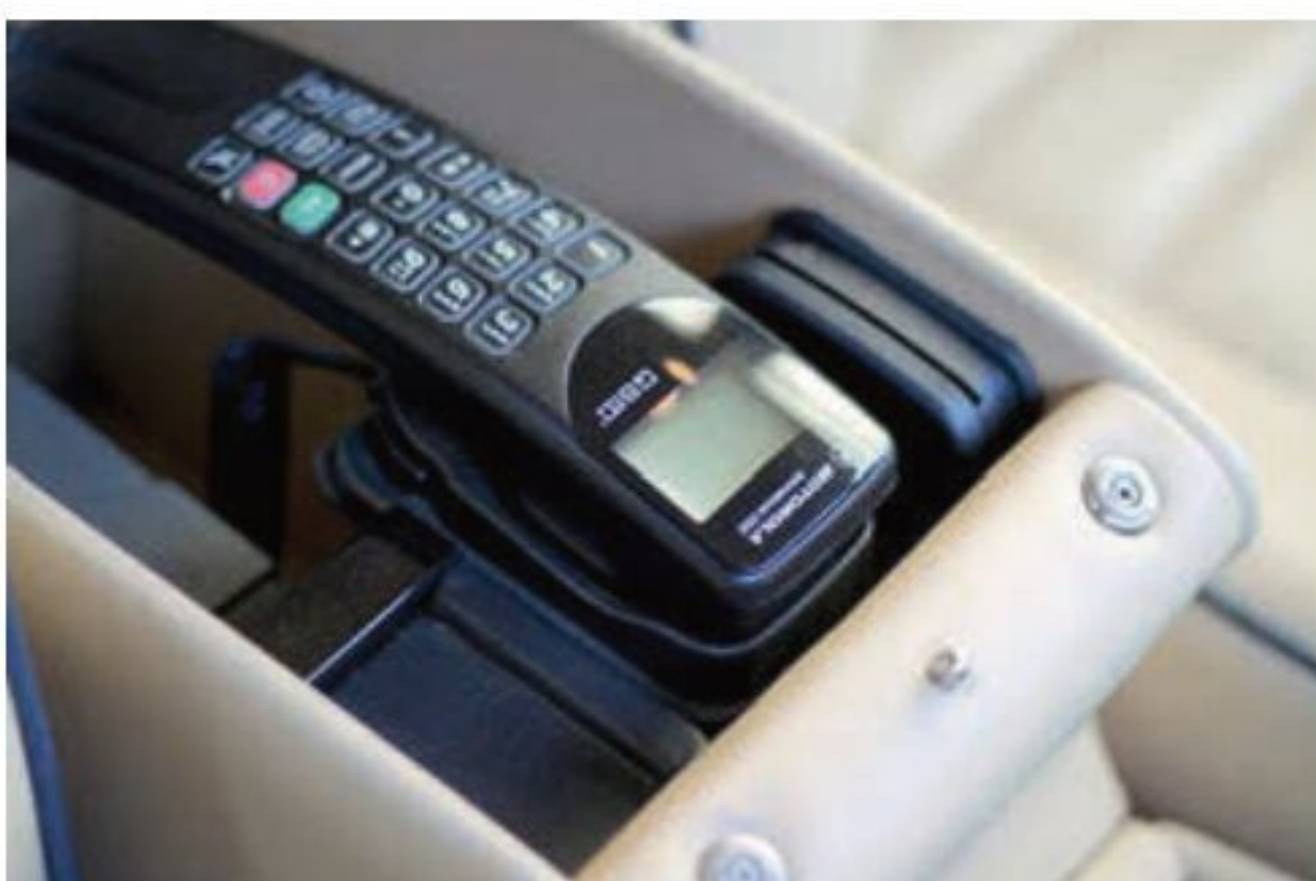
Storage compartment beneath the hinged front armrest contains the hands-free telephone and six-disc CD changer
