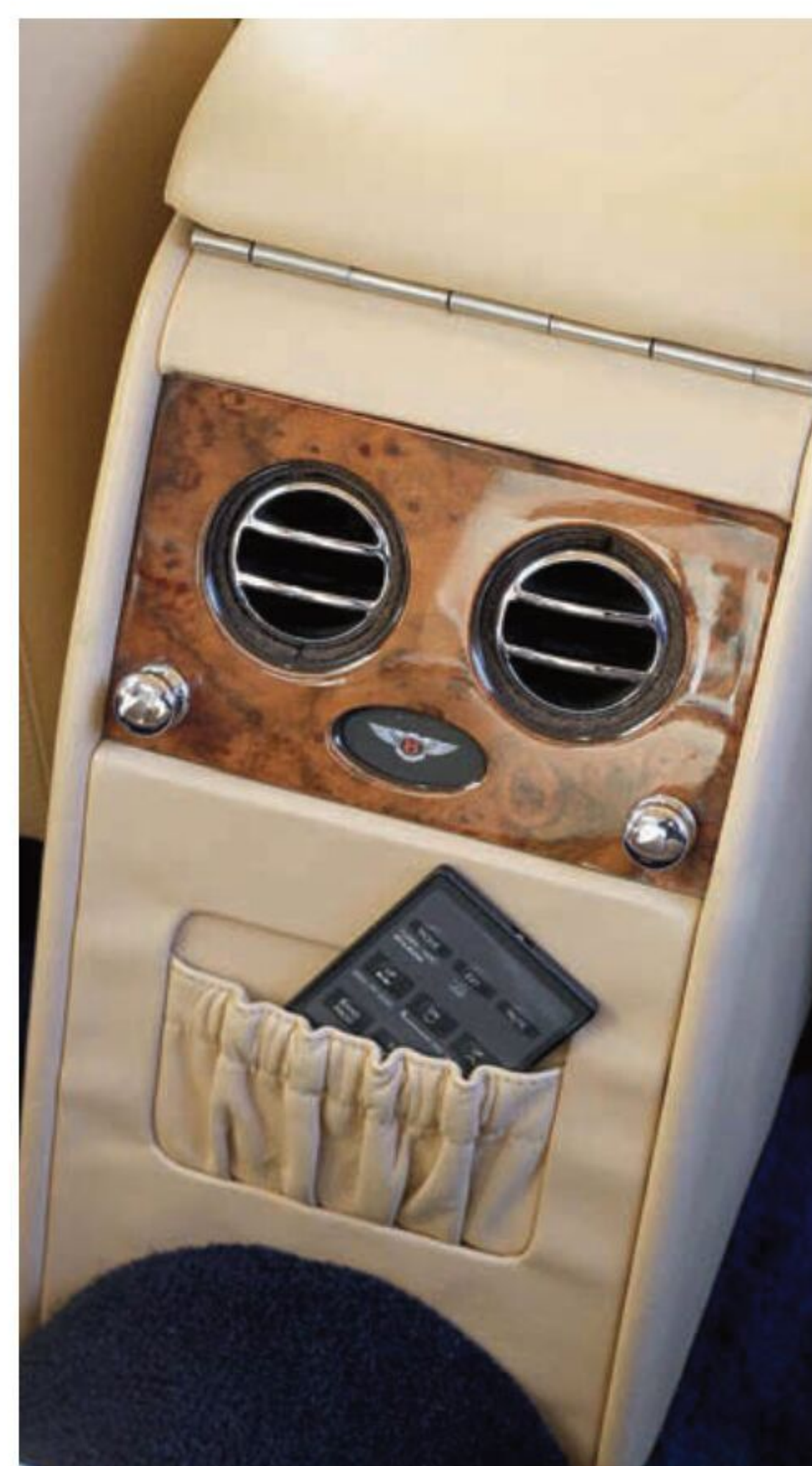
From model-year 1996, cars had individually controlled rear air vents; a credit card-sized remote controls the stereo
