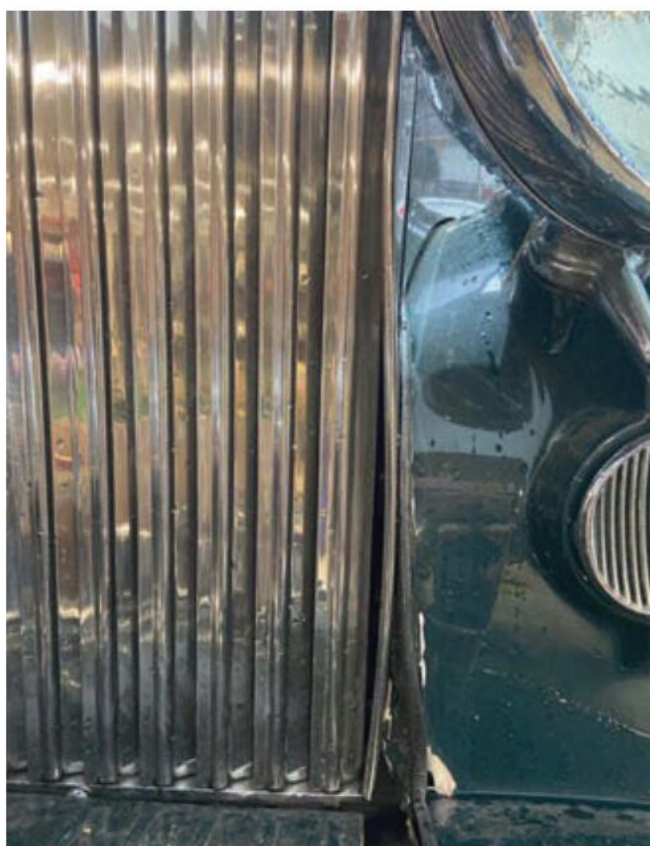
The Rolls-Royce radiator grille suffered some twisting but was persuaded back into shape
