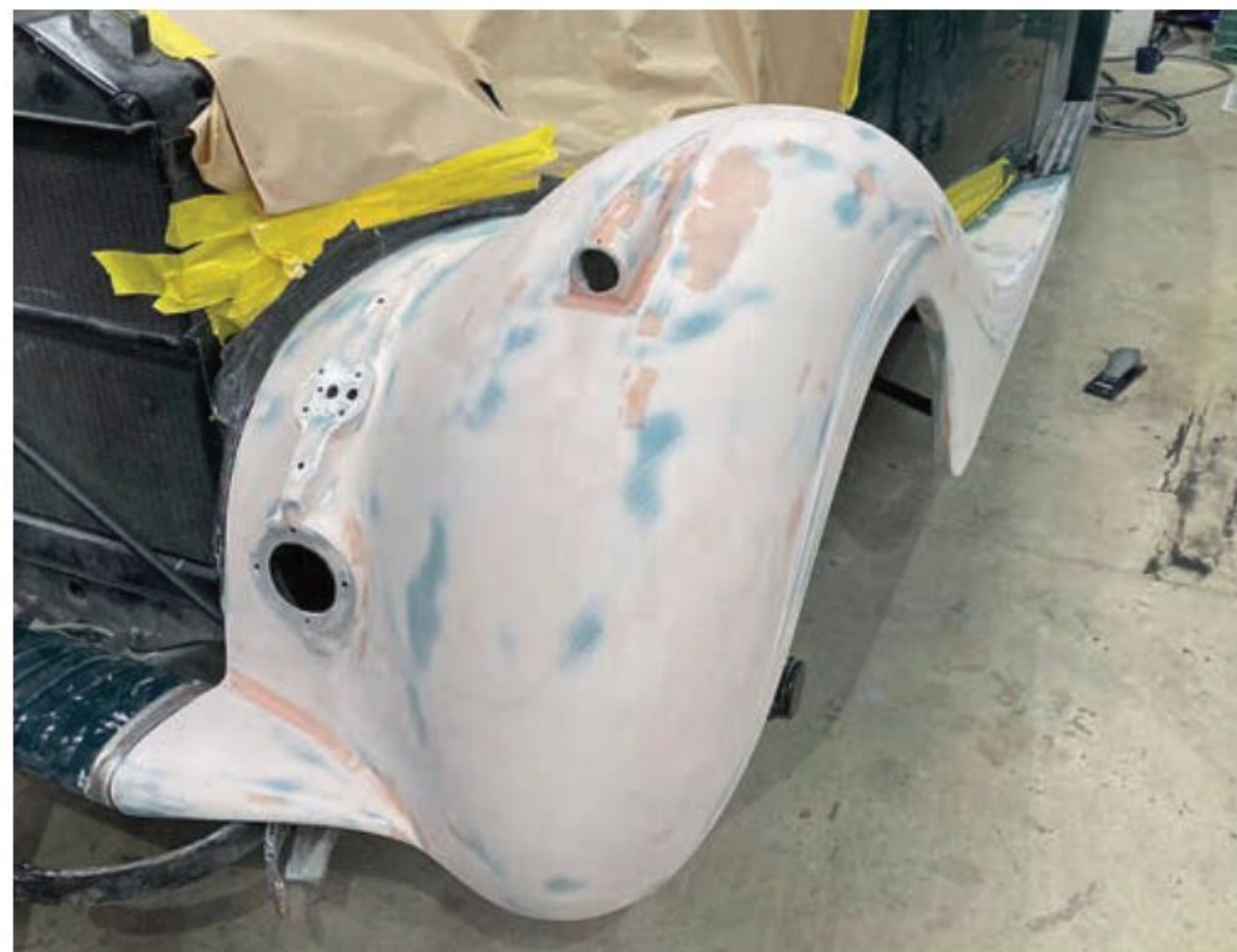
Repeated processes of filling, priming and flattening were involved in the finishing touches
