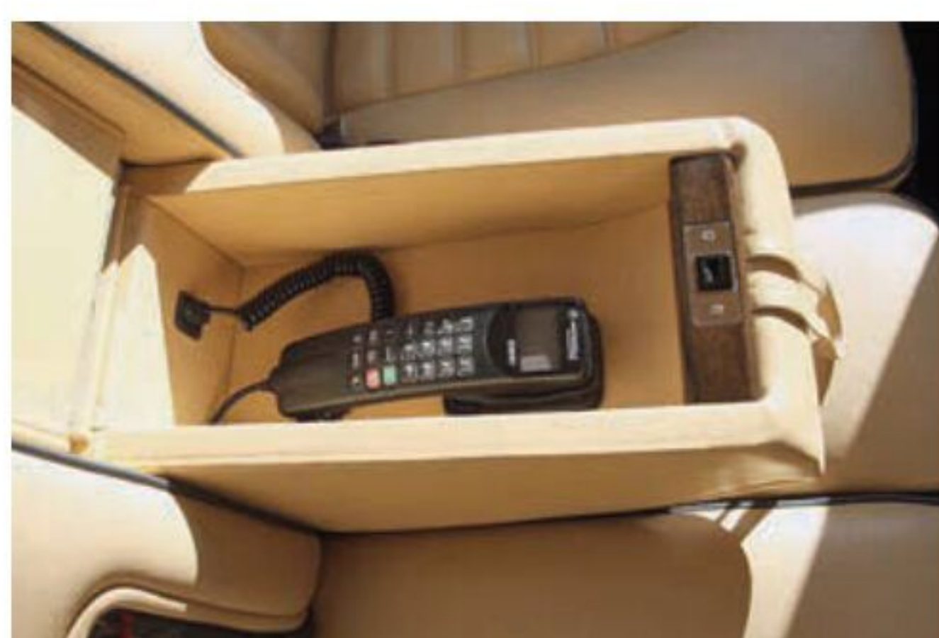
An additional plug-in Motorola GSM 2500 handset is fitted inside the rear armrest
