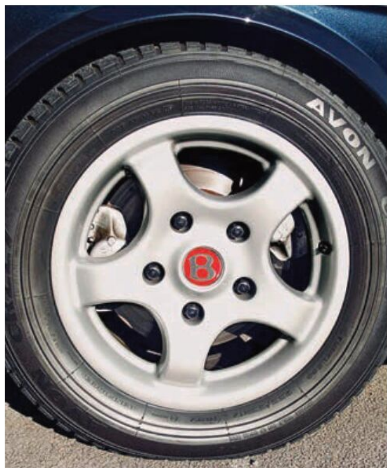
The Turbo RT features five-spoke 17-inch alloys and Continental T twin-caliper ventilated front discs
