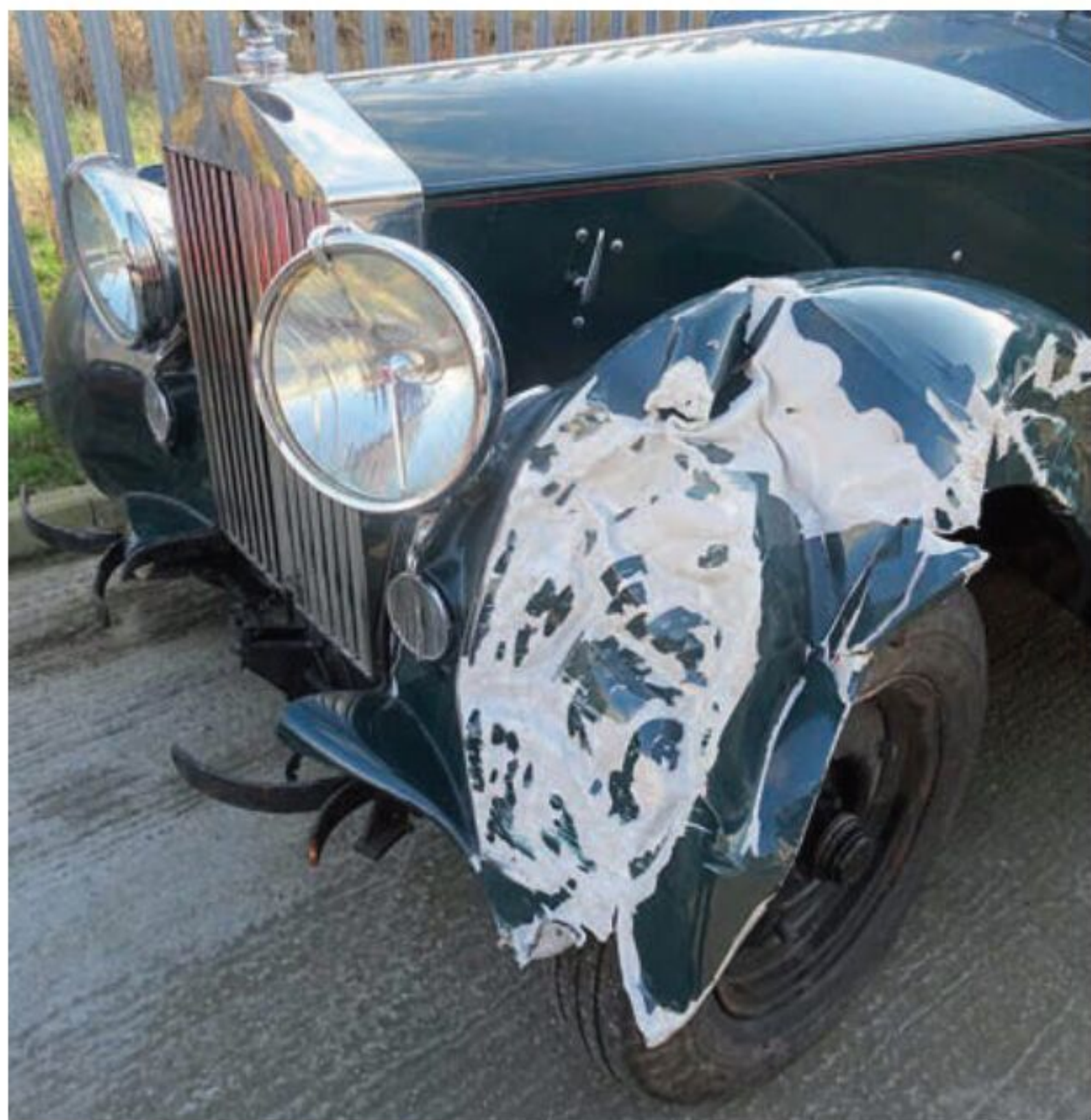
The Silver Wraith arrived at The Beaconsfield Workshop with extensive wing damage
