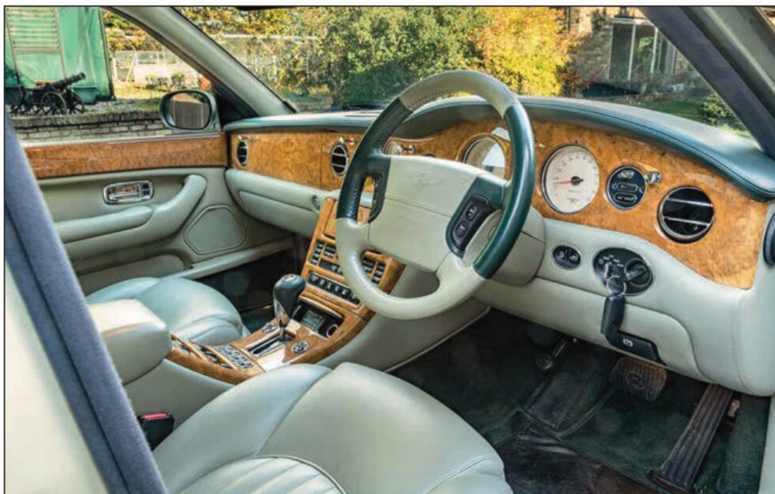
While the Seraph and Arnage were similar inside, the Bentley had a centre gear selector and more comprehensive instrumentation
