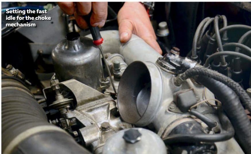
Moving on to balance idle settings on both carbs
