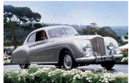
OLG 490 was the first R-type Continental; note the split-windscreen that was a feature of the prototype but not carried through to the production cars.
