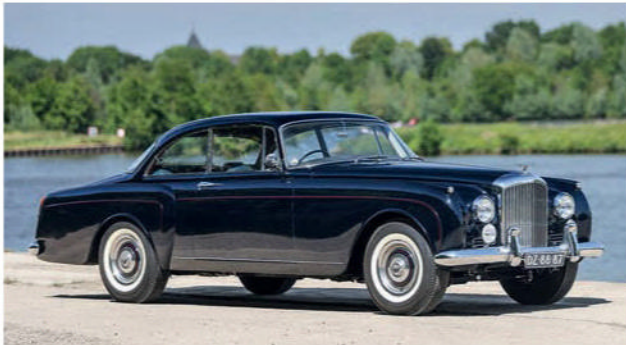
For the S2, H J Mulliner updated its Continental body, incorporating a notchback tail with wraparound rear window.
