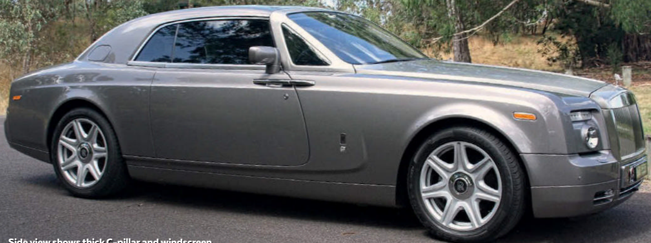
Side view shows thick C-pillar and windscreen support shared with Convertible
