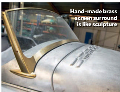
Shown here before plating and painting, the new body has impressive presence
