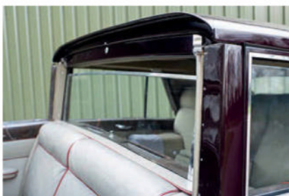
Division is electrically raised and lowered
