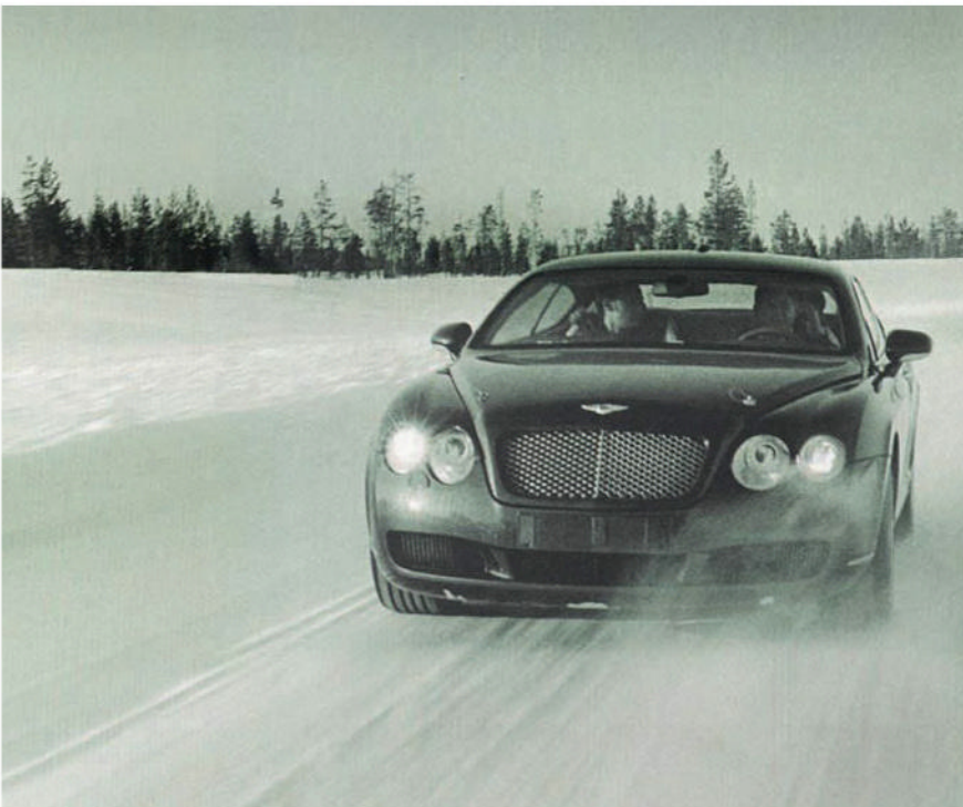
Cold weather testing – assessing the car for snow packing performance. Note the VW Transporter pulling the sledge to stir up snow in front of the car
