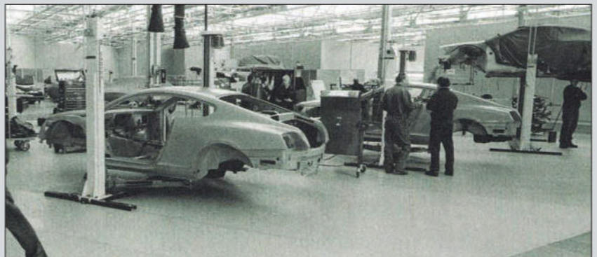
Inside the Bentley Engineering Workshop, showing prototype Continental GT bodies waiting to start assembly
