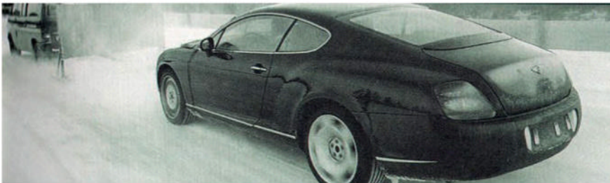
Cold weather testing – assessing the car for snow packing performance. Note the VW Transporter pulling the sledge to stir up snow in front of the car
