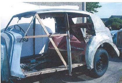
The bodyshell was braced to ensure there were no problems with distortion
