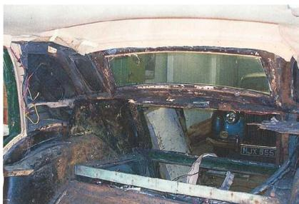
The rear window frame was totally rotten, which meant making an exact replica
