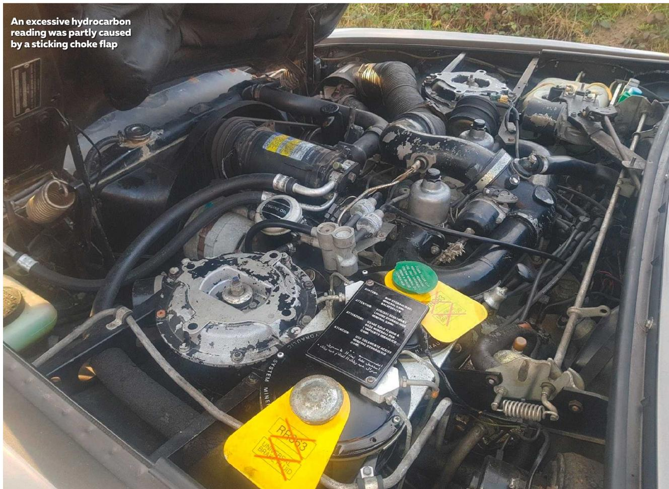
An excessive hydrocarbon reading was partly caused by a sticking choke flap
