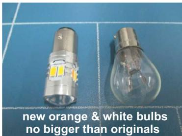
The bulbs in semaphore arms can be upgraded to bright orange flashing ones, to make them useful instead of decorative. At the rear of early cars, the tail and brake lights are often very dim and again, the lack of orange flashing indicators can be a safety issue. Better Car Lighting can help here too. Most of the usual suspects
