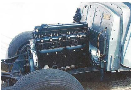
The engine received new piston rings, re-ground valves and other essential work
