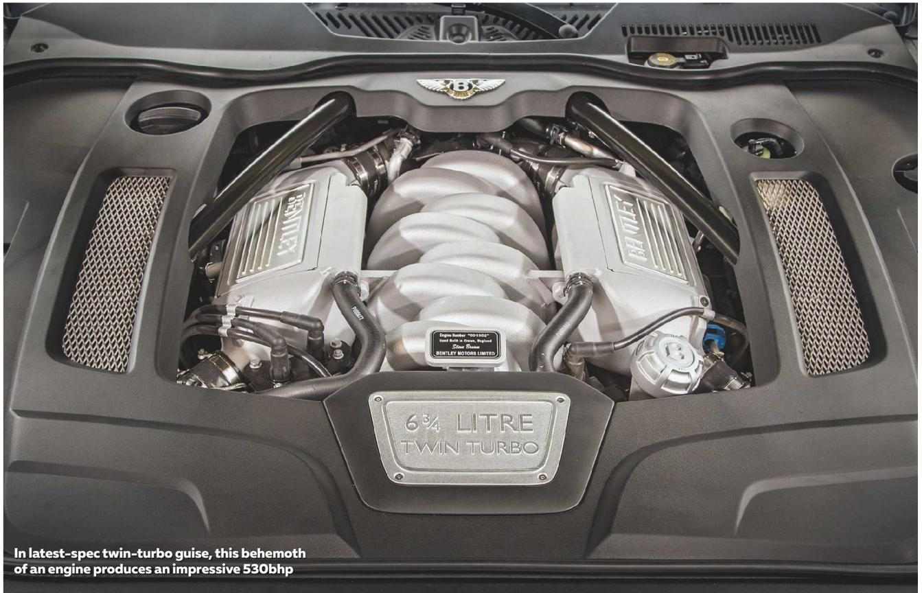
In latest-spec twin-turbo guise, this behemoth of an engine produces an impressive 530bhp
