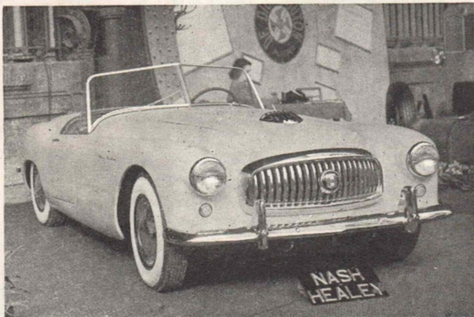
Britain's newest: The six-cylinder, 115 b.h.p., 3.8-litre, Nash-engined Healey is reputed to be the fastest car to be produced by the Warwick concern. Chassis specification is similar to the Silverstone model.
