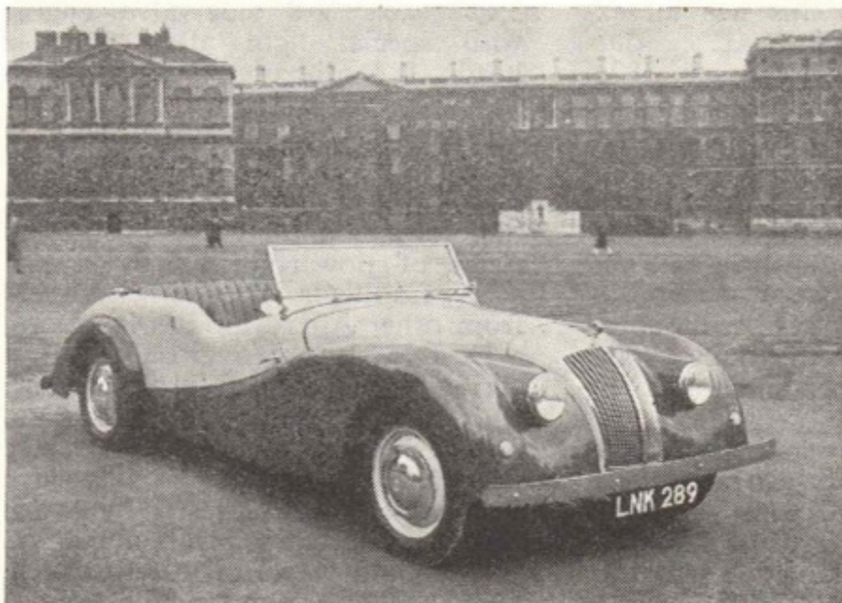
SPORTS - TOURER: The six-cylinder, 2-litre A.C. is one of the few remaining cars with non-independent front suspension. It is seen here as an open 5-seater.
