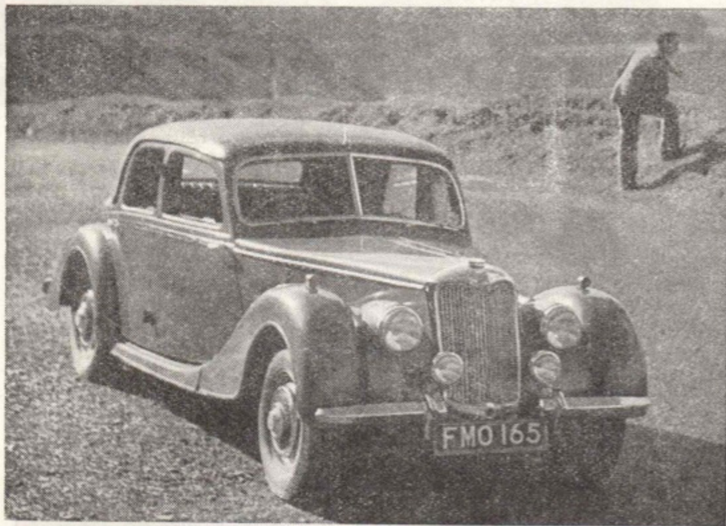
RILEY: The successful 2½-litre Riley sports saloon continues practically unchanged for 1951. It is a genuine 90 m.p.h. machine, and has torsion-bar i.f.s.
