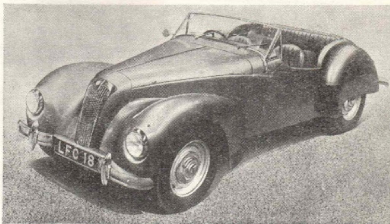
LEA-FRANCIS: The open sports "2½-litre" has a twin-camshaft, push-rod engine developing 100 b.h.p. It is capable of over 90 m.p.h.
