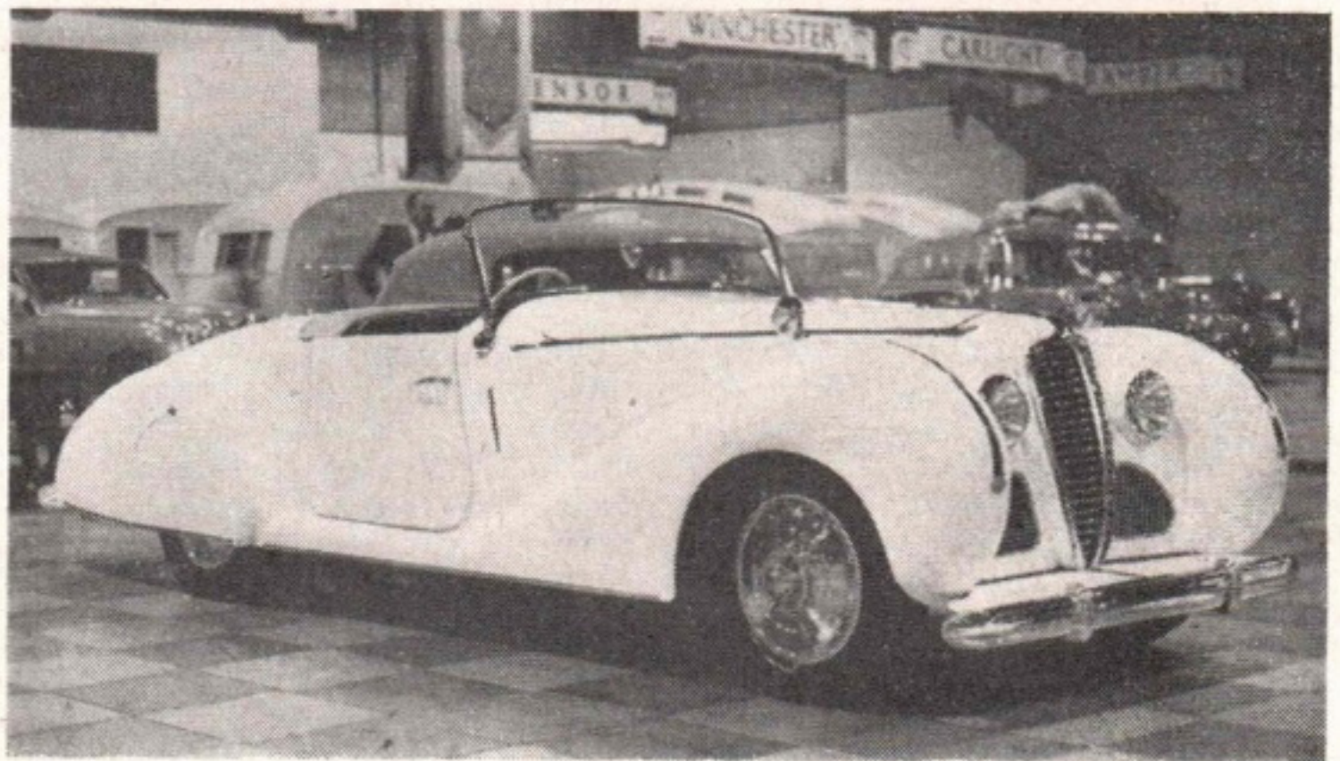
A smart two-seater Delahaye on the Type 135 M chassis. This has an o.h.v. six-cylinder engine, transverse leaf i.f.s., and Cotal-electric gearbox.
