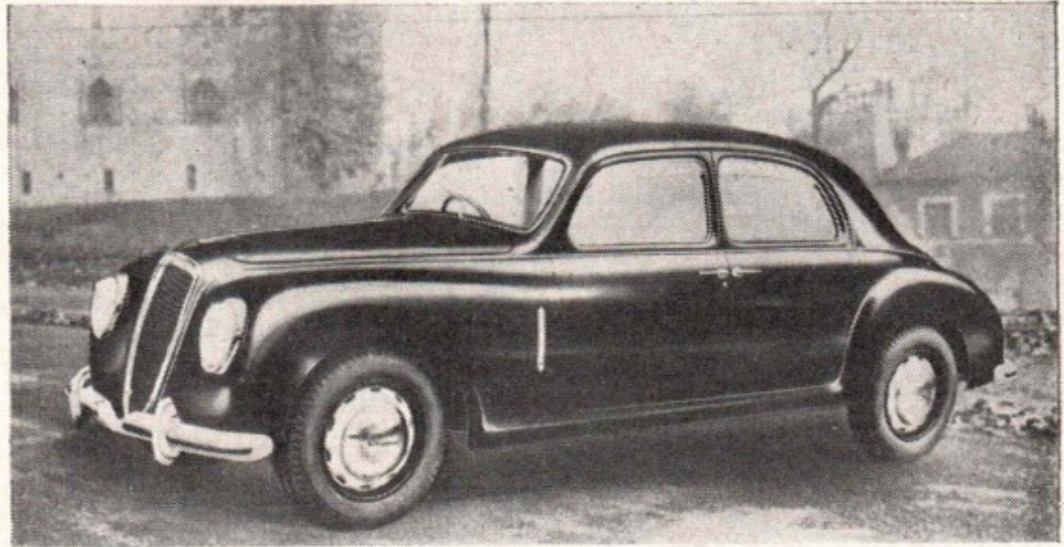
The Lancia Aurelia is unorthodox in the use of a V-6 engine, gearbox and clutch combined with final drive, and inboard rear brake drums.
