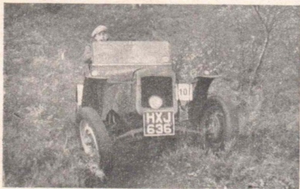
R. A. Hopkinson's Bancroft Special (above) openly reveals its transverse cart-spring front suspension while wrestling with Tank Trap in the Crewe and S. Cheshire M.C.'s Clifford Cup Trial, held on 5th November.
