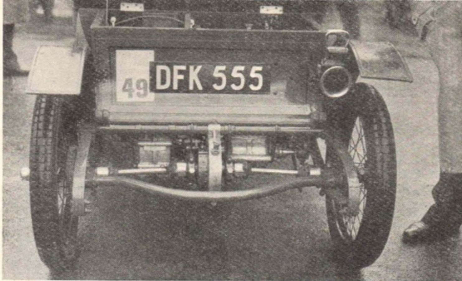
Modern fitment (1): De Dion rear axle as seen on several cars of that famous make. This is Dudley John's 1901 model.
