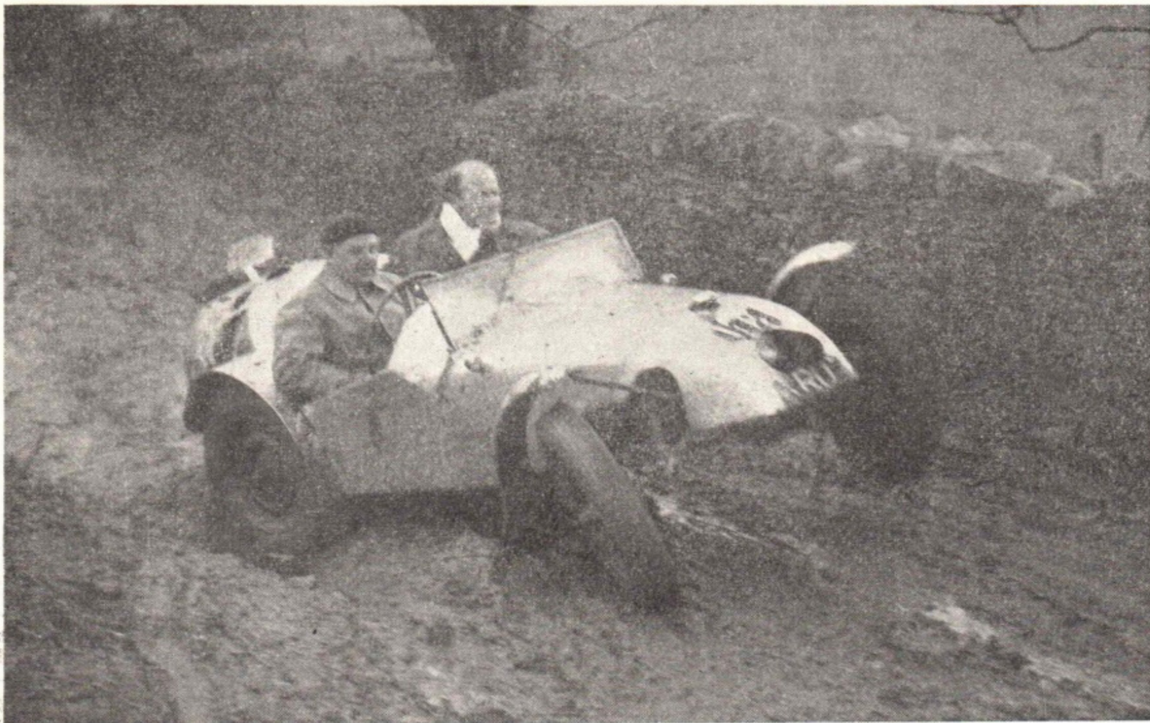
AIRBORNE: This Green Lanes shot of Leslie Onslow-Bartlett's Bartlett-J.A.P. proves fairly conclusively that controllability has been sacrificed to an excessive rear-to-front weight distribution ratio.
