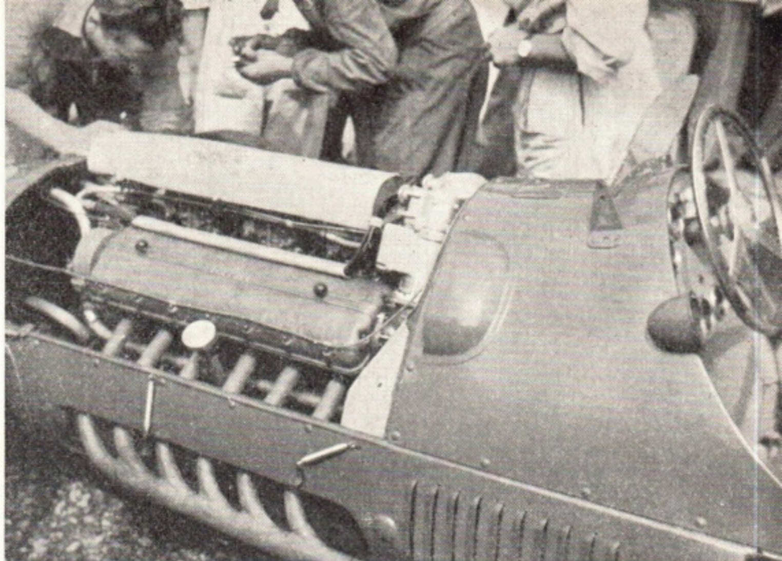
UNBLOWN: A close-up of the much-discussed 4½-litre, unsupercharged V-12 Ferrari engine. The three carburetors are fitted with a special air-scoop, and twin magnetos are driven from the rear of the overhead camshafts.
