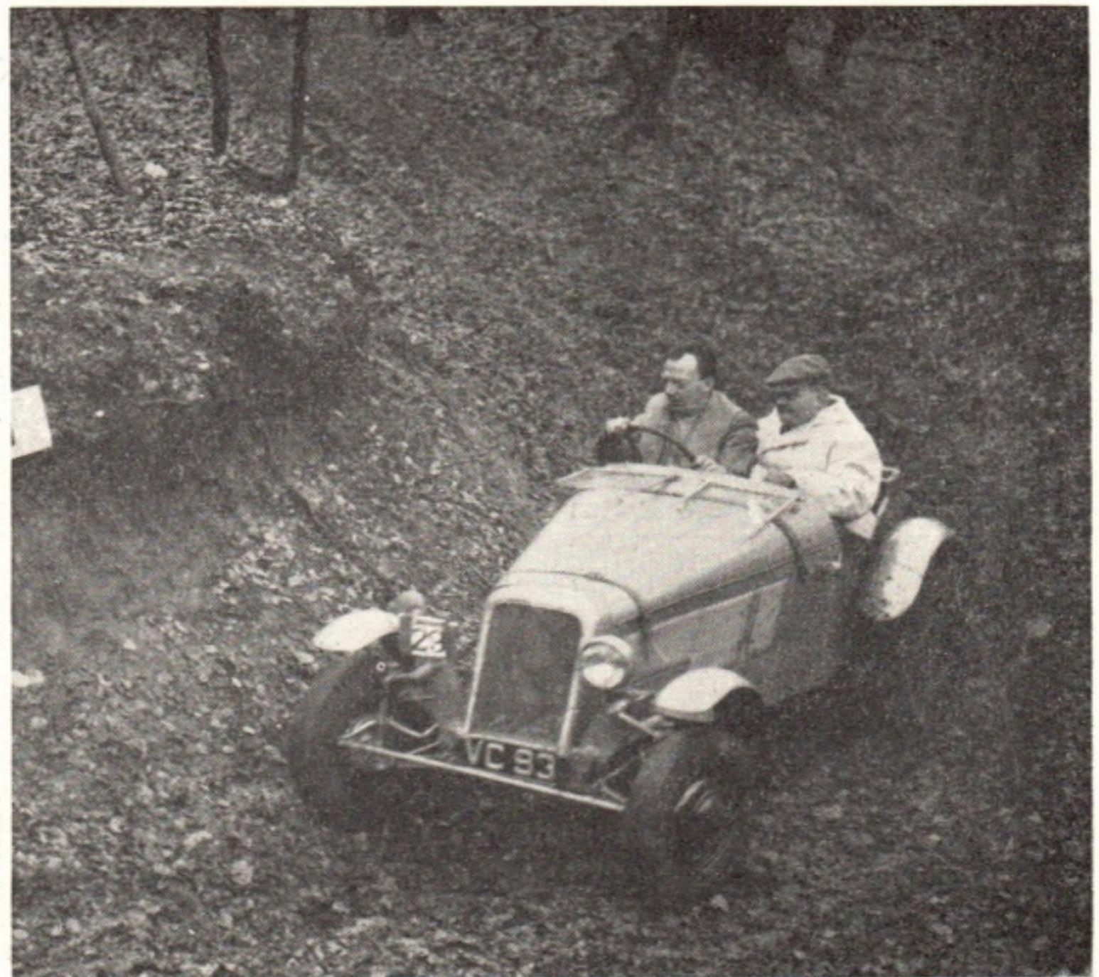
H. F. Brayshaw's interesting torsion-bar i.f.s. lightweight special about to come to rest on Breakheart.
