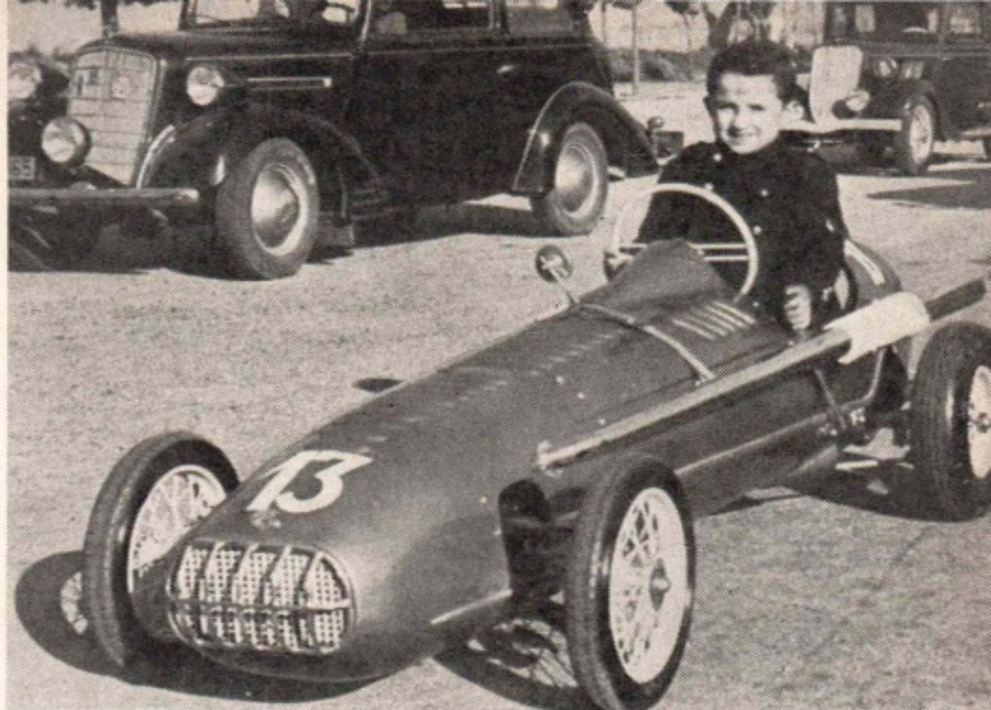
SPANISH SPECIAL: Angel Gabrera Marzal of Barcelona, built this delightful racing-car for his son. It is 30 ins. high, 7 ft. long, does 80 m.p.g., has a 3-speed and reverse gearbox, and does over 35 m.p.h. It cost about £100, taking 720 man-hours to build.
