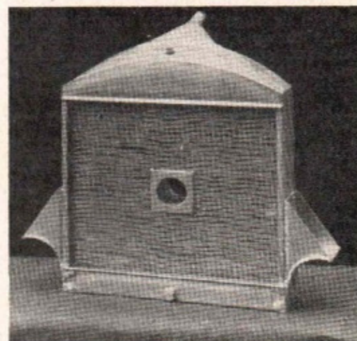
A combined oil radiator and cooler constructed for the Connaught Engineering Co. Ltd., by Gallay Ltd. The unit is designed to bring the oil temperature down to approximately that of the water temperature.
