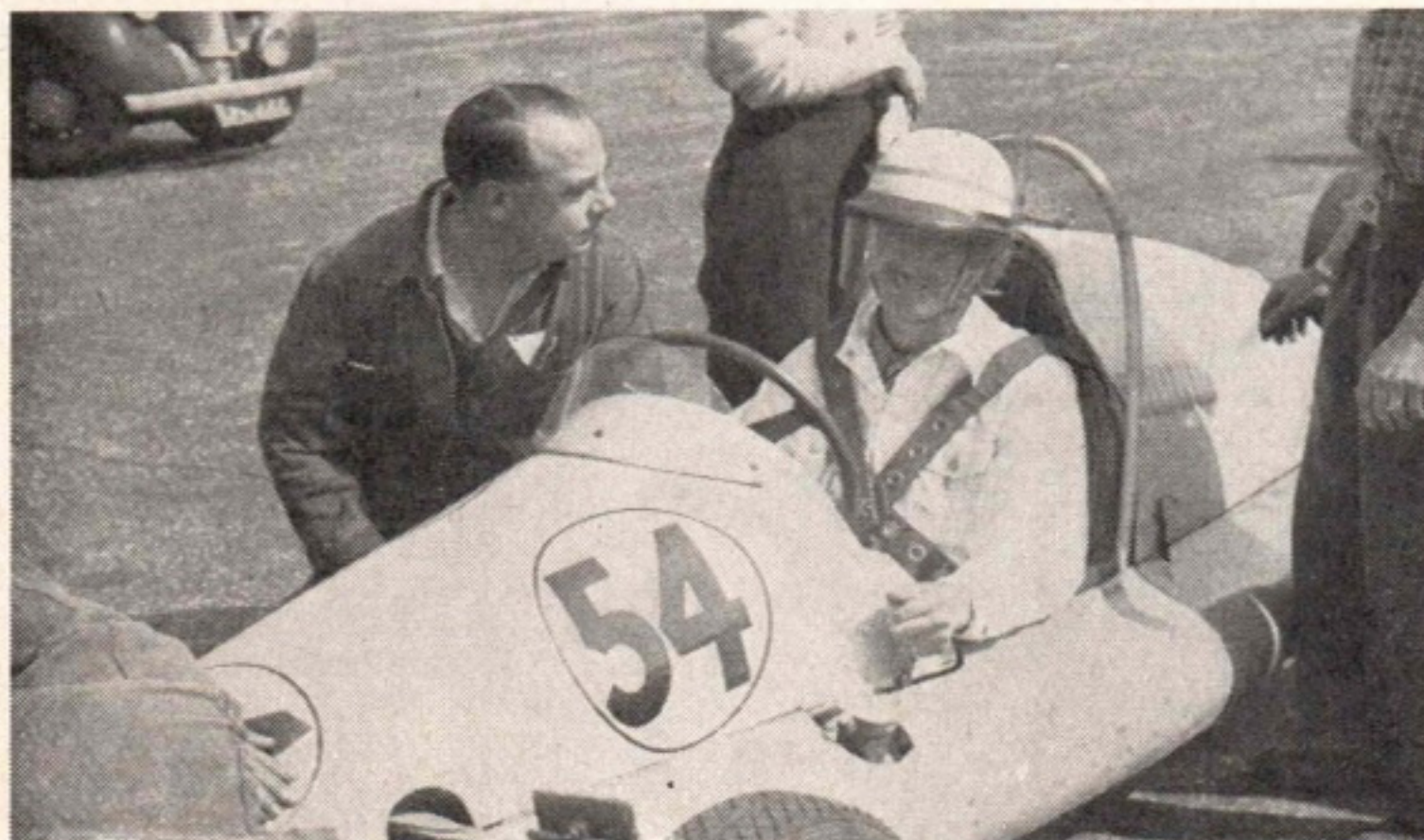
SAFEGUARD: More and more Formula 3 cars are appearing with anti-crash bars. Here is "Pop" Lewis-Evans and his Cooper, which is so fitted.
